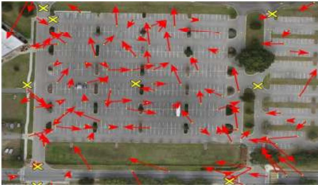
**Figure 22: Sample of GPS error when compared to ground control points exaggerated by 1000 times**
