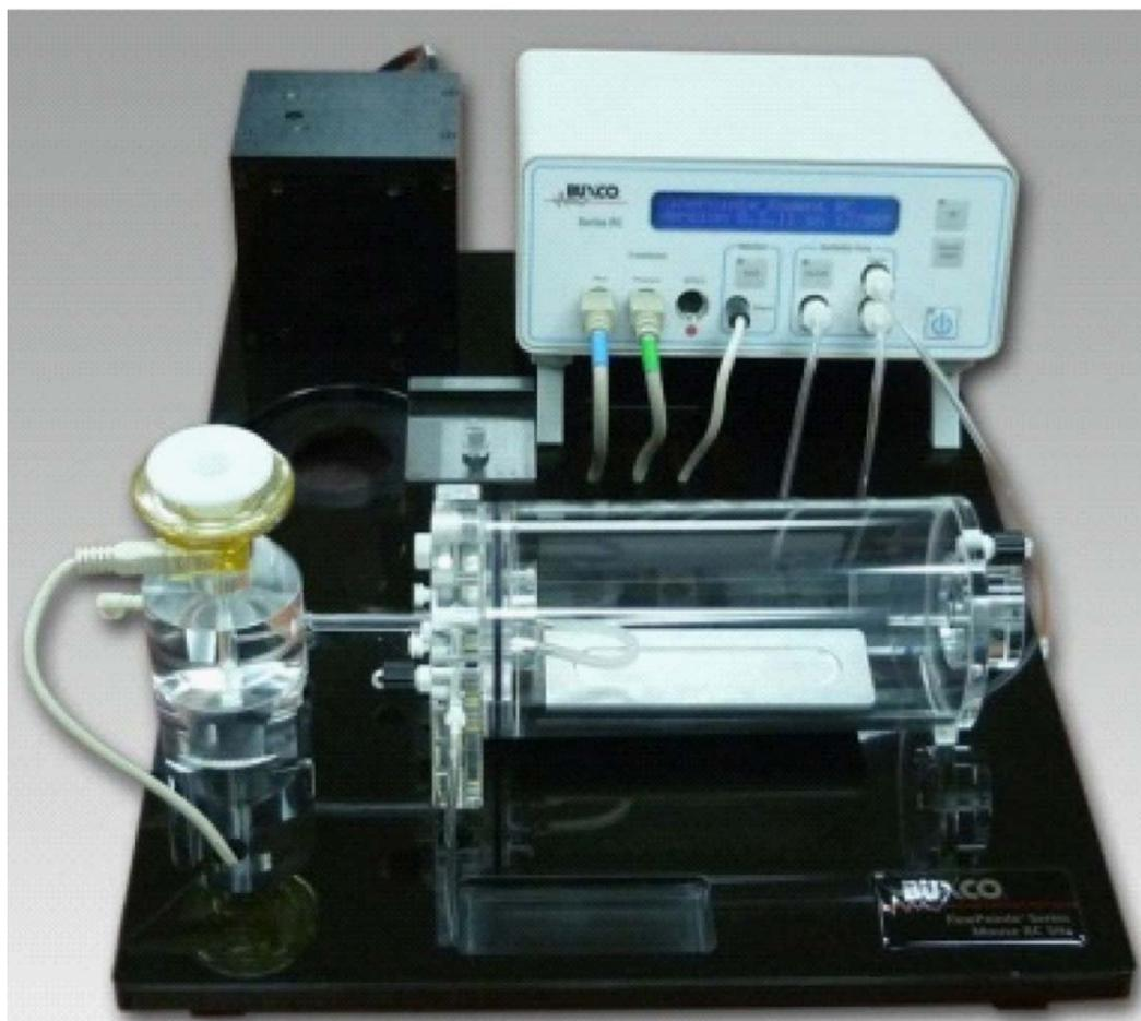
**Fig. 2-1 R&C (resistance and compliance) system (Buxco, USA)**
