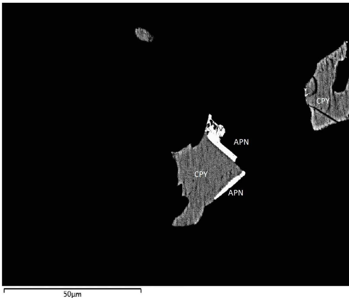
Figure 23: A backscatter electron image taken during the SEM-EDS study that shows euhehedral argentopentlandite and associated chalcopyrite grains. APN: argentopentlandite; CPY: chalcopyrite.
