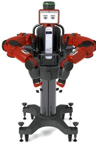
Figure 1.4: Baxter, the world first low-cost industrial humanoid robot
