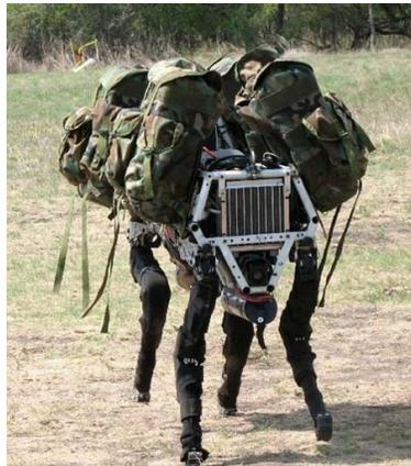
Figure 1.3: BigDog quadruped robot
