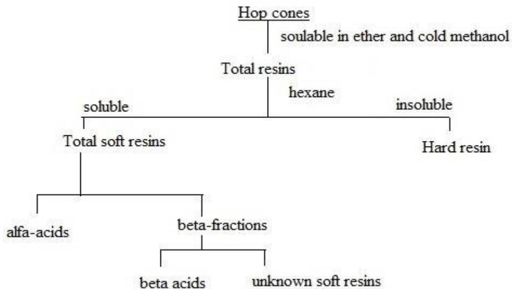
**Figure 2.** Hop extraction and fractionation (modified from [10])
