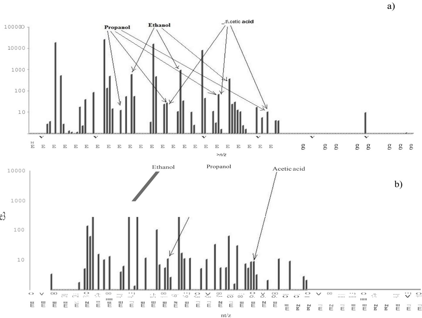
**Figure 10.** Headspace gas SIFT-MS spectra analysis of wort inoculated with *L. brevis* measured on day 7. Graph a) represents spectra using  $H_3O^+$  precursor ions and b) represents spectra using  $NO^+$  precursor ions. Ions produced from blank (wort) sample were subtracted from this data. Product  $m/z$  values for major peaks are indicated on the graph.
