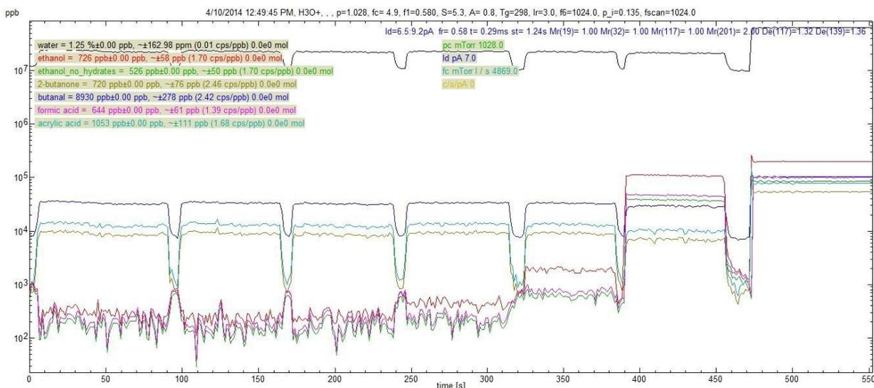
**Figure 6.** Example of MIM mode for detection of ethanol using  $\text{H}_3\text{O}^+$  precursor ion. The plateaus represent calculated average concentrations (in ppb) of various (colour coded in the software) product ions.
