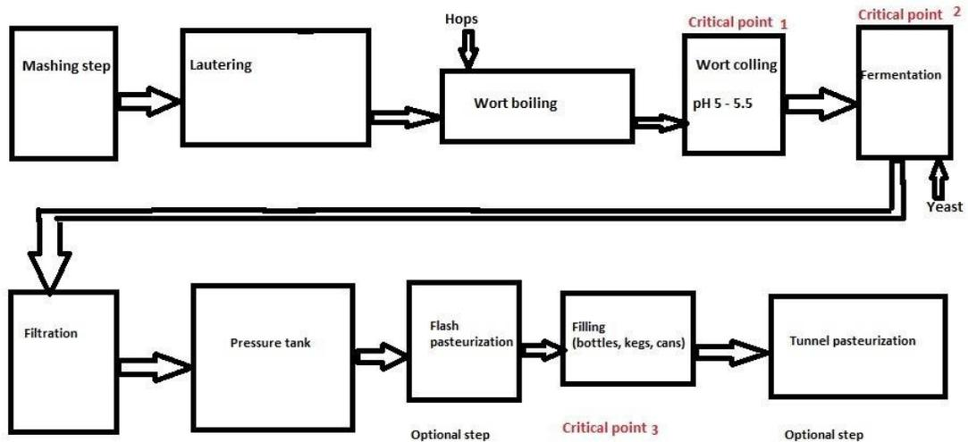
**Figure 1.** Production line of beer with critical control points
