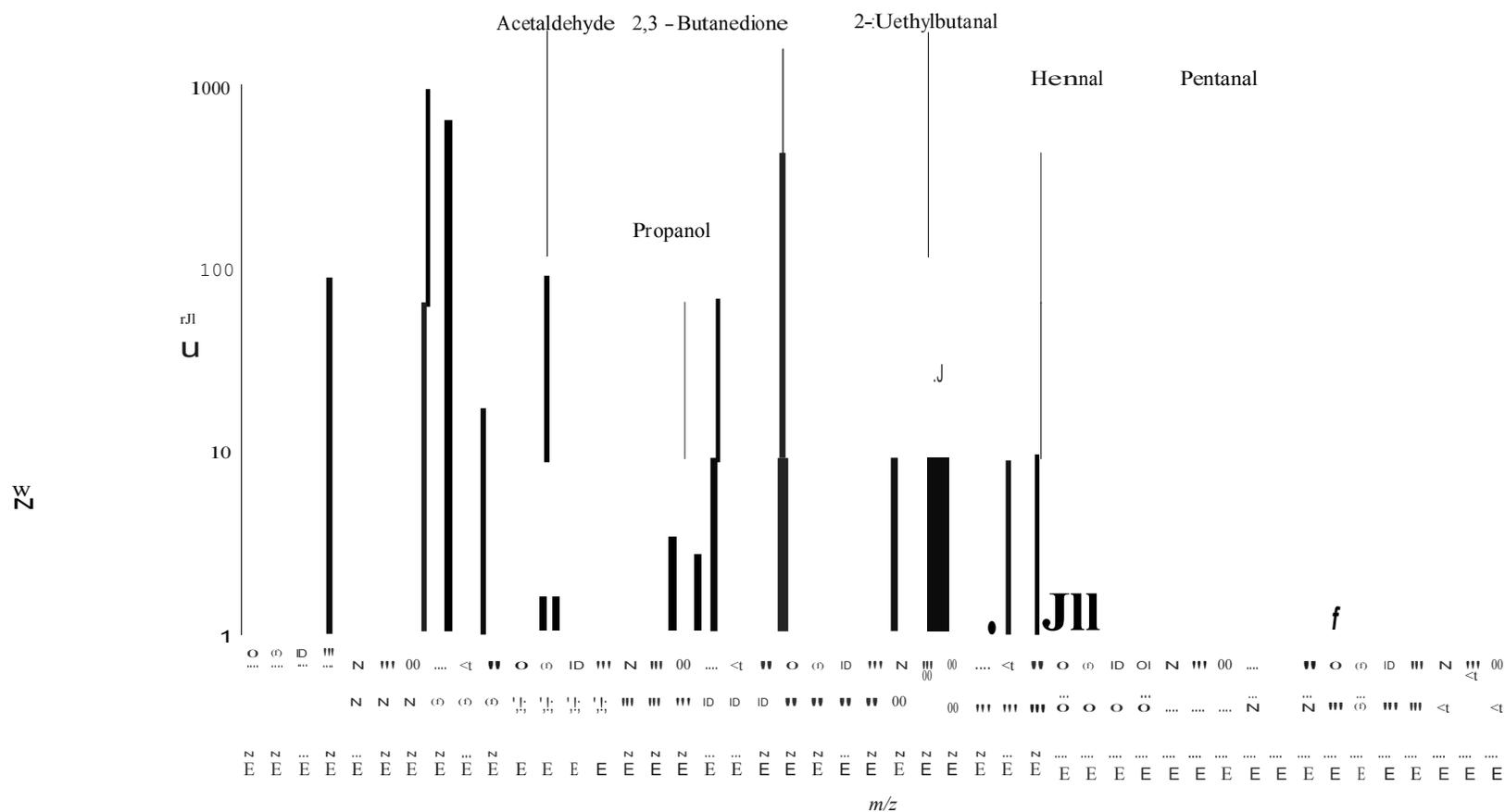
**Figure 8.** Headspace gas SIFT-MS spectra analysis of wort using NO<sup>+</sup> precursor ions. The mean of 3 samples is shown. Ions produced from blank (water) sample were subtracted from this data. Product m/z values for common compounds in wort as conformation of the compounds acetaldehyde, 2,3 – butanedione, hexanal and 2-methylbutanal are indicated on the graph.
