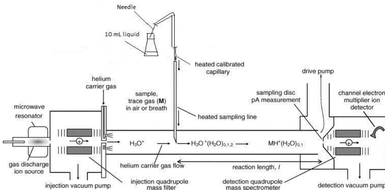
**Figure 4.** SIFT-MS diagram with indicated precursors, carrier gases and way of operation (From references [48, 49]).
