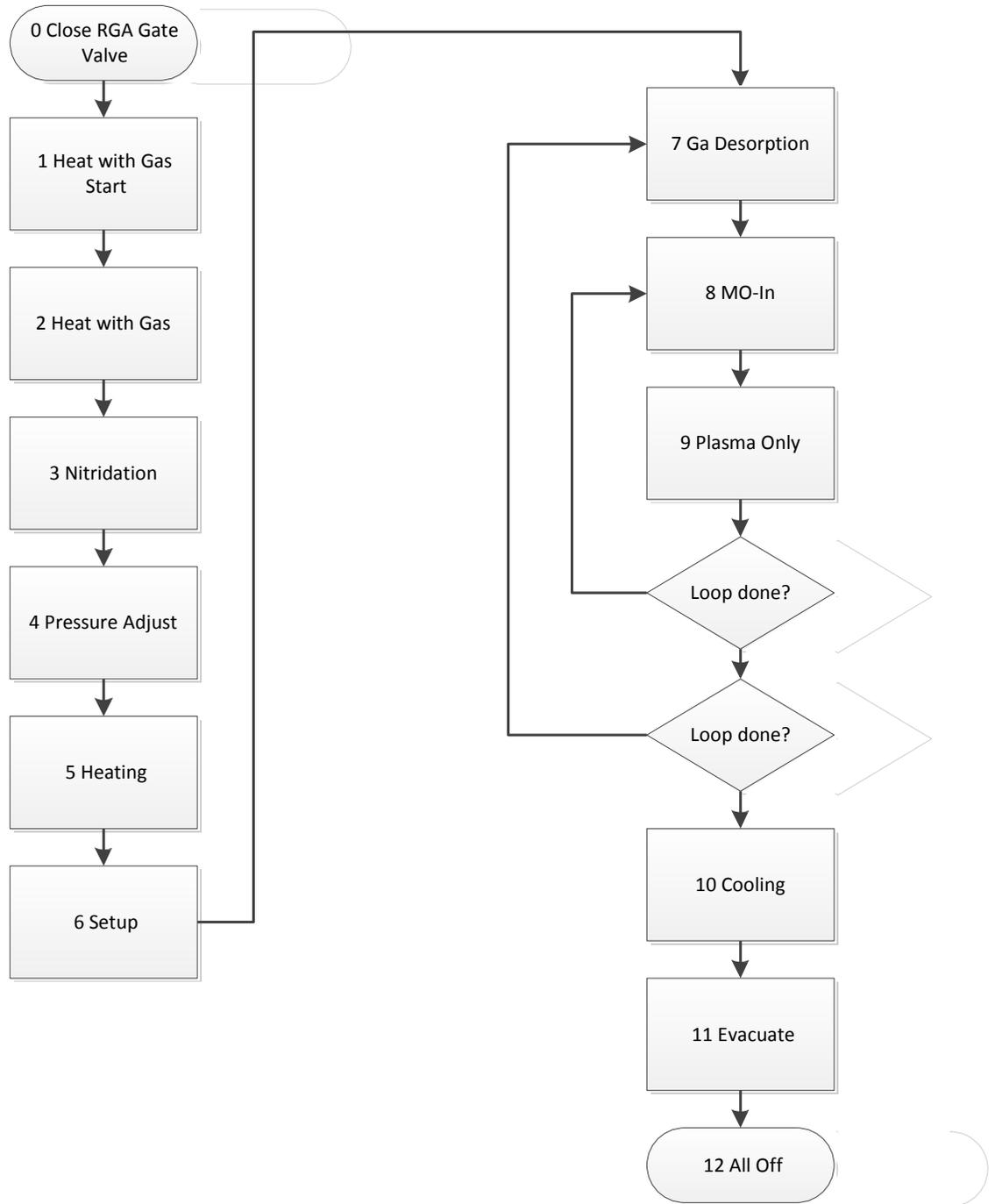
**Figure 17. Modified GaN film growth flow chart showing desorption step.**
