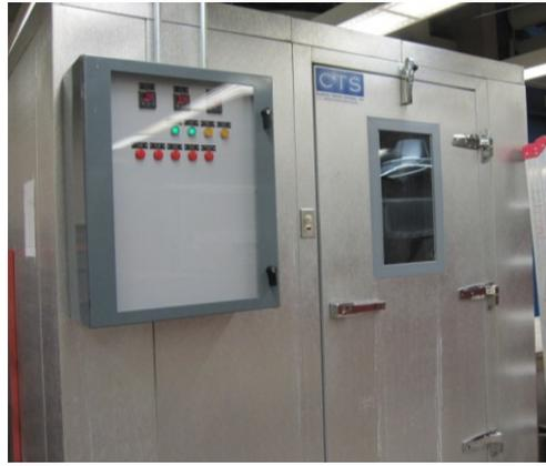
**Figure 3.1: Walk-in freezer used to freeze sludge samples**
