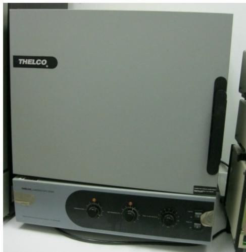
**Figure 3.2: Precision Thelco laboratory oven**
