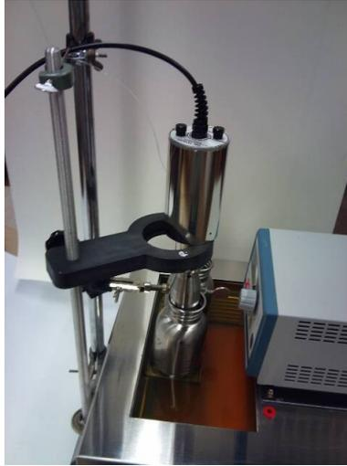
**Figure 5.1: Set-up of probe and freezing bath for progressive ultrasonic freezing experiments.**
