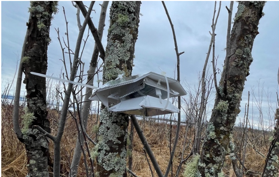
Figure 2.4. Setup to record air temperature at study ponds. The silver and white plastic rectangle is a radiation shield for the thermal logger (HOBO MX2201).
