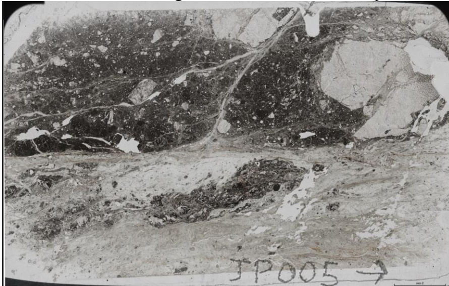
JP005 PPL – Tonalite and gabbro-norite fault core with slip surface
