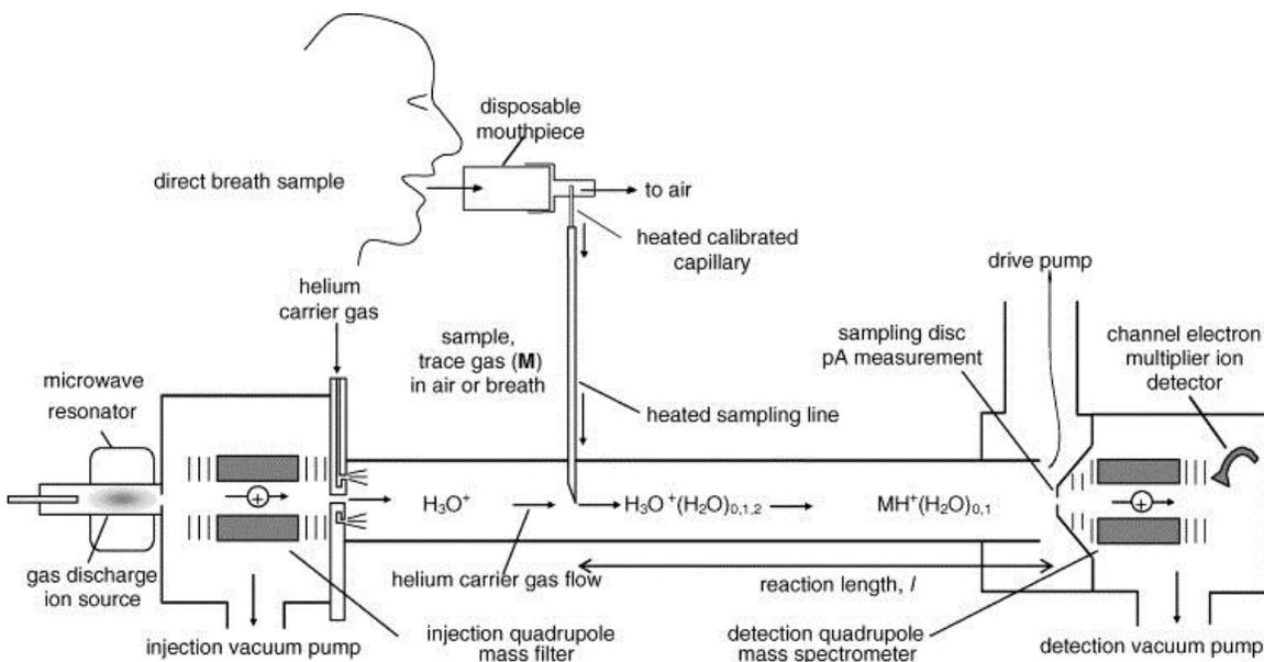
**Figure 5:** Schematic diagram of a SIFT-MS machine showing sample microwave resonator ion source, which produces precursor ions that react with samples introduced downstream either through breath or headspace analysis. Ions react and are carried along the flow tube by helium gas, and finally sampled by the downstream quadrupole mass spectrometer (Spanel *et al.* 2005).
