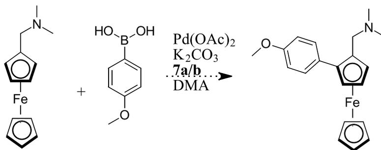
**Scheme 15.** Initial, unsuccessful attempt at a cross-coupling reaction between 4-methoxyphenylboronic acid and N,N-dimethylaminomethylferrocene in the microwave reactor using CILs.
