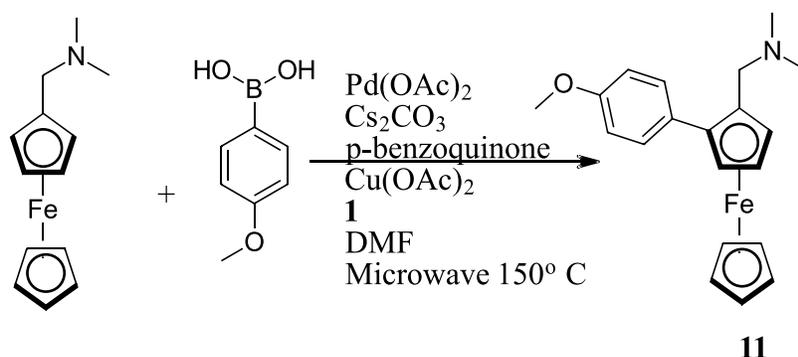
**Scheme 17.** Initial successful reaction conditions of a cross-coupling reaction between N,N-dimethylaminomethylferrocene and an aryl boronic acid.
