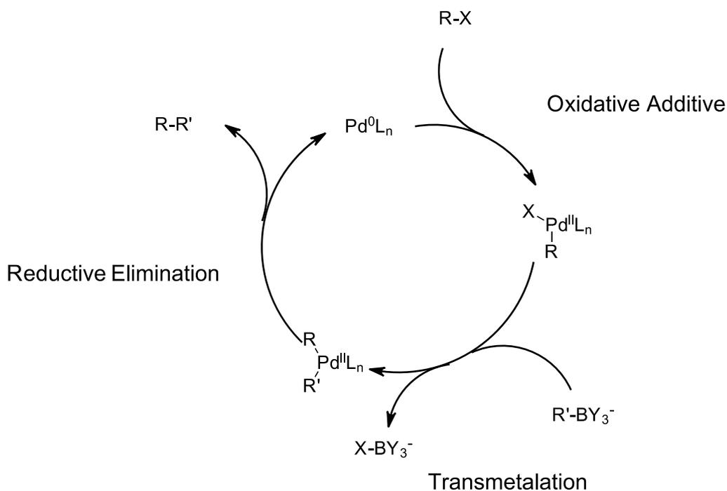
**Scheme 1.** A generic Suzuki cross-coupling catalytic cycle, comprising three steps: oxidative addition, transmetalation and reductive elimination.
