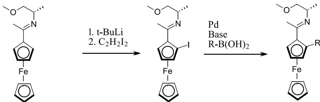
**Scheme 3.** The typical method for synthesis of planar chiral disubstituted ferrocenes<sup>33</sup>. An enantioselective lithiation is followed by lithium halogen exchange and finally a cross-coupling reaction.
