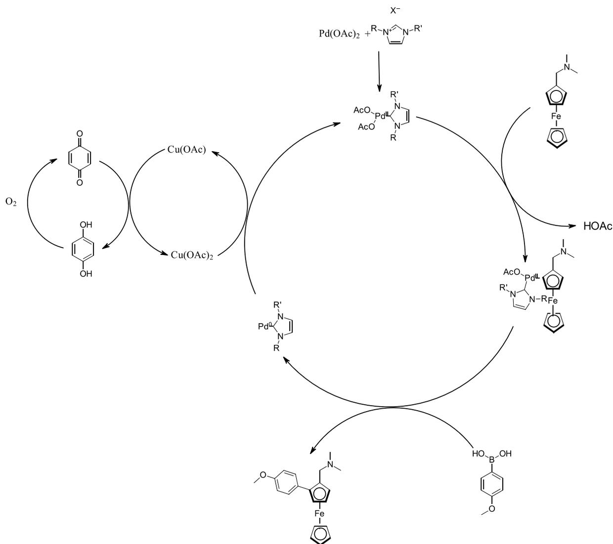
**Scheme 16.** Proposed catalytic cycle for the reaction between N,N-dimethylaminomethylferrocene and 4-bromoanisole.
