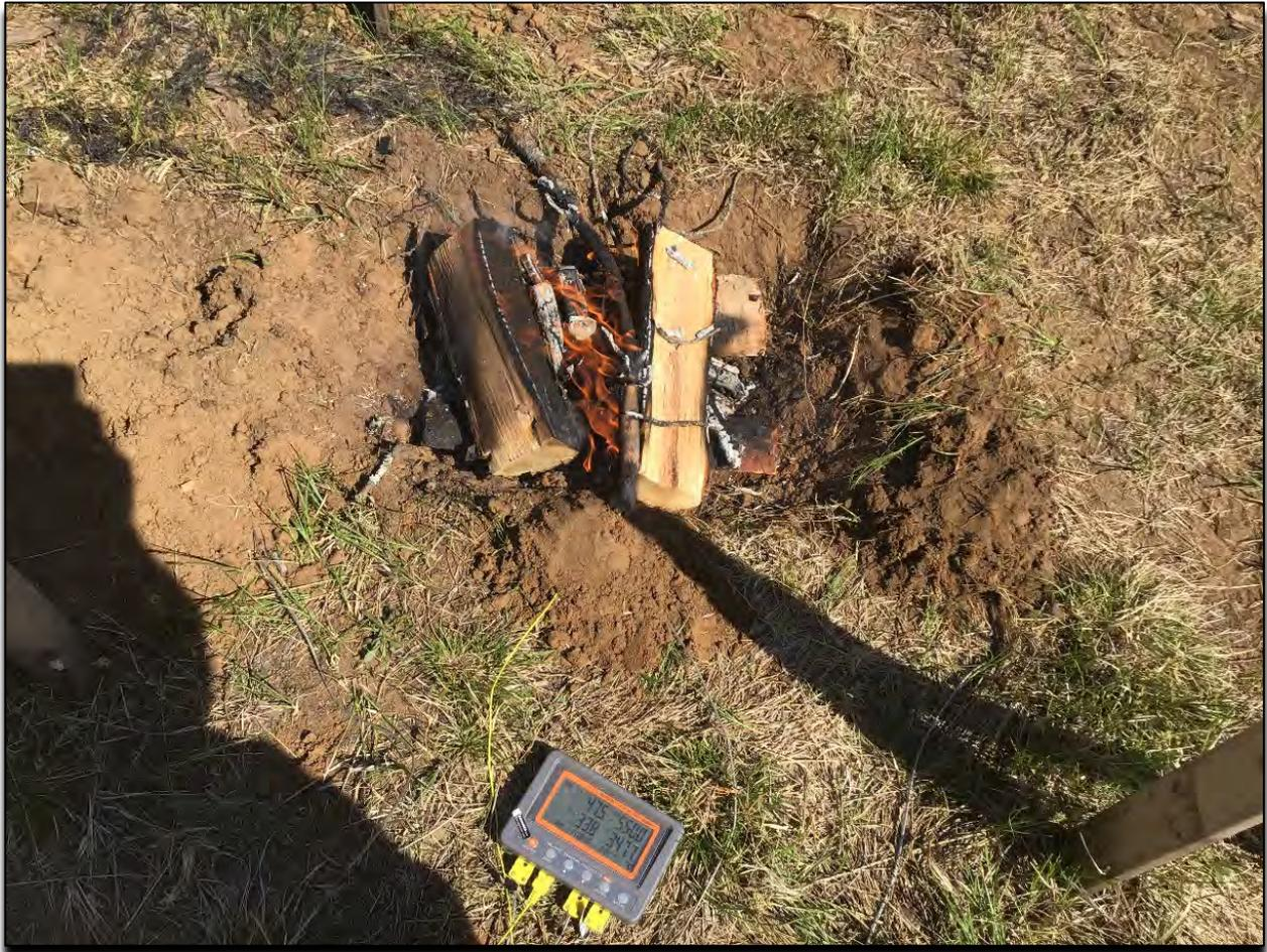
*Figure 4.8 Thermocouple probes and thermometer in use during a long-term firing experiment.*
