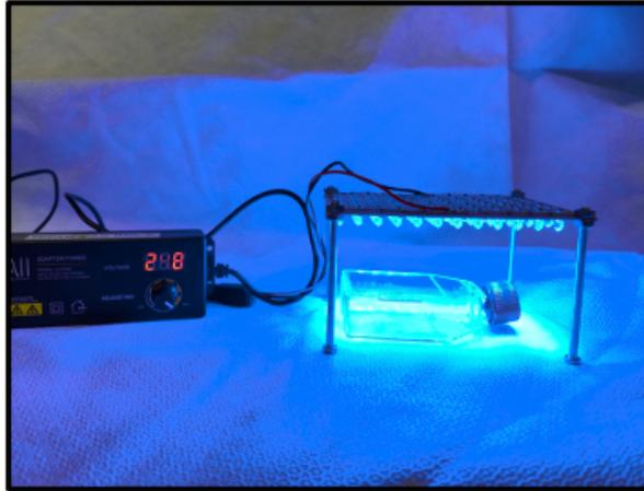
**Figure 3.1 – Blue Light Panel Exposing a T-25 Flask** The blue light manifold supported on top of a T-25 flask to show how it is used in the tissue culture incubator. The LED panel is connected to a power supply and mechanical timer. These work together to ensure that the LED panel receives the required voltage of power for the proper duration of time.
