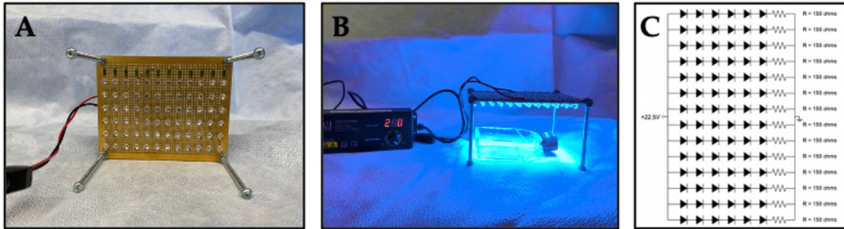
**Figure 2.9 - Blue Light Apparatus.**
