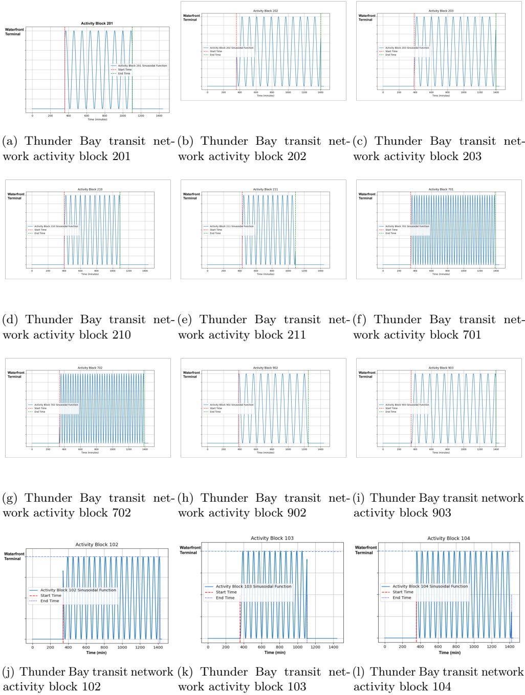
FIGURE 6: City of Thunder Bay transit system piece-wise sinusoidal-modelled activity blocks charging at Waterfront terminal
