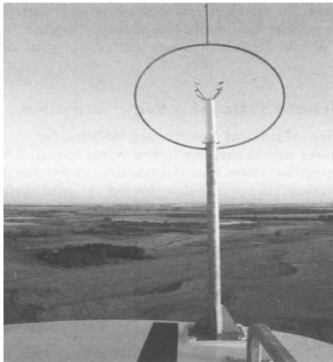
Fig. 2-6. Ultrasonic anemometer wind speed sensor [8]
