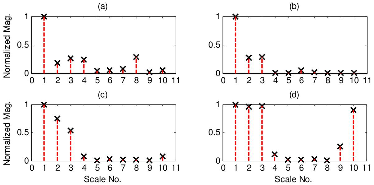
**Figure 3.4.** Demonstration of normalized DP indicator values versus IMF scale numbers corresponding to different bearing health conditions: (a) healthy bearing; (b) bearing with outer race defect; (c) bearing with inner race defect; (d) bearing with rolling element defect.
