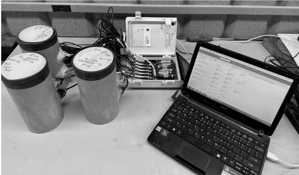
Figure 3.5. Mould Base Monitoring Program (A) a 5TE sensor measuring moisture, temperature, and electrical conductivity, (B) a TEROS 21 sensor measuring water potential and temperature, (C) a data logger identified as ZL6, (D) the process of data collection, and (E) the test samples.
