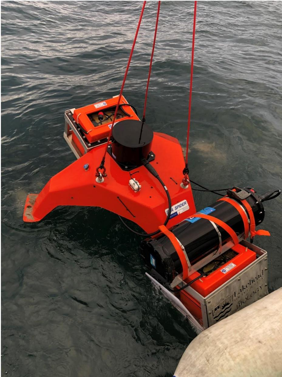
Figure 1.1. Picture of the acoustic platform deployment with a two-battery arrangement.
