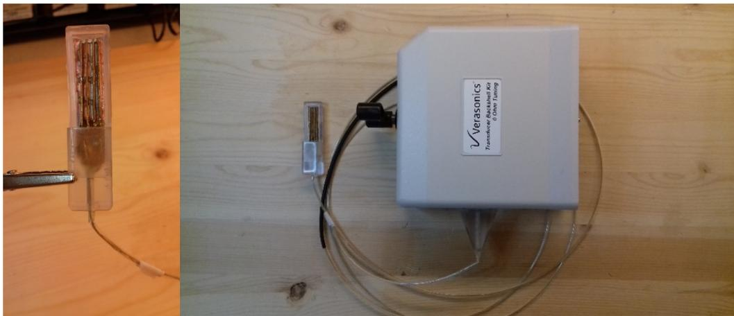
*Fig. 6. 1. Four-Elements ultrasound imaging biaxial probe.*
