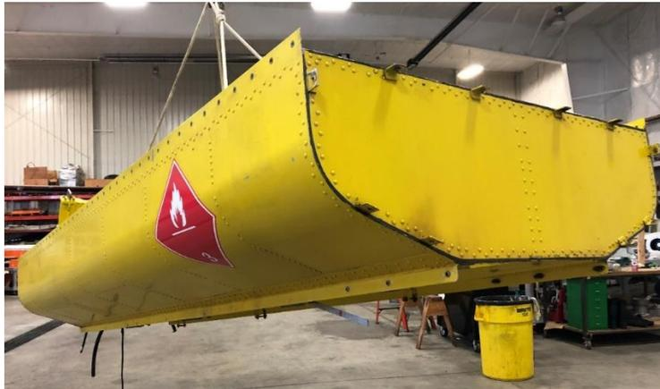
Figure 2.5:AT-802 FuelBoss belly tank
