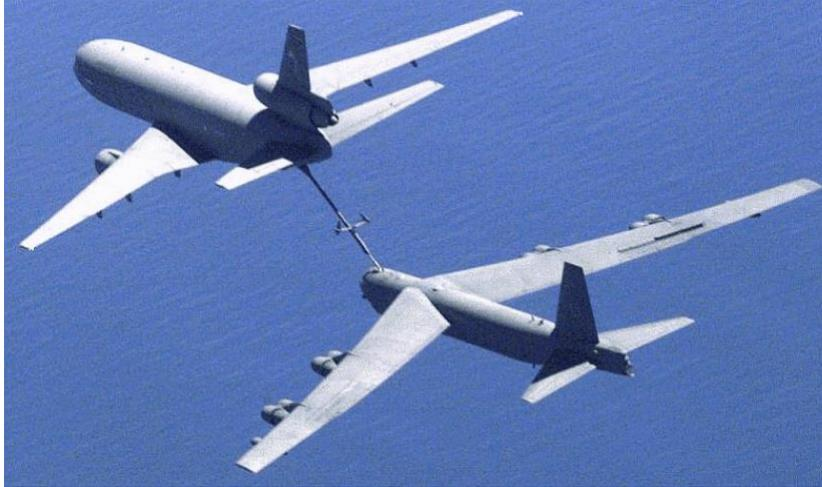
Figure 1.3: KC-10 refueling a B-52 using the 'flying boom' method [8]
