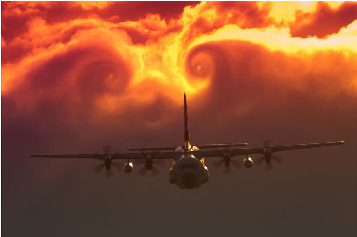
Figure 1.5: U.S. Coast Guard photo of C-130J with wake turbulence visible in clouds [12]
