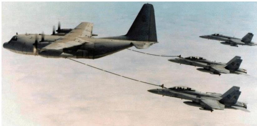
Figure 1.4: KC-130 refueling multiple F-18s using the probe and drogue method [5]
