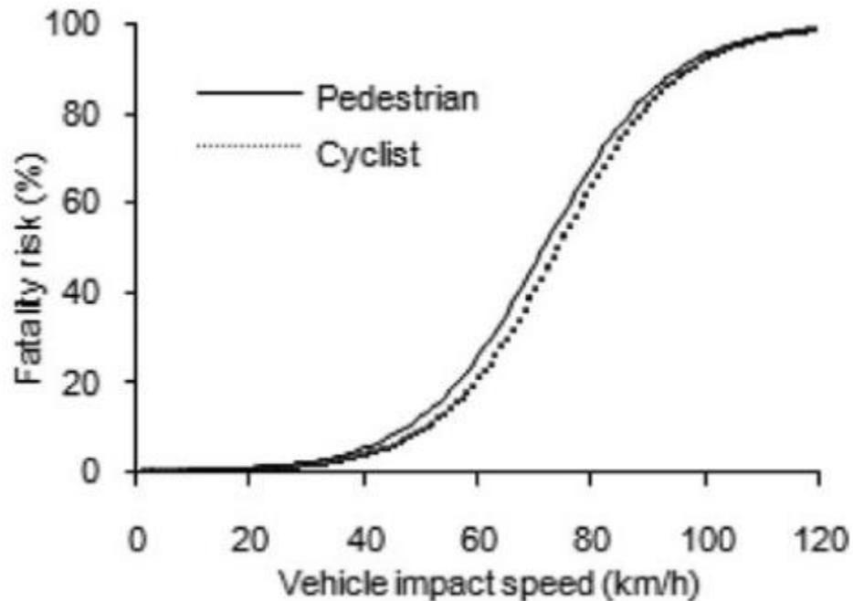
**Figure 10: Relationships between Vehicle Speed and Fatality Risk for Pedestrians in a Collision [15]**
