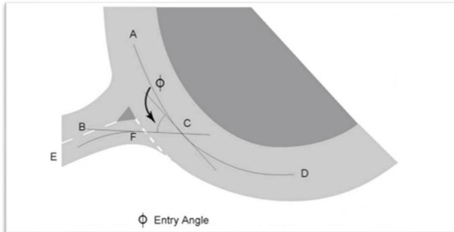
**Figure 6: Showing Vehicle Entry Angle Phi ( $\phi$ ) [11]**
