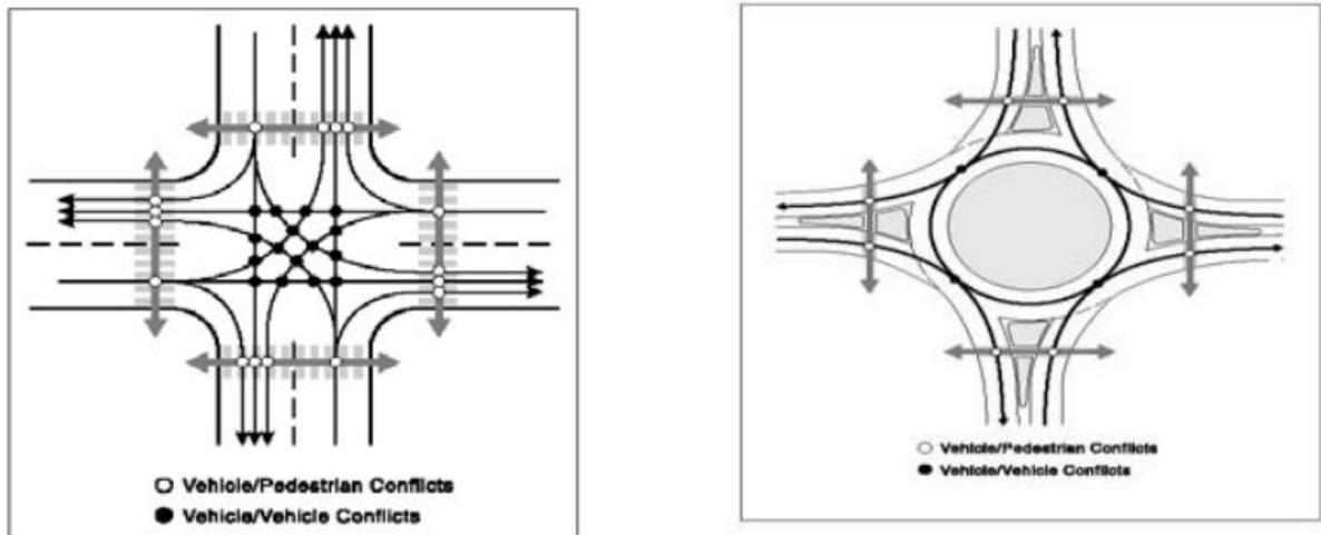
**Figure 8: Vehicle - Pedestrian conflict points at a Signalized Conventional Intersection compared to a Single-Lane Roundabout [2].**
