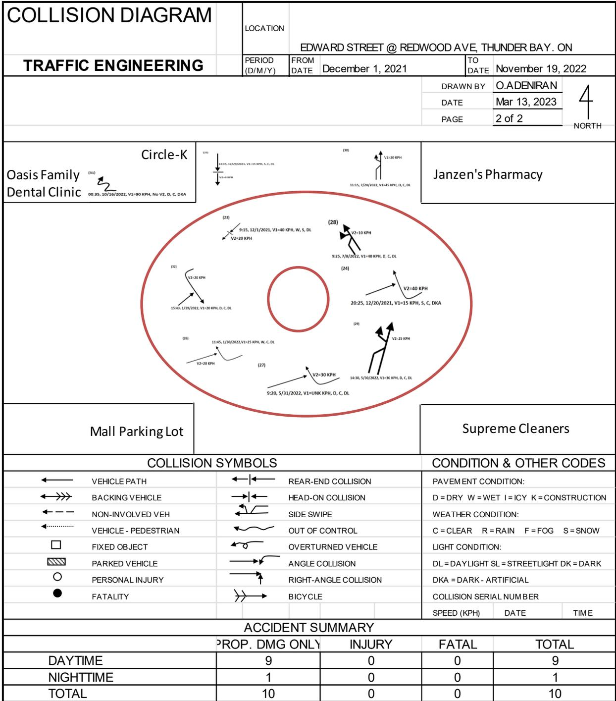
Figure 38: Collision Diagram for the intersection - After Roundabout Construction
