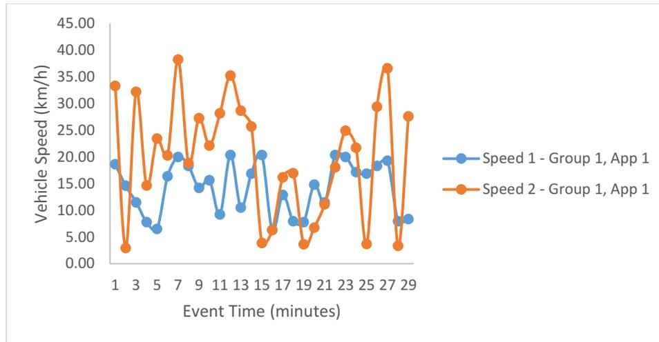
**Figure – I a: Vehicle Speed versus Time of Event's Occurrence without Treatment - Group 1 Approach 1. Each of the multiple vehicles monitored, passing through the scene has a pair of speeds named Speed 1 and Speed 2**
