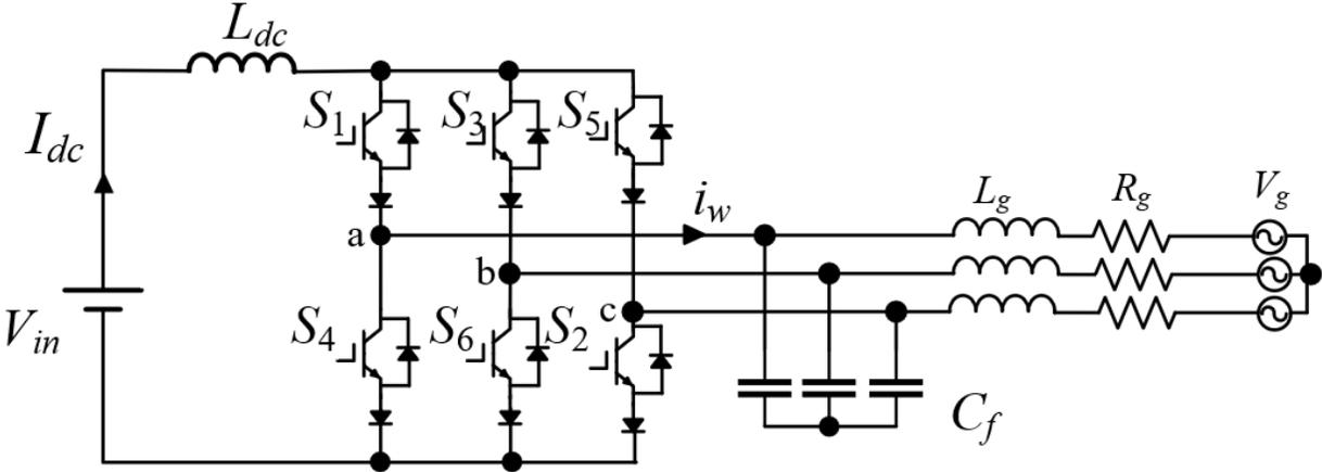
Figure-1-1 The conventional grid-tied CSI using IGBTs with series diodes.
