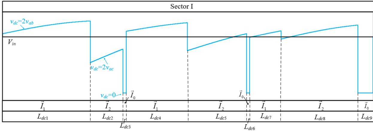
Figure 1-10 Waveforms of  $V_{in}$  and  $v_{dc}$  in Sector I for a conventional two-CSI system using SQ1 SVM,  $f_{sw}=540$  Hz.
