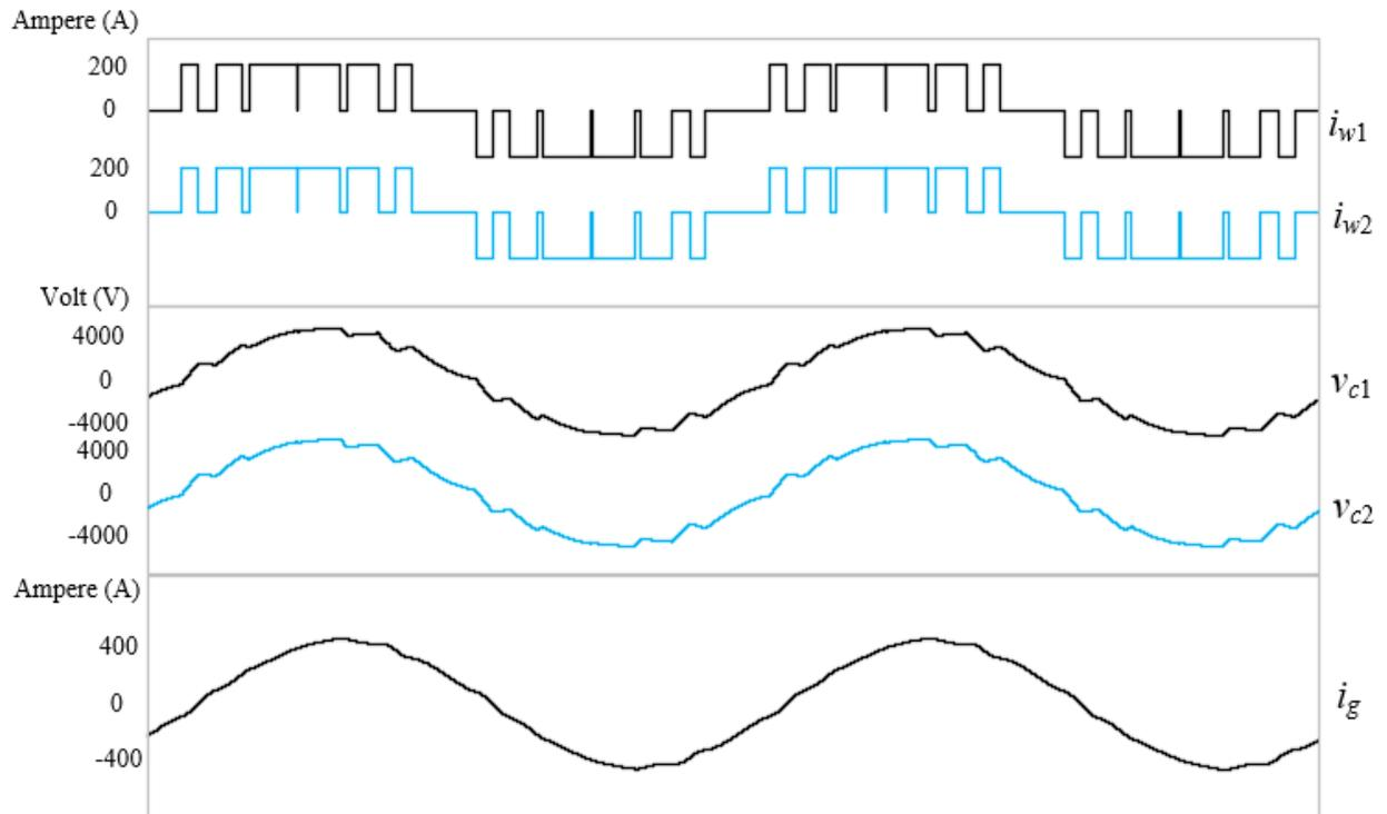
Figure 2-6 Simulated waveforms for a two-CSI system without active damping,  $f_{sw}=360$  Hz.
