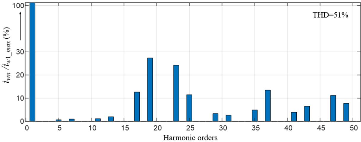
Figure 1-6 Harmonic spectrum of the inverter output current  $i_w$ .
