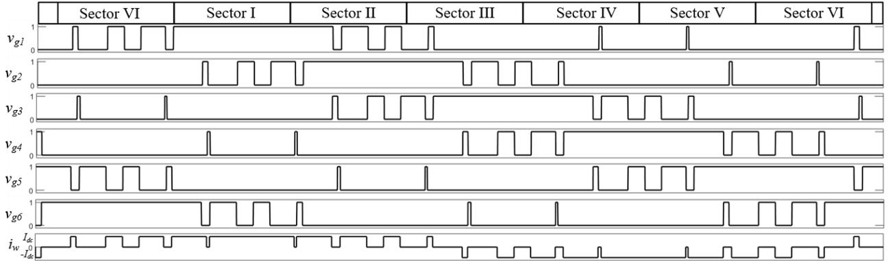
Figure 1-5 Switching sequence of SQ1 SVM,  $f_{sw}=540$  Hz,  $m_a=1.0$ .
