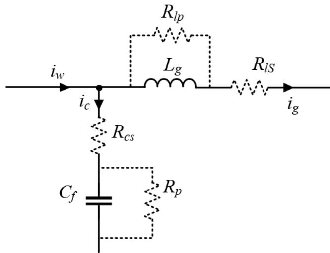
Figure 2-1 Possible locations of virtual resistors in an LC filter circuit [34].
