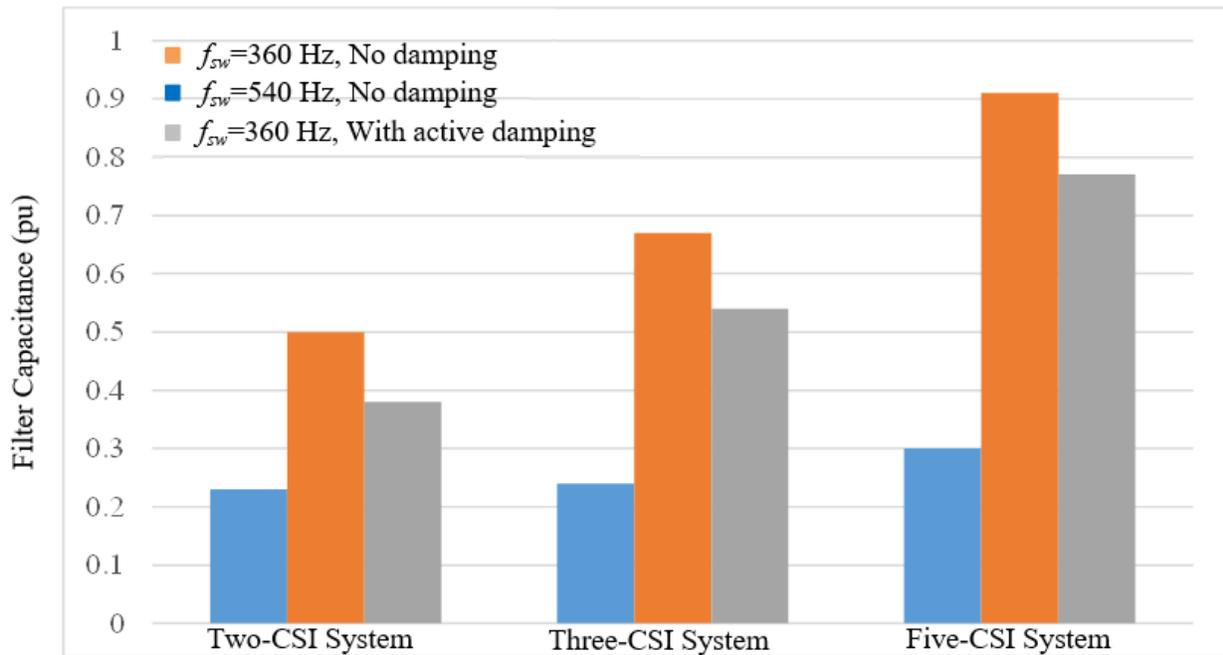
Figure 2-4 Comparison of filter capacitance of SC-CSIs.
