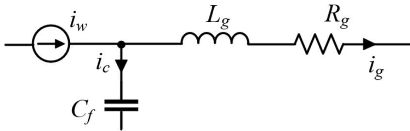
Figure 1-11 The output LC filter of a single CSI.
