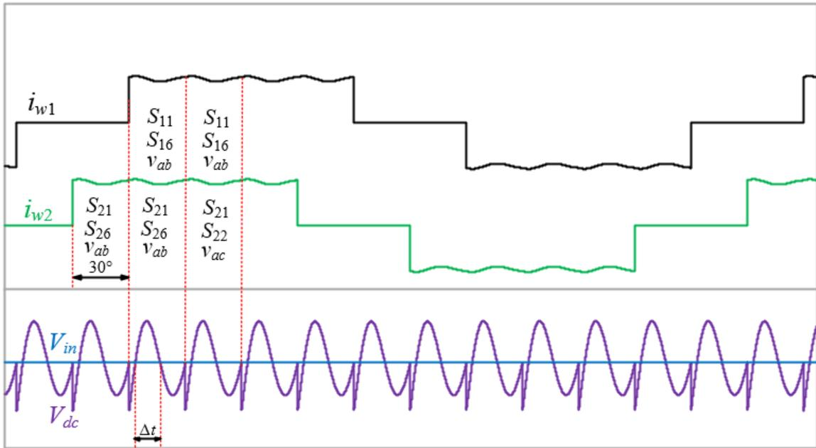
Figure 3-5 Waveforms of  $V_{in}$  and  $v_{dc}$  for a 60-Hz 2-SC-CSI.
