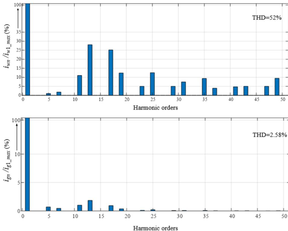
Figure 2-7 Harmonic spectrums of the inverter output current and grid current without active damping.
