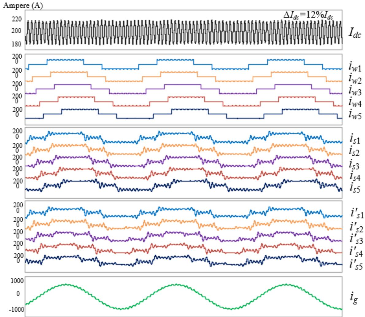
Figure 3-8 Simulated waveforms for a 60-Hz five-CSI.
