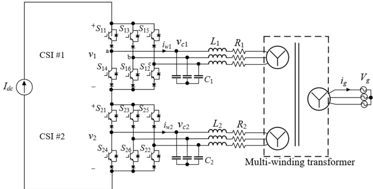
Figure 2-5 Simulation circuit for two-CSI systems.
