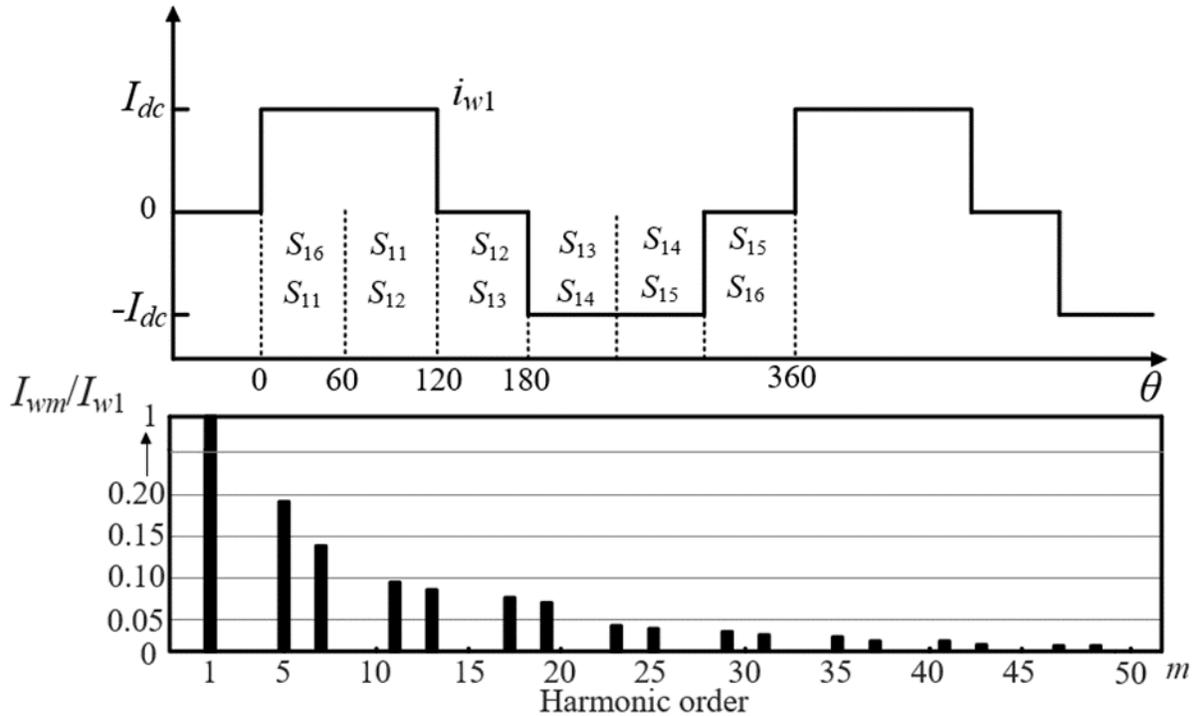
Figure 3-2 Waveform of inverter output current and its harmonic spectrum [42].
