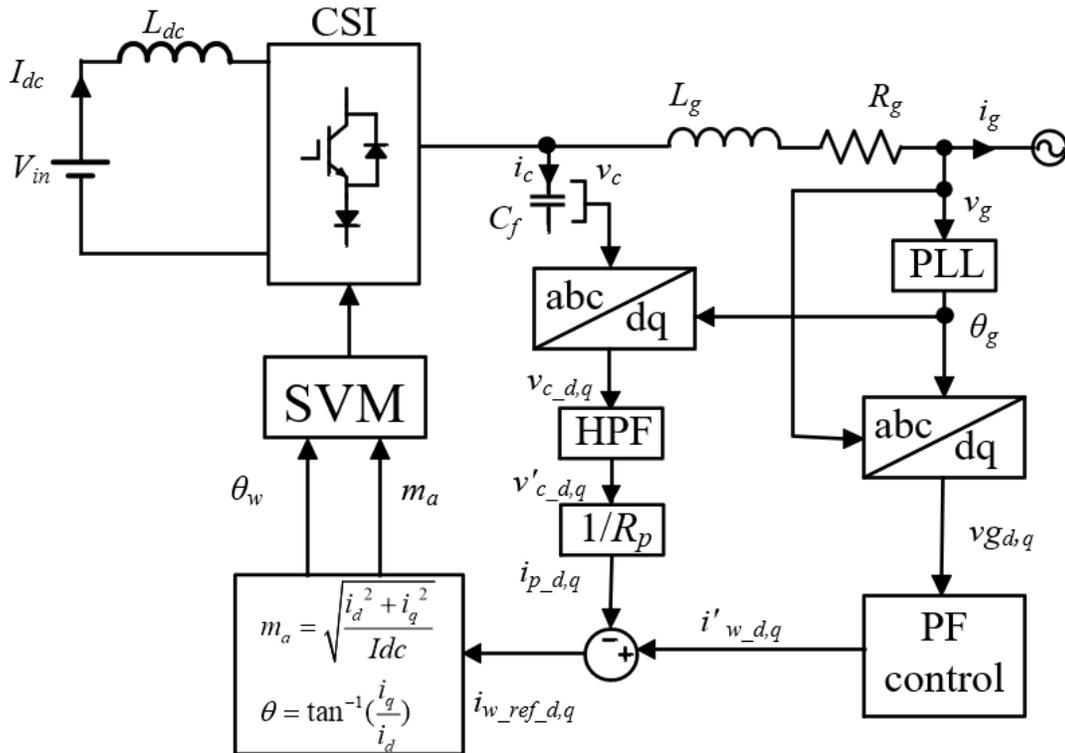
Figure 2-3 Block diagram of active damping control.
