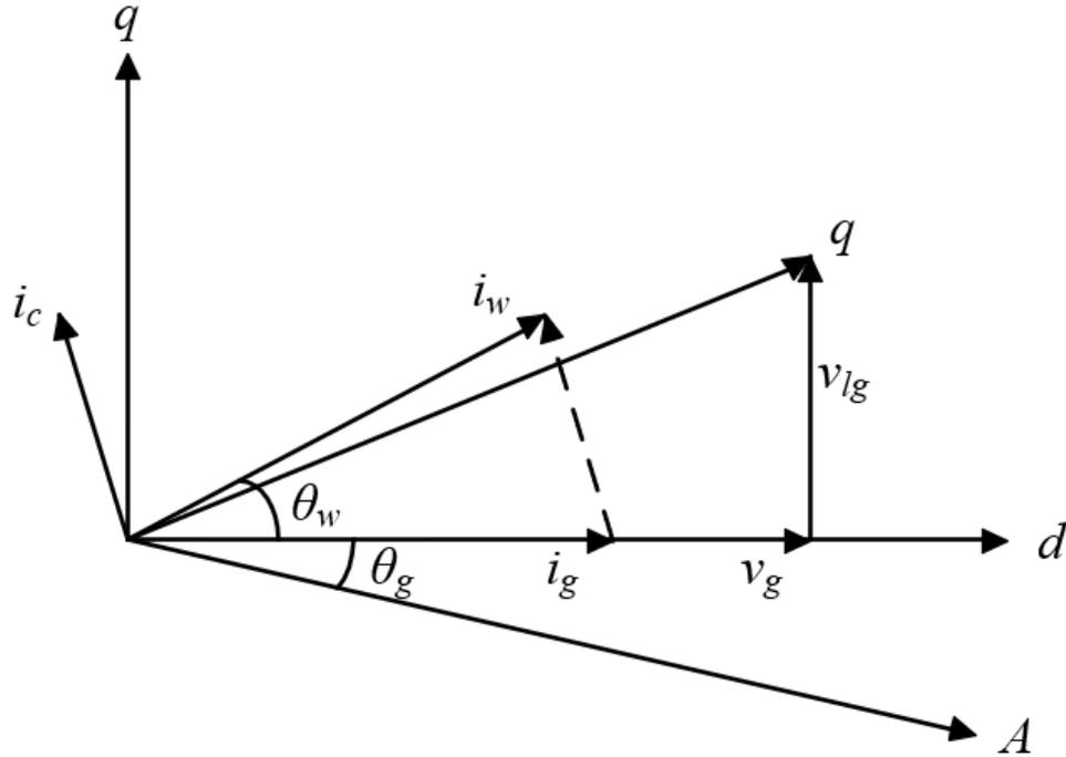
Figure 1-8 Phasor diagram of the PF control.
