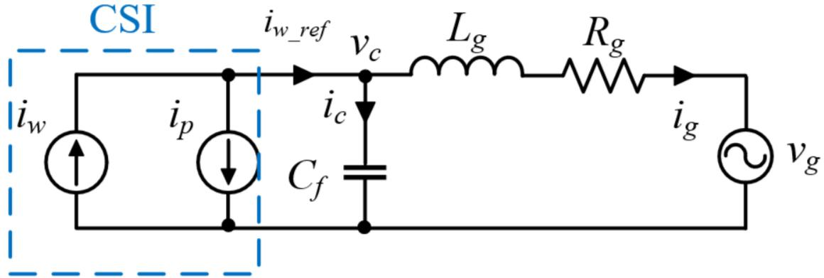
Figure 2-2 Equivalent circuit of a single CSI with active damping control.
