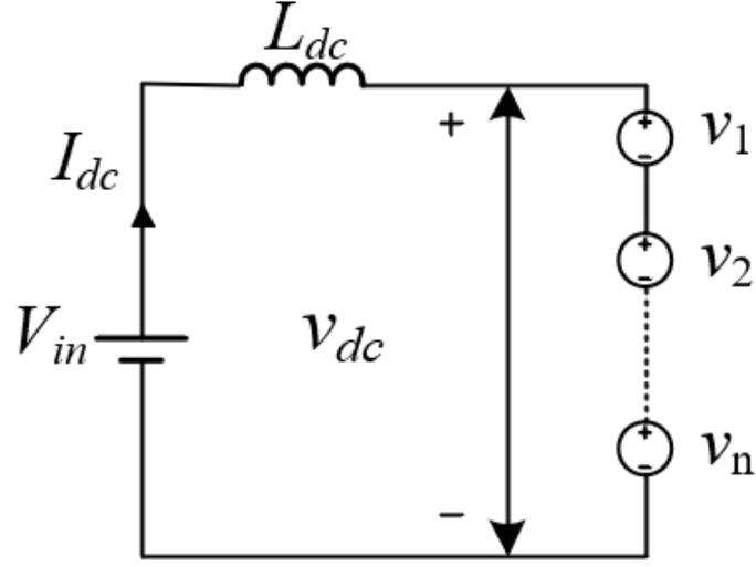
Figure 1-9 Equivalent circuit of a n-SC-CSI [24].
