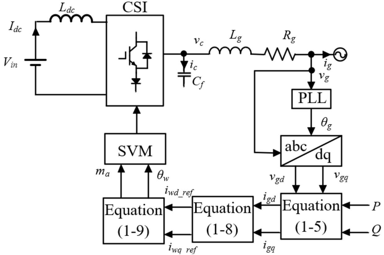
Figure 1-7 Block diagram of PF control.
