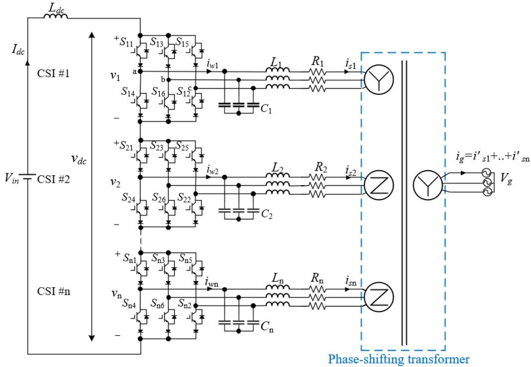
Figure 3-1 Topology of a 60-Hz n-SC-CIS.
