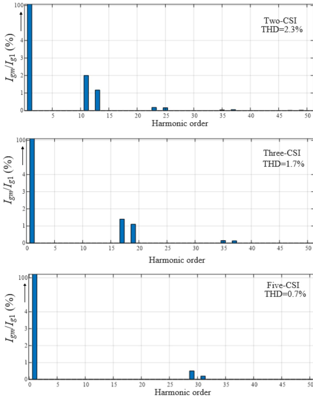
Figure 3-9 Harmonic spectrums of grid current  $i_g$  in 60-Hz SC-CSIs.
