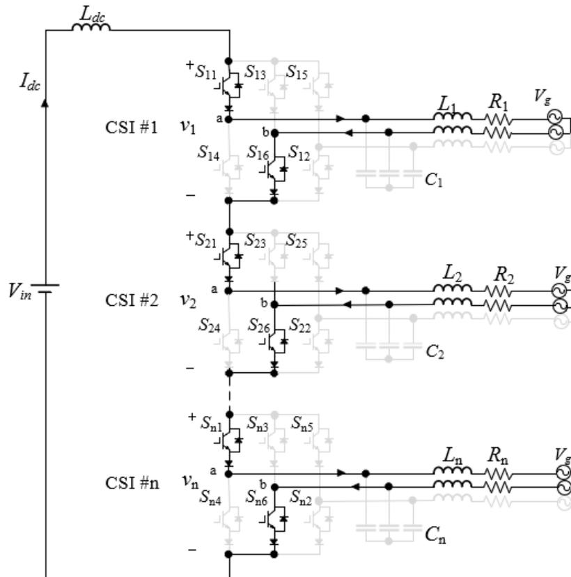
Figure 1-3 Equivalent circuit of a n-SC-CSI when  $S_1$  and  $S_6$  on.
