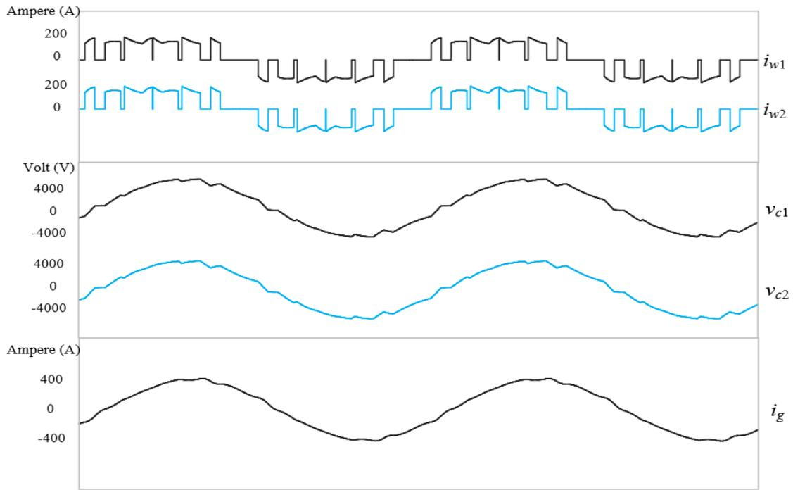
Figure 2-8 Simulated waveforms for a two-CSI system with active damping,  $f_{sw}=360$  Hz.
