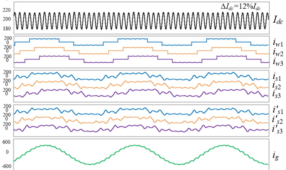
Figure 3-7 Simulated waveforms for a 60-Hz three-CSI.
