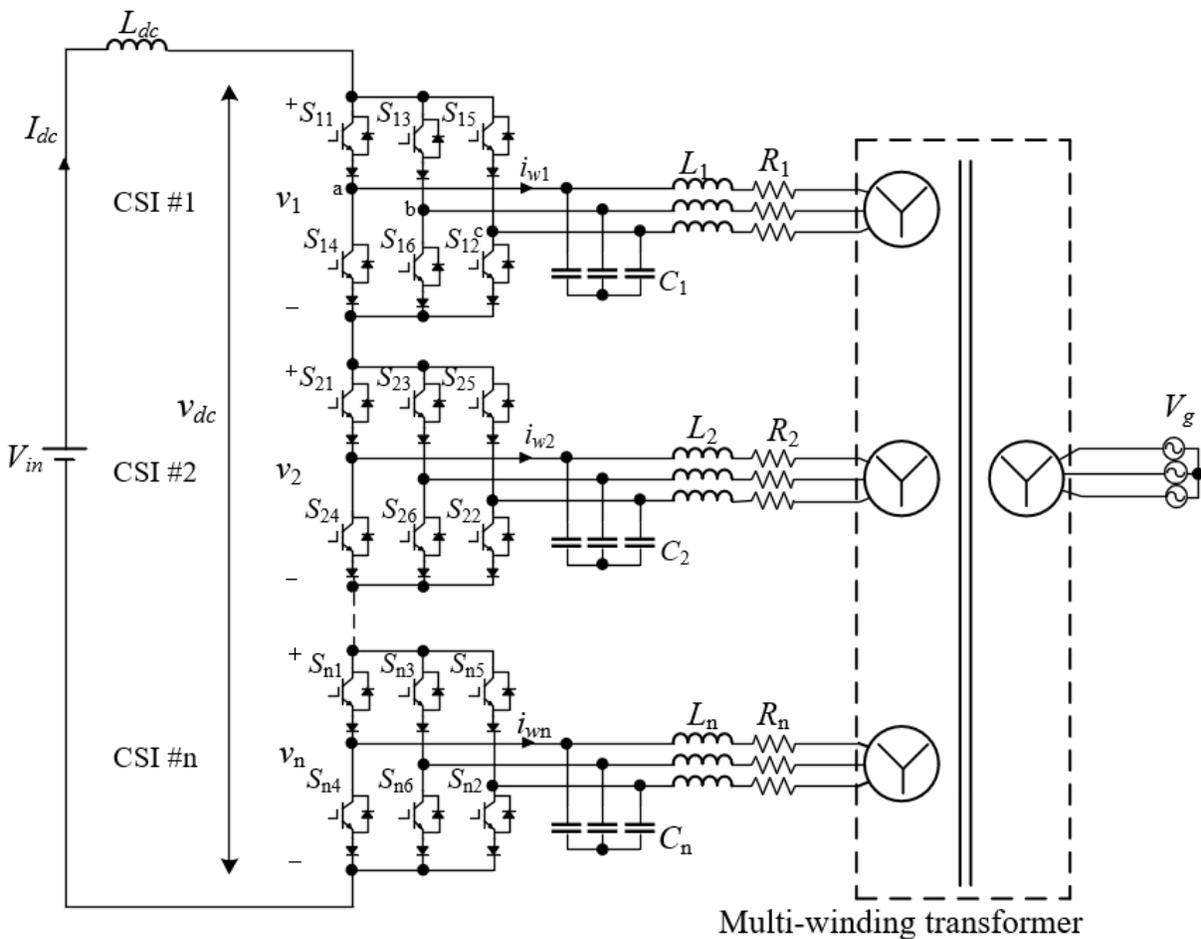
Figure 1-2 The conventional grid-tied n-SC-CSI.
