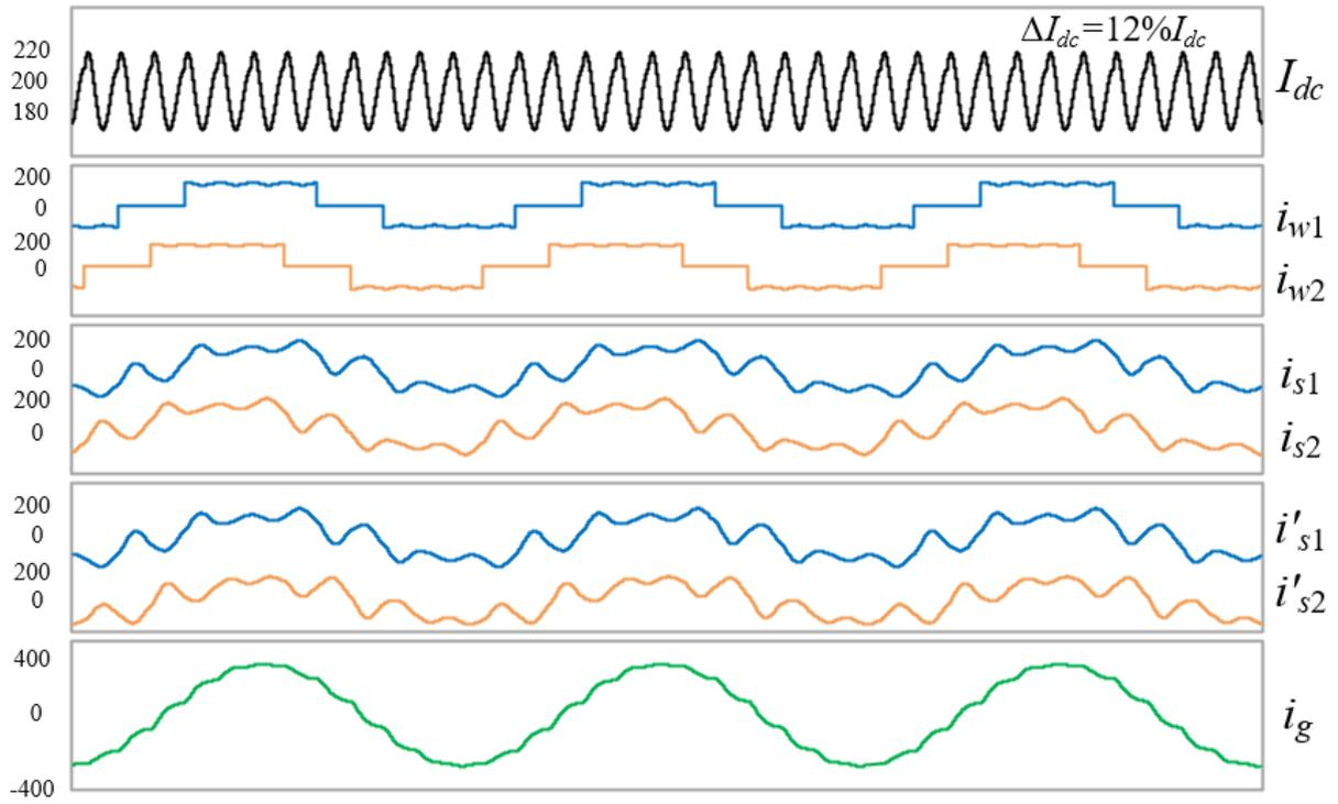
Figure 3-6 Simulated waveforms for a 60-Hz two-CSI.
