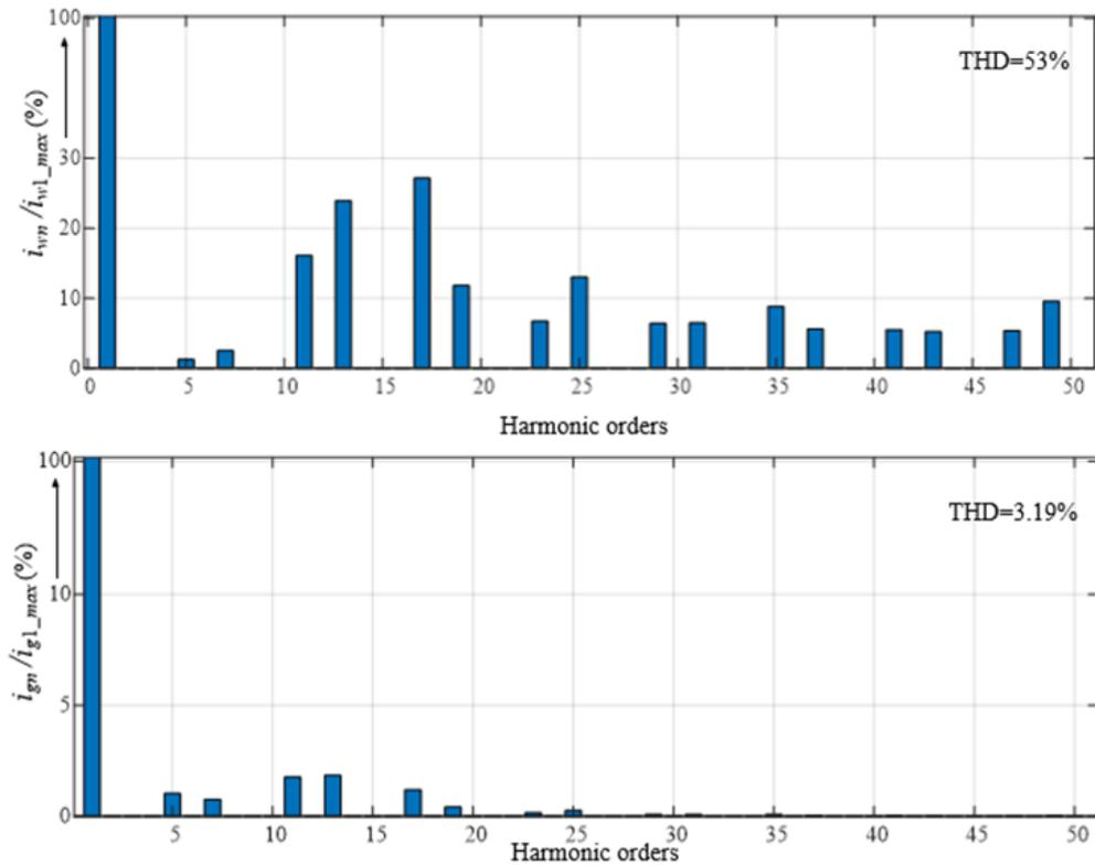
Figure 2-9 Harmonic spectrums of the inverter output current and grid current with active damping.
