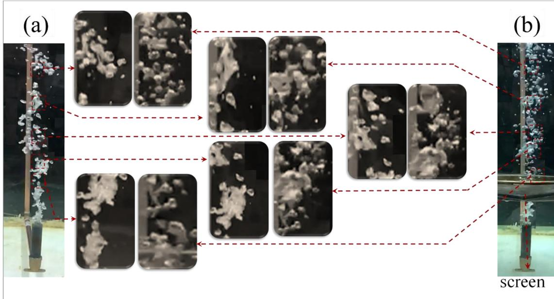
**Figure 2. 5:** Effect of grid-screen on bubble breakup at different distances from the nozzle for  $Q_a = 4$  L/min,  $d_o = 1$  mm: a) bubble plume without a grid-screen; b) bubble plume with a grid-screen,  $d_s = 0.841$  mm,  $X_s = 0.14$  m.
