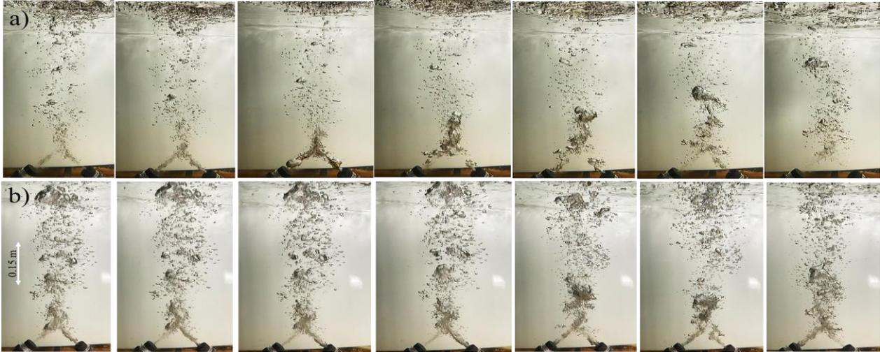
**Figure 6. 3:** Time-series images of Twin-Inclined (TI-Series) bubble jets. The time step between each image is 0.05 seconds: a) Test No.14 (TI1.11D3); b) Test No.16 (TI3.33D3).
