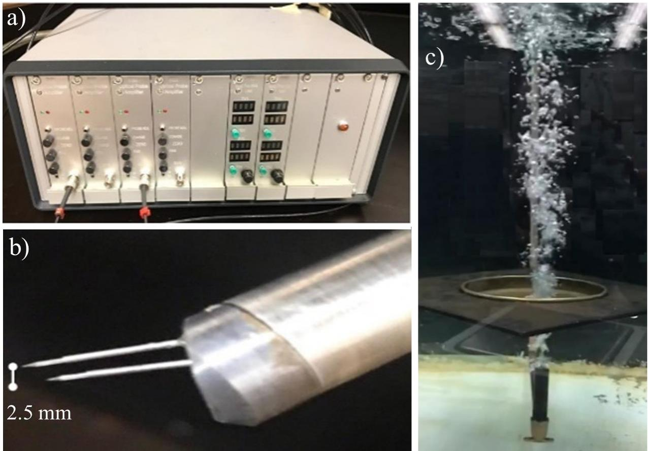
**Figure 4. 2:** Images of the RBI instrumentation and bubbly plume: a) RBI optoelectronic unit; b) double-tip optical fiber probe; c) vertical bubble plume passing through a grid-
