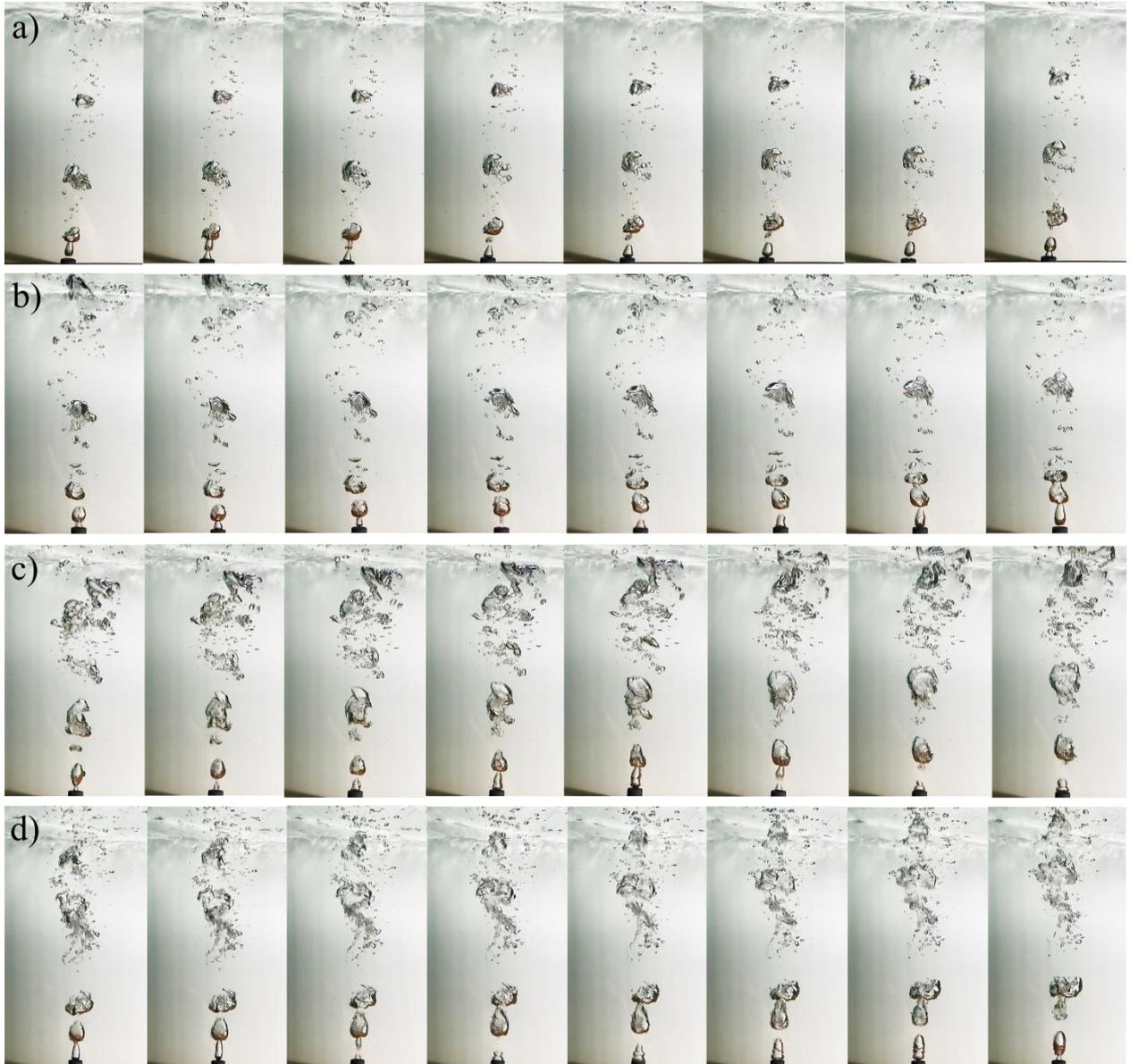
**Figure 3. 3:** Images of bubble plume variations with time for the plume tests with  $d_o = 3$  mm. The time step between each image is 0.07 seconds: a)  $Q_a = 3$  L/min; b)  $Q_a = 6$  L/min; c)  $Q_a = 9$  L/min; d)  $Q_a = 12$  L/min.
