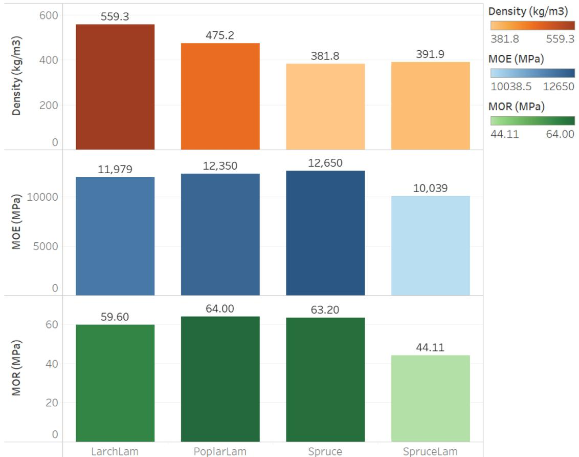
Figure 17. Graph comparing strength properties of spruce solid wood and laminated wood samples.
