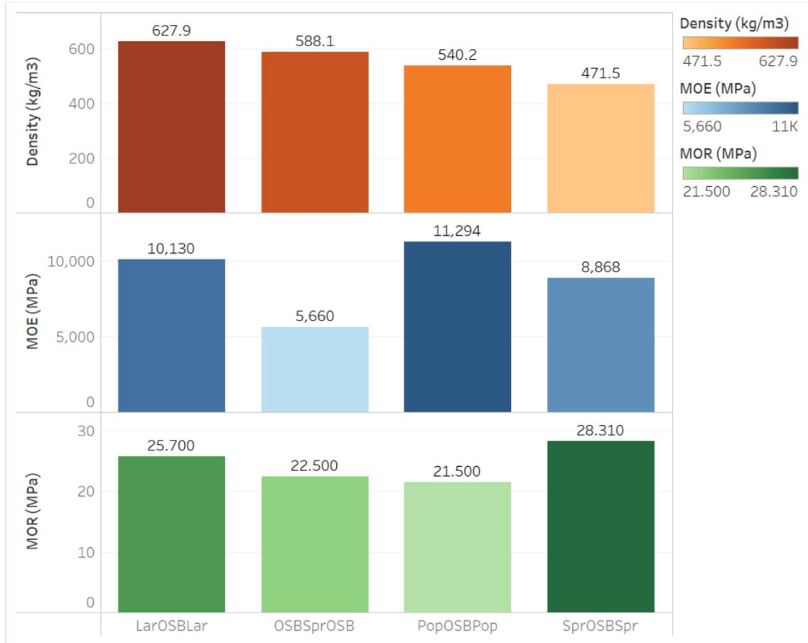
Figure 15. Graph showing comparison of strength properties of different combinations of OSB samples.
