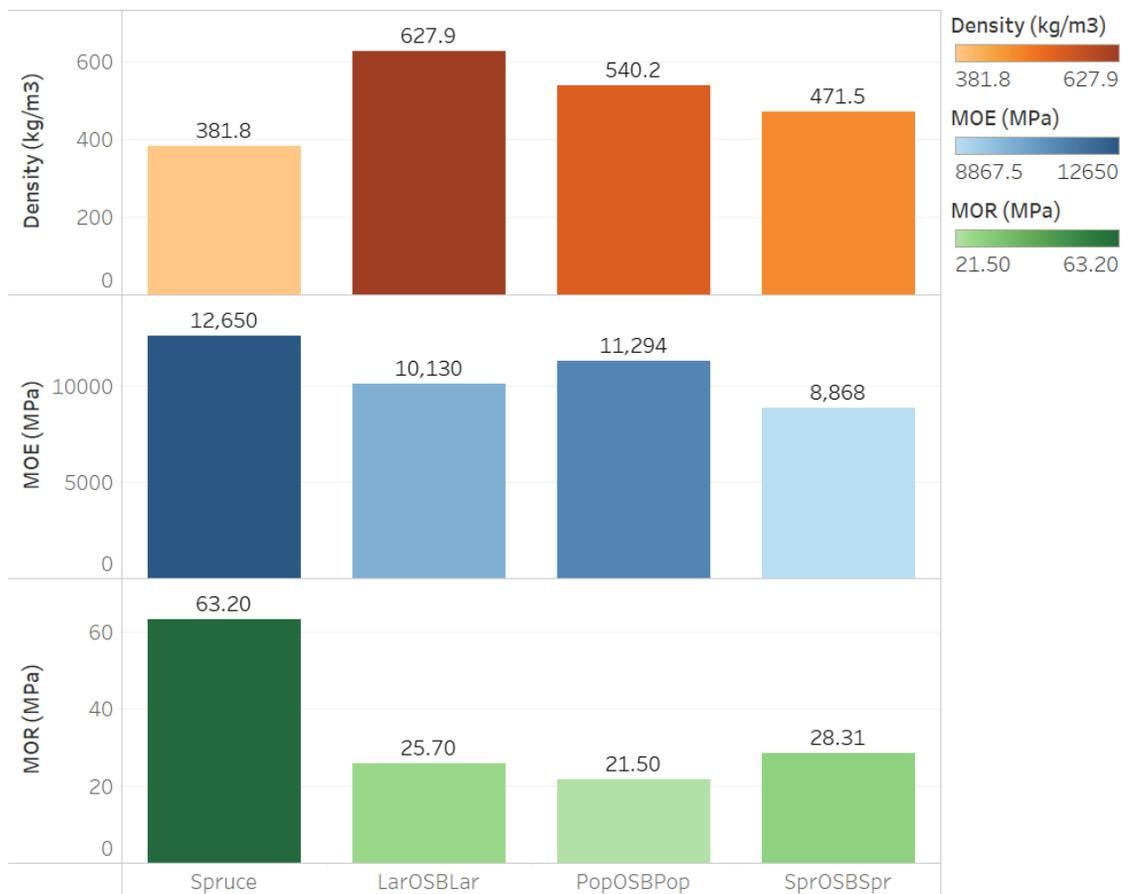
Figure 16. Graph comparing strength properties of spruce solid sample and OSB samples.
