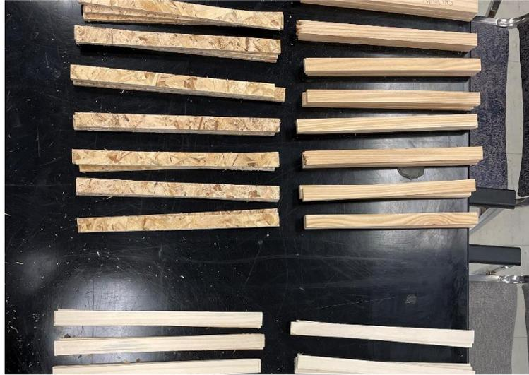
Figure 9 . Glued samples kept for drying.
