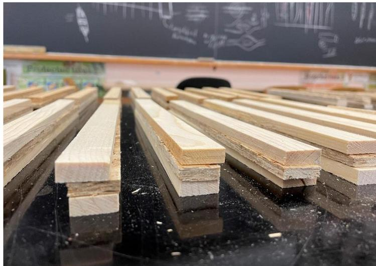
Figure 10 . Picture showing spruce sample glued with OSB as a neutral axis layer.
