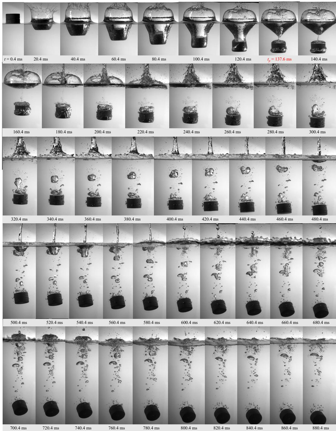
**Figure 3.5.** A sequence of snapshot images showing the water-entry of a thick disk and cavity formation by falling a gravity-driven hydrophobic solid disk in stagnant water, Test No. 16;  $\chi = 1.5$ ;  $\rho_d/\rho_w = 1.080$ ,  $h_r/d_o = 5.25$ . The time is tagged under each frame, and the pinch-off time  $t_p = 137.6$  ms.
