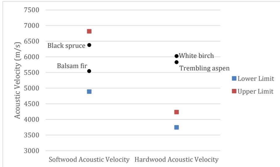
Figure 24. Comparison of tested acoustic velocity values to the published ranges.
