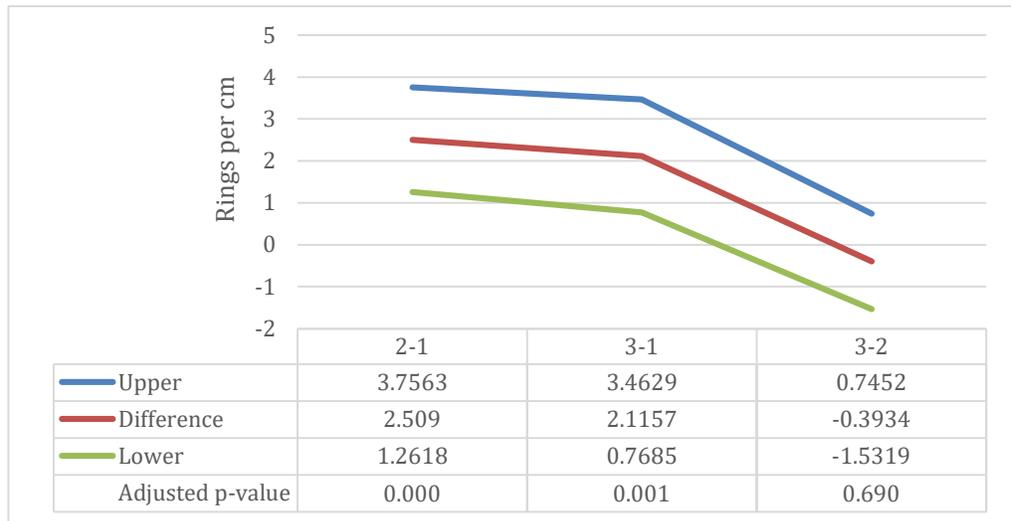
Figure 21. Host Hoc results for rings per centimeter between radial positions, where the red line shows the difference in values, the blue line show the upper limit, and the green line shows the lower limit.
