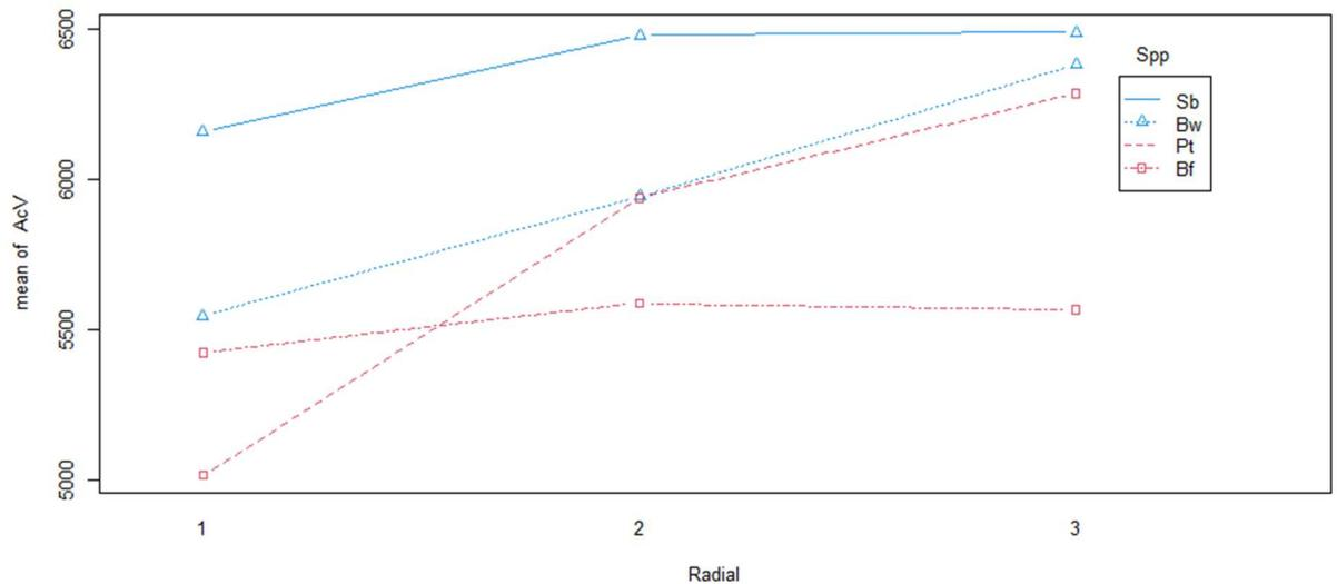
Figure 10. Comparison of mean acoustic velocity values of each species by radial position.
