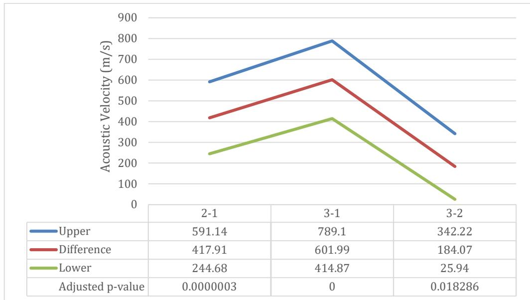
Figure 12. Post Hoc results for acoustic velocities between radial positions, where the red line shows the difference in values, the blue line show the upper limit, and the green line shows the lower limit.
