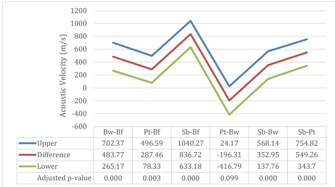
Figure 11. Post Hoc results for acoustic velocities between species, where the red line shows the difference in values, the blue line show the upper limit, and the green line shows the lower limit.
