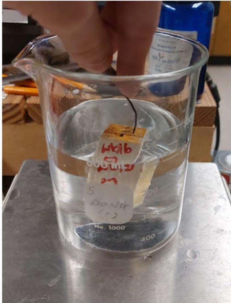
Figure 8. Density measurement using the water immersion method.
