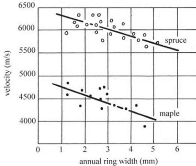
Figure 1. Ultrasonic velocity and annual ring width in resonance wood (Bucur 1984).
