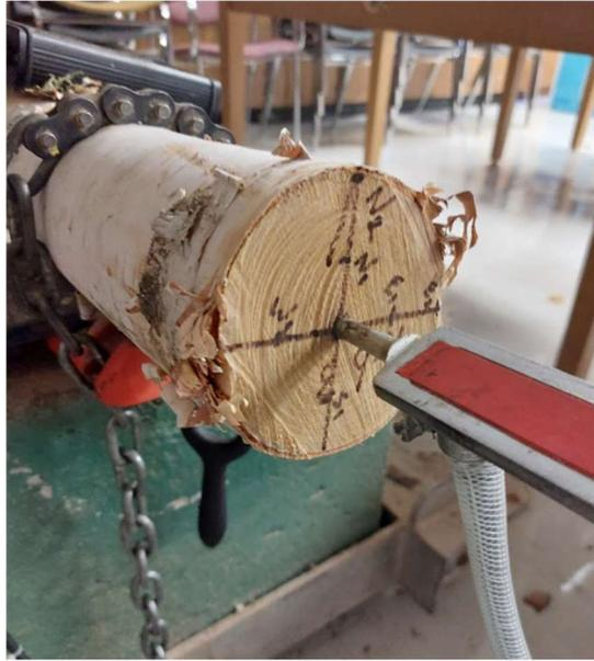
Figure 6. The start probe being inserted into the bottom of log Wb3.
