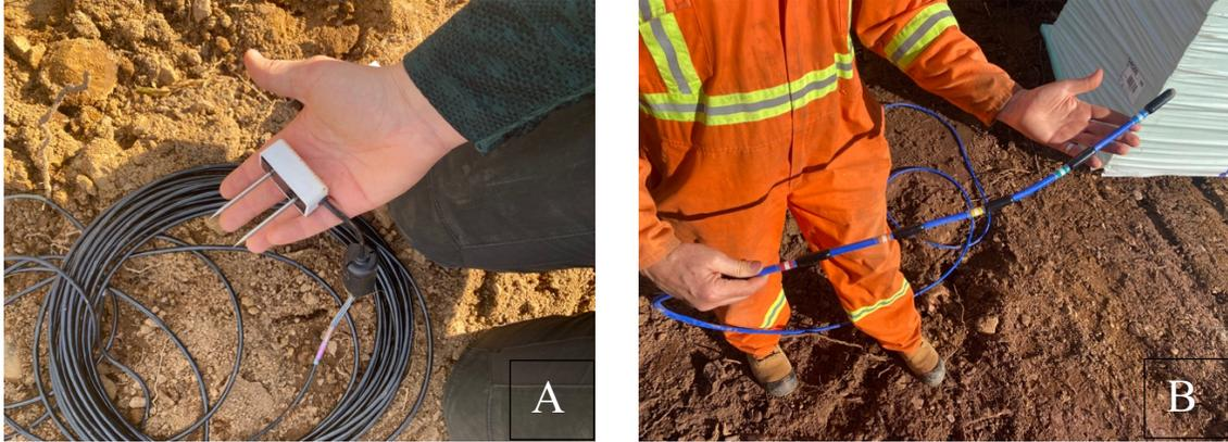
Figure 4. (A) TEROS 10 soil moisture sensor, and (B) five 44007RC Precision Epoxy NTC thermistors arranged in a single cable (or thermistor stack)..
