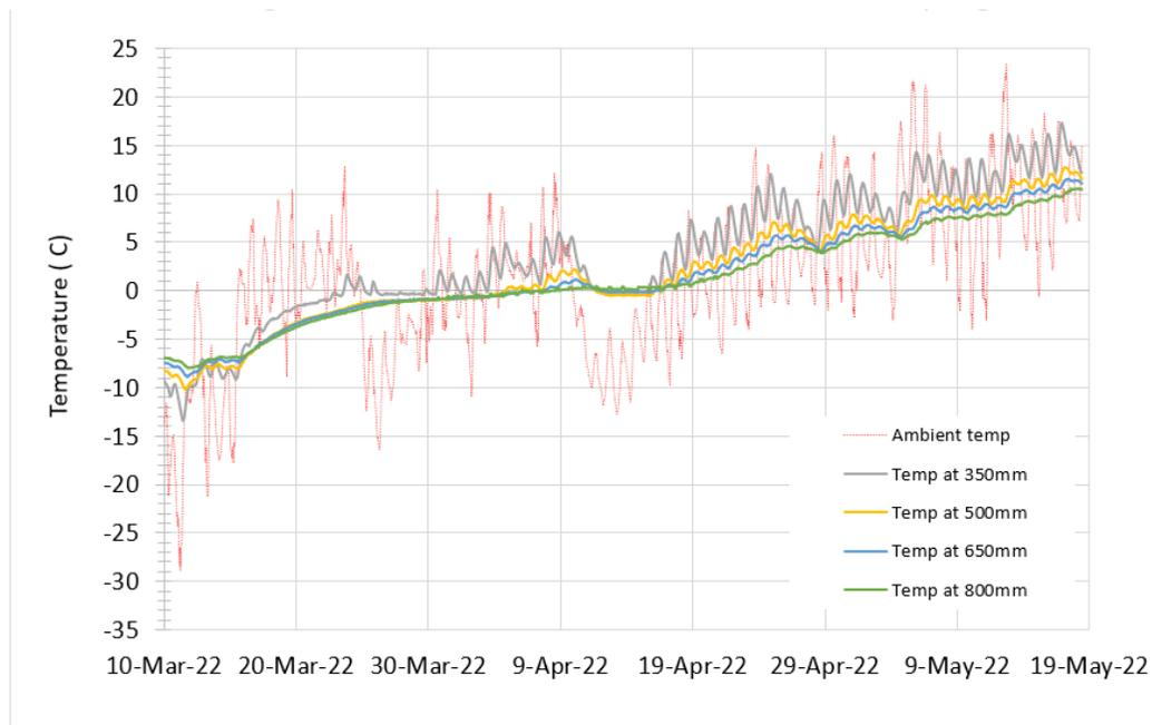
Figure 1. Roadbed thawing in insulated SK resource road during spring 2022.
