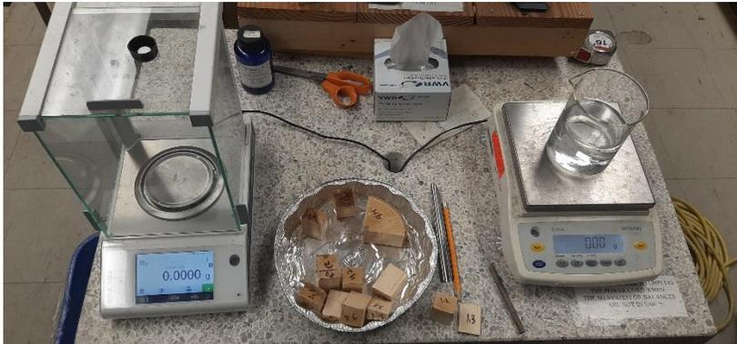
Figure 2 - Wood density instruments
