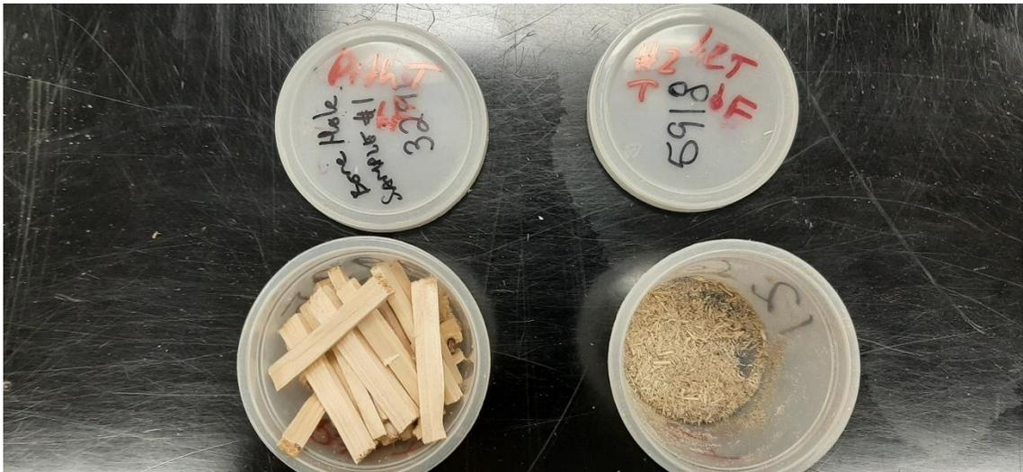
Figure 5 - chipped and ground wood samples
