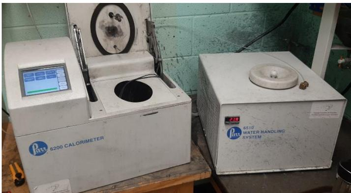
Figure 3 - Bomb calorimeter
