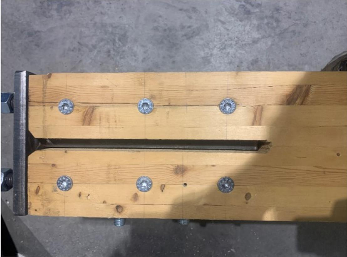
**Figure 3.16** Top view of the glulam beam showing 6 STS installed.
