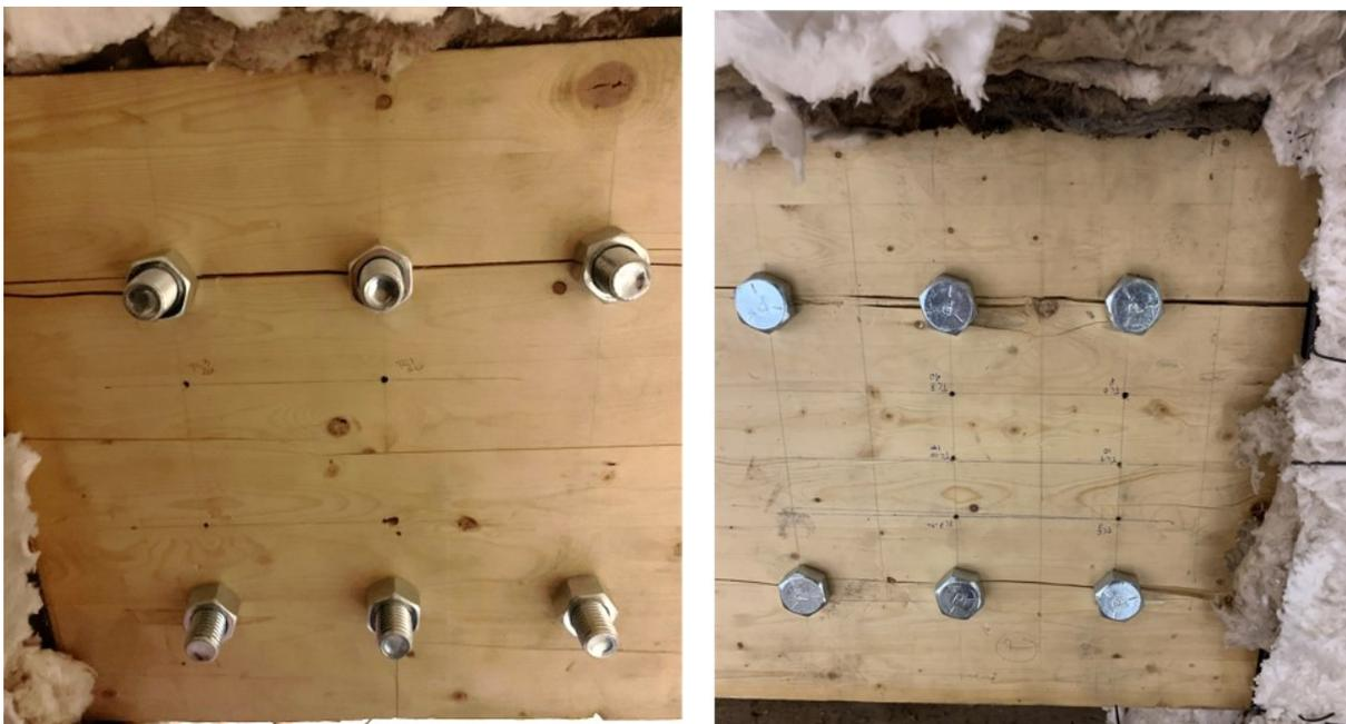
**Figure 4.3** Initial state of the STS-retrofitted, unprotected connection configuration that utilized six bolts in the first bolt pattern (6BP1NP).
