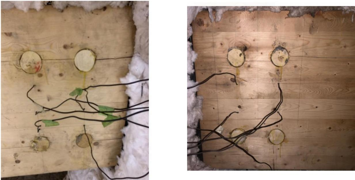
**Figure 4.9** Initial state of the STS-retrofitted, protected connection configuration that utilized four bolts in the first bolt pattern (4BP1P).
