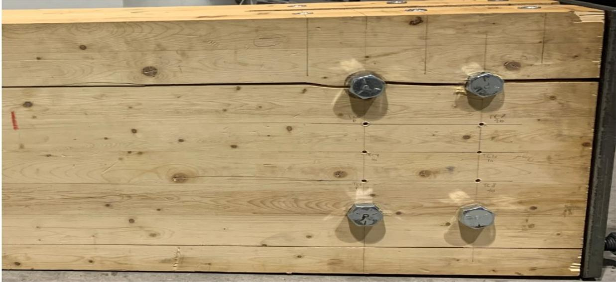
**Figure 4.1** Initial state of the STS-retrofitted, unprotected connection configuration that utilized four bolts in the first bolt pattern (4BP1NP).
