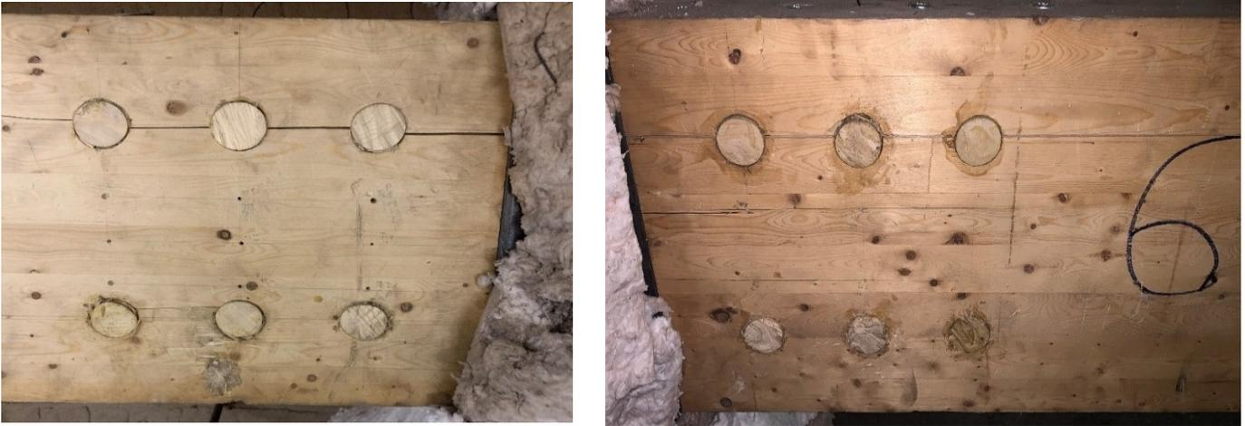
**Figure 4.11** Initial state of the STS-retrofitted, protected connection configuration that utilized six bolts in the first bolt pattern (6BP1P).
