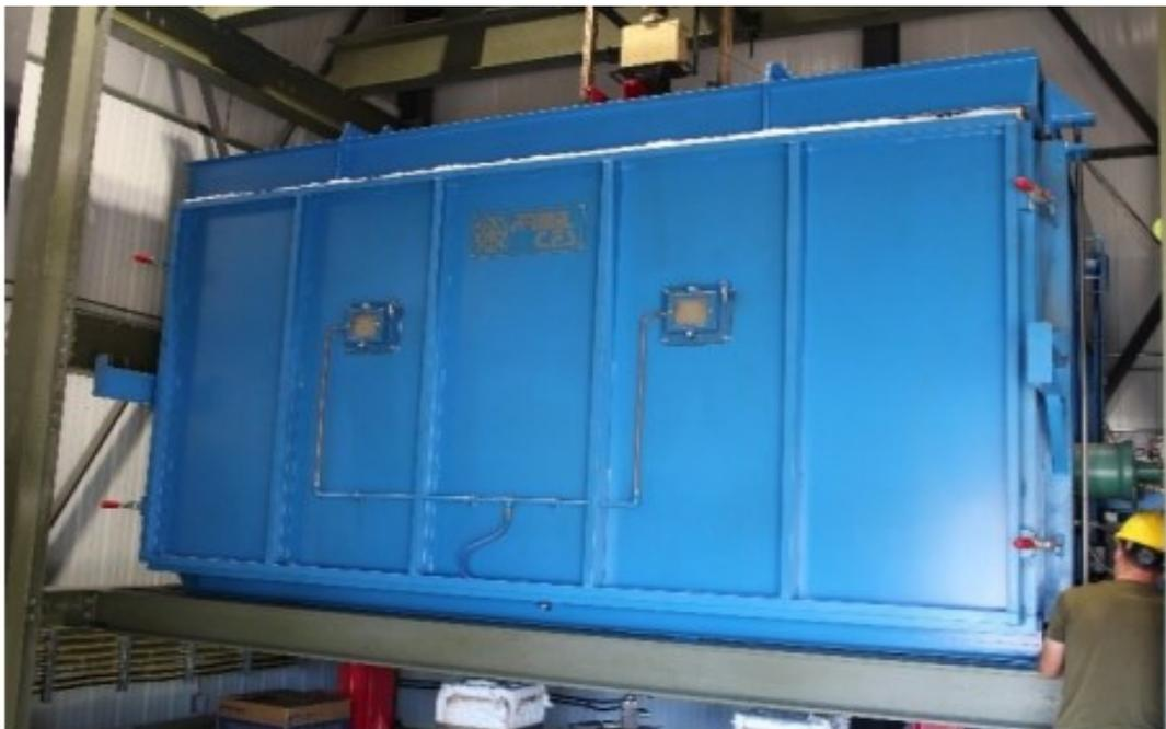
**Figure 3.9** Fire testing furnace (Courtesy of Dr. Salem, 2019).
