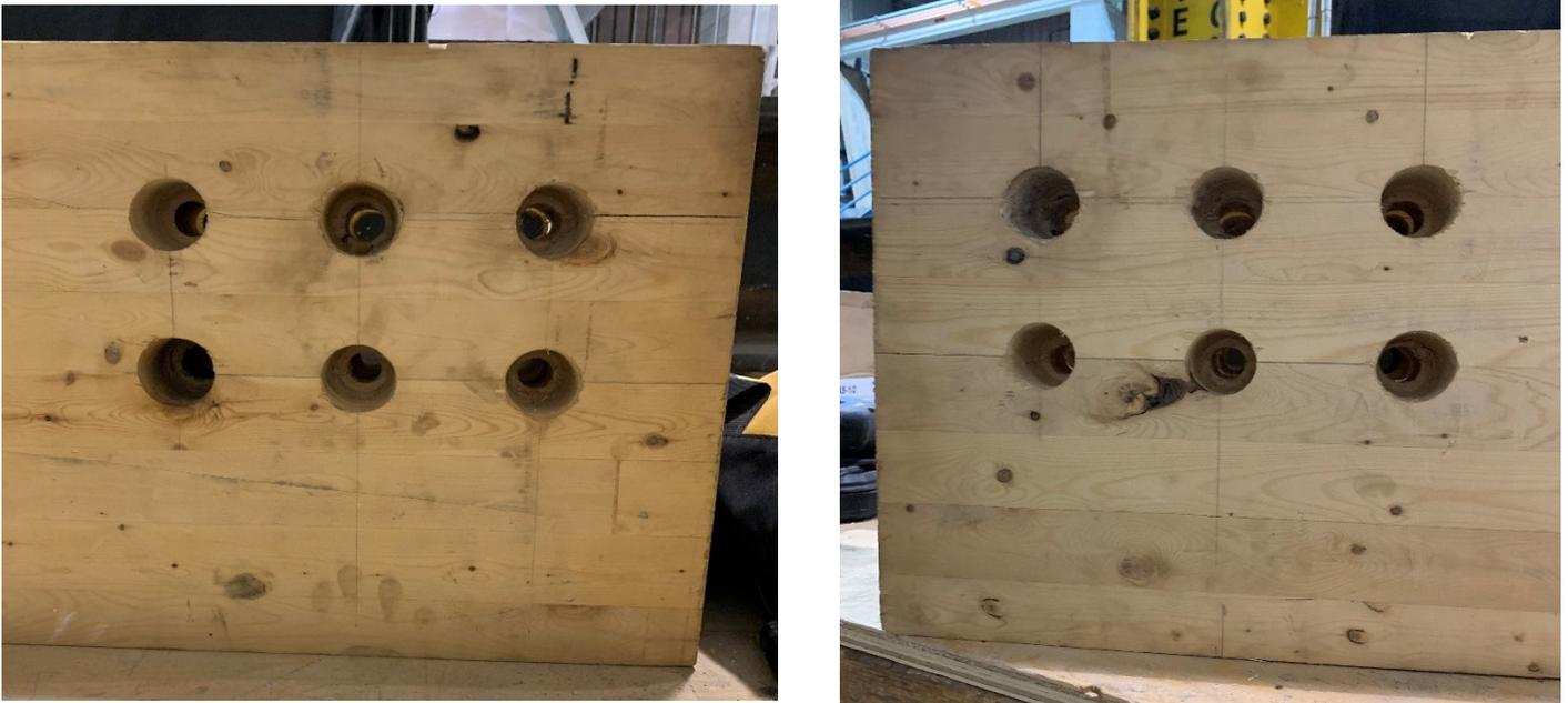
**Figure 4.15** Initial state of the STS-retrofitted, protected connection configuration that utilized six bolts in the second bolt pattern (6BP2P).
