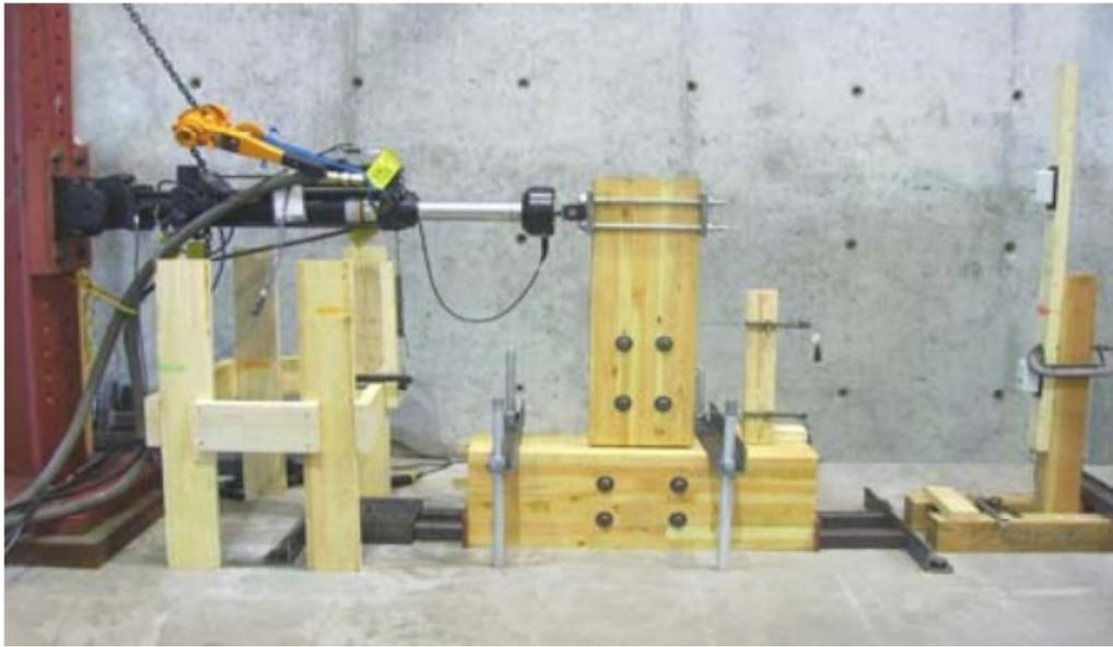
**Figure 2.19** Bolted connection Test Set Up (Adapted from Lam et al., 2008).
