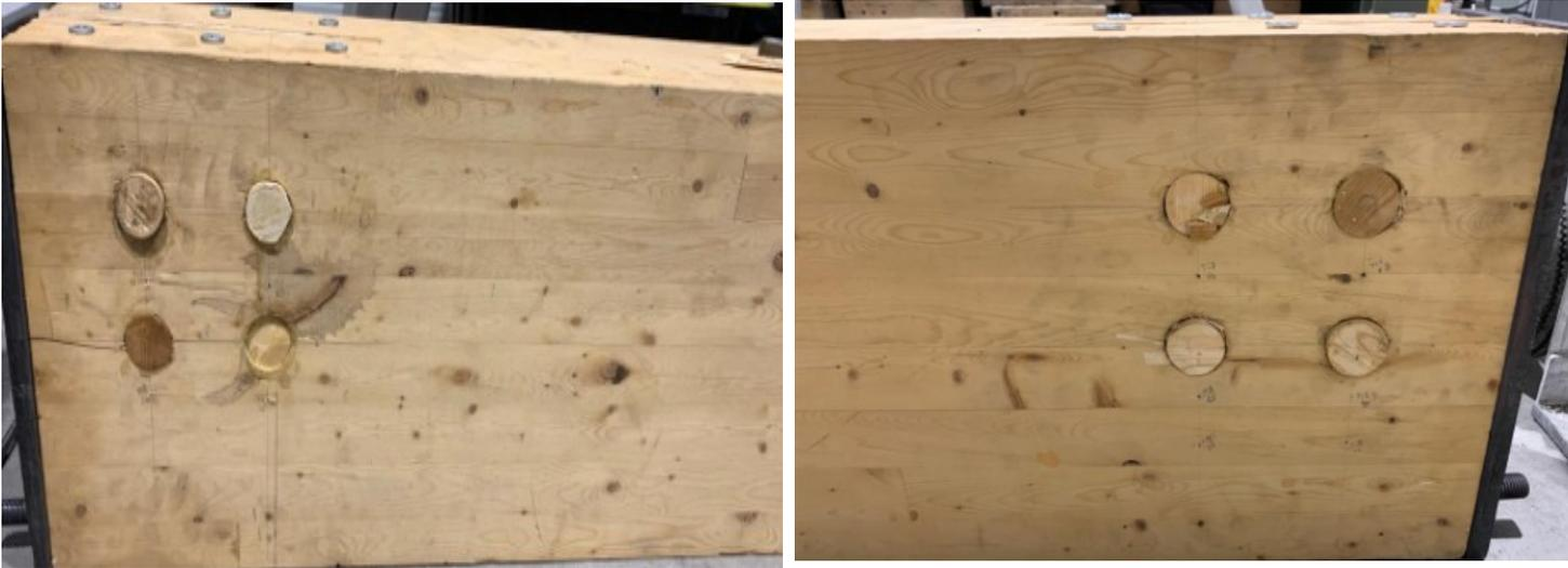
**Figure 4.13** Initial state of the STS-retrofitted, protected connection configuration that utilized four bolts in the second bolt pattern (4BP2P).
