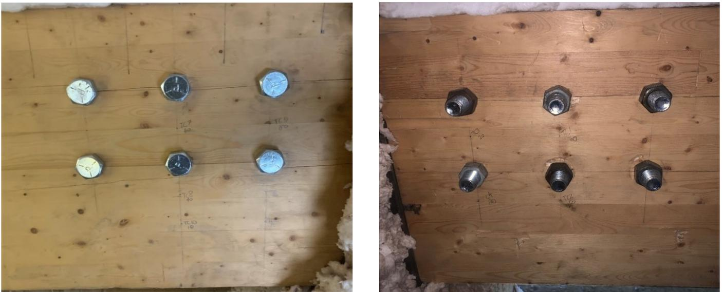
**Figure 4.7** Initial state of the STS-retrofitted, unprotected connection configuration that utilized six bolts in the second bolt pattern (6BP2NP).
