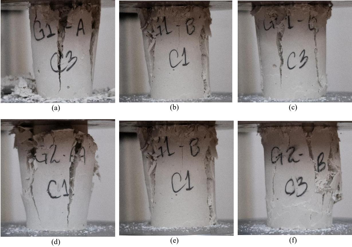
**Figure 4.7** Effect of fiber length (a-6mm, b-13mm, and c-19mm) and fiber content (d-0.25wt%, e-0.5wt%, and f 0.75wt%) on the post-peak failure patterns of 90-day FR-CPB.
