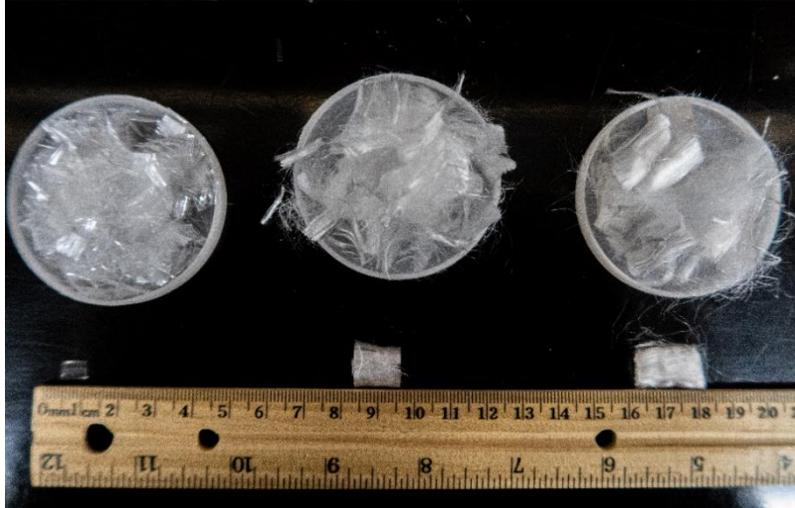
**Figure 3.2** Adopted polypropylene fibers - from left to right: 6 mm, 13 mm, and 19 mm.
