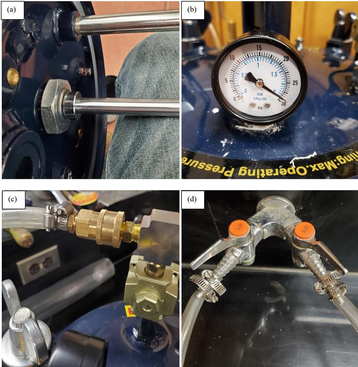
**Figure 3-5** Modifications to the Levlor Sprayer Tanks (a) internal rods (b) pressure gauge (c) quick connect coupler and regulator (d) laboratory supply outlets.
