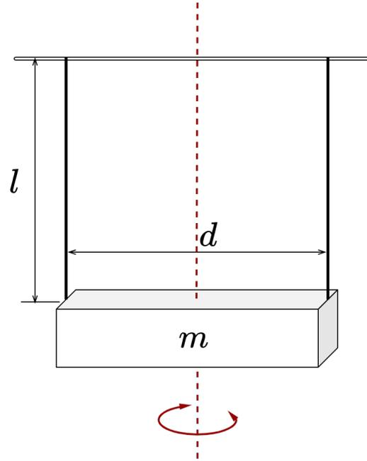
Figure 3.3: The bifilar pendulum principle model
