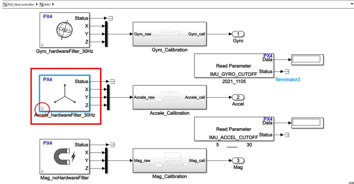
Figure 5.17: IUM model for reading the IMU data from Pixhawk 4
