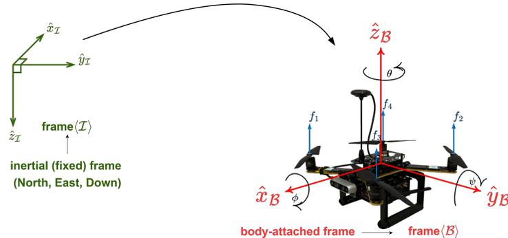
Figure 2.1: Configuration of the inertial frame  $\mathcal{I}$  and the body frame  $\mathcal{B}$
