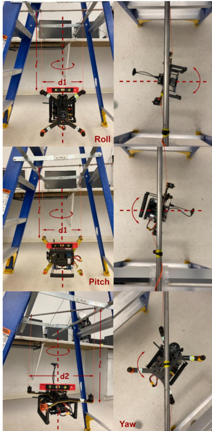
Figure 3.4: The experimental setup of bifilar pendulums for moments of inertia measurements
