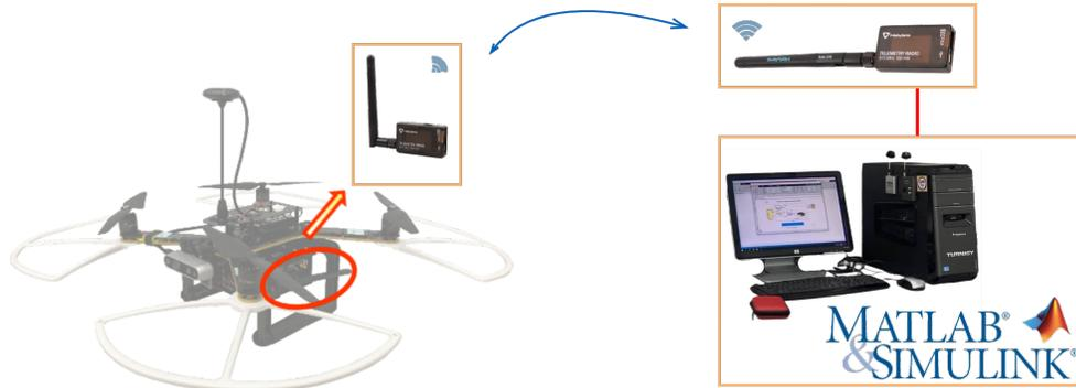
Figure 5.8: Radio serial 1 module (left) and radio USB module (right)
