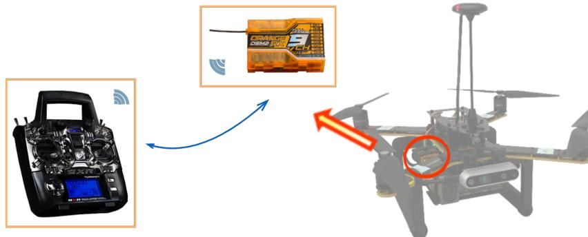
Figure 5.7: Turnigy 9XR transmitter (left) and ORX R910 DSM2 receiver (right)
