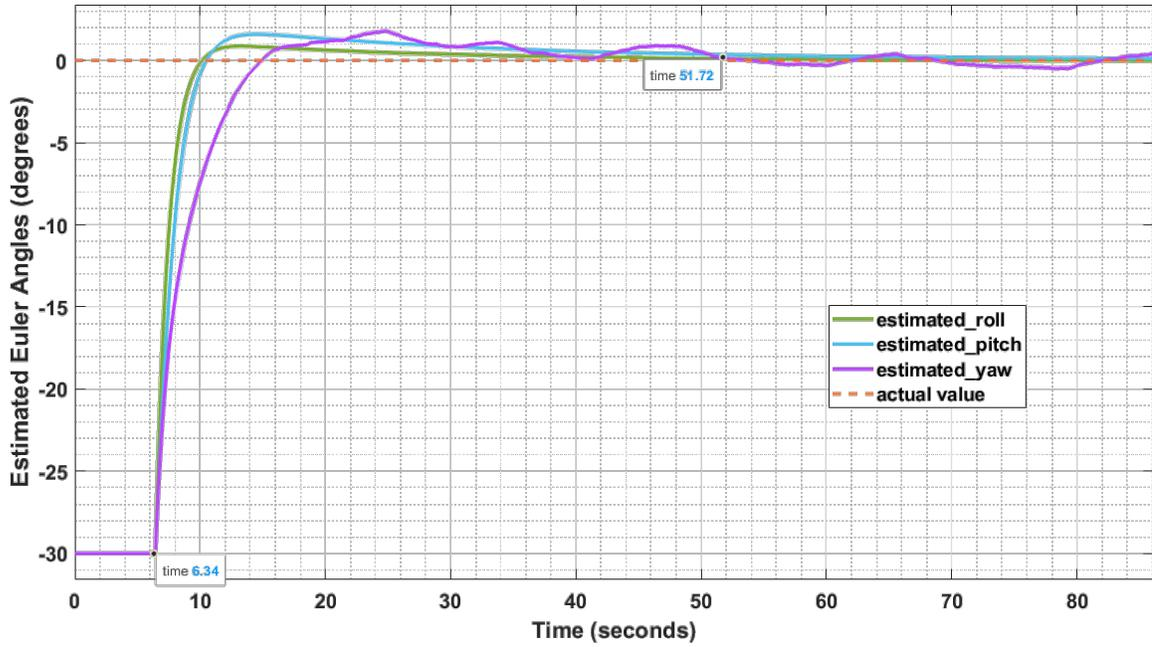
Figure 4.2: Real-time estimation for static attitude
