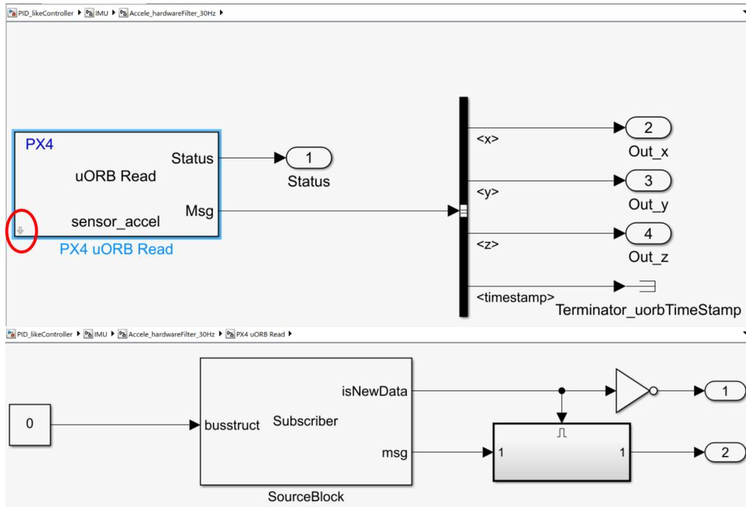
Figure 5.20: PX4 *sensor\_accel* uORB Read block (top) and the block details (bottom)
