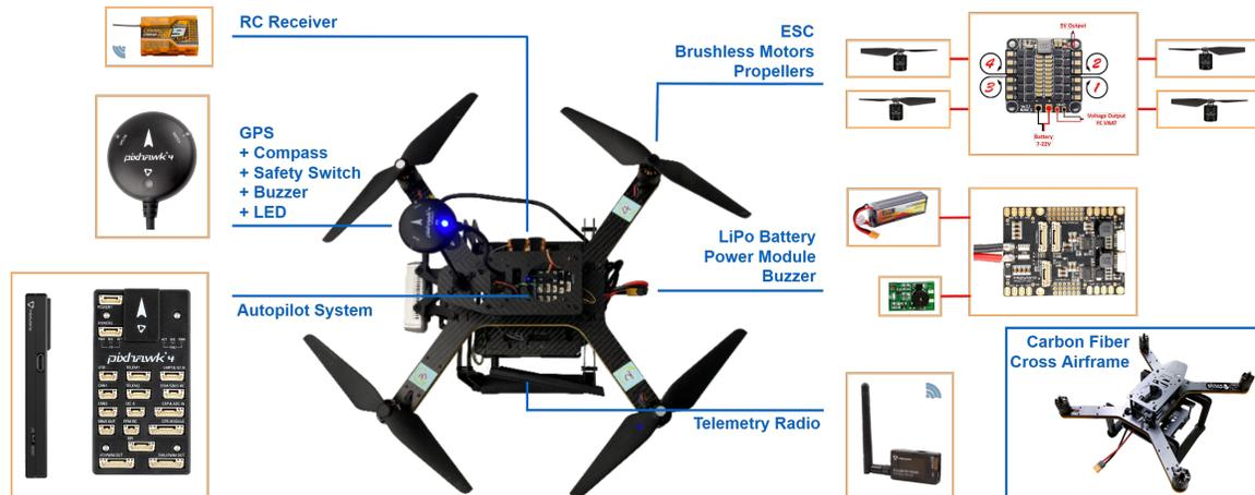
Figure 5.3: Overview of the quadrotor hardware
