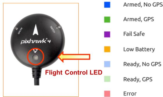
Figure 5.6: M8N GPS with the tri-colored LED indicator
