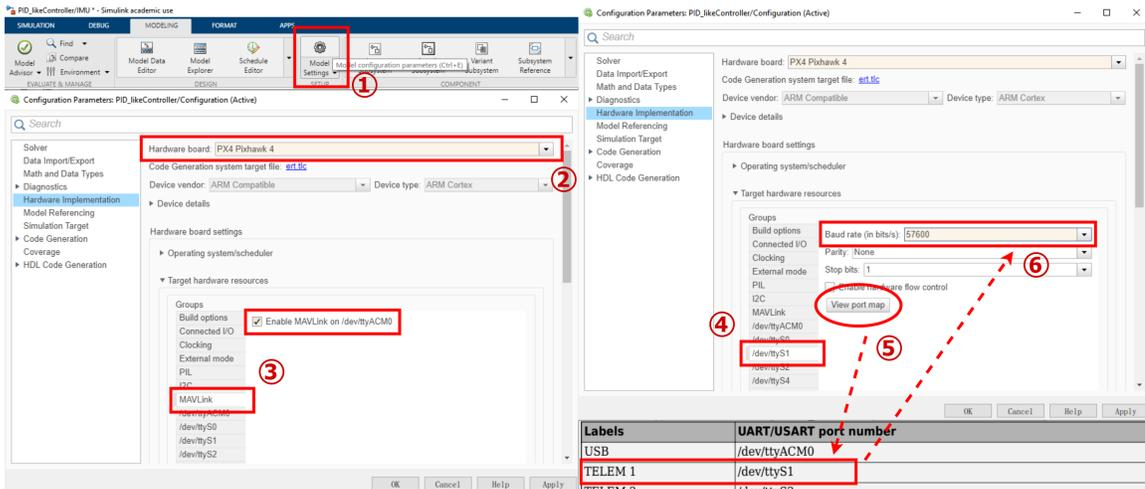
Figure 5.15: Configure the model for Pixhawk hardware
