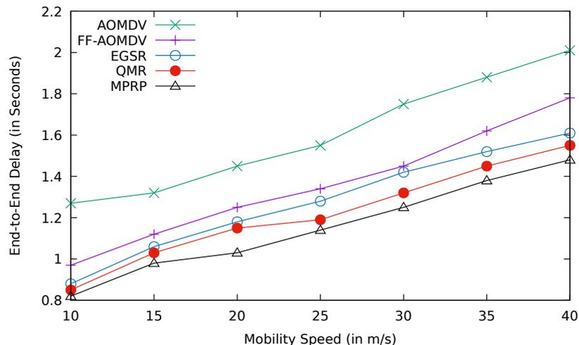
**Fig. 4.44:** Comparison between AOMDV, FF-AOMDV, EGSR, QMR and proposed protocol MPRP for end-to-end delay with mobility speed.
