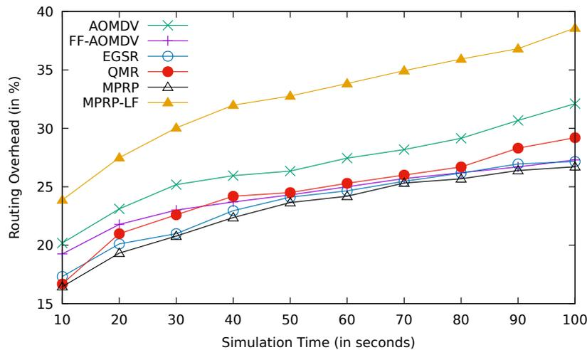
**Fig. 4.9:** Comparison between AOMDV, FF-AOMDV, EGSR, QMR and proposed protocol MPRP and MPRP-LF for routing overhead with simulation time.
