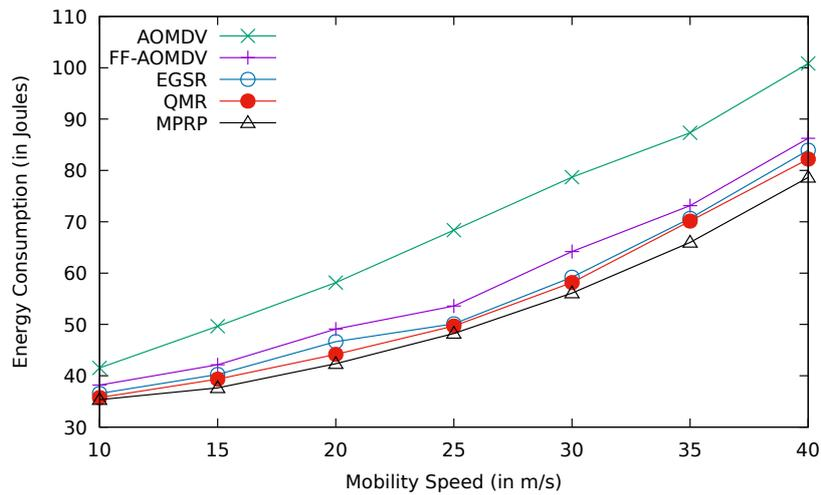
**Fig. 4.45:** Comparison between AOMDV, FF-AOMDV, EGSR, QMR and proposed protocol MPRP for energy consumption with mobility speed.
