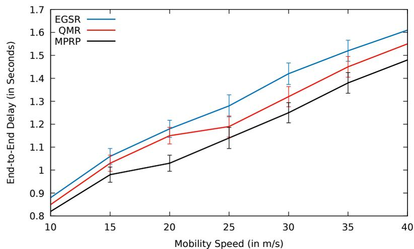
**Fig. 4.54:** Comparison between EGSR, QMR and proposed protocol MPRP for end-to-end delay including error bars with mobility speed.
