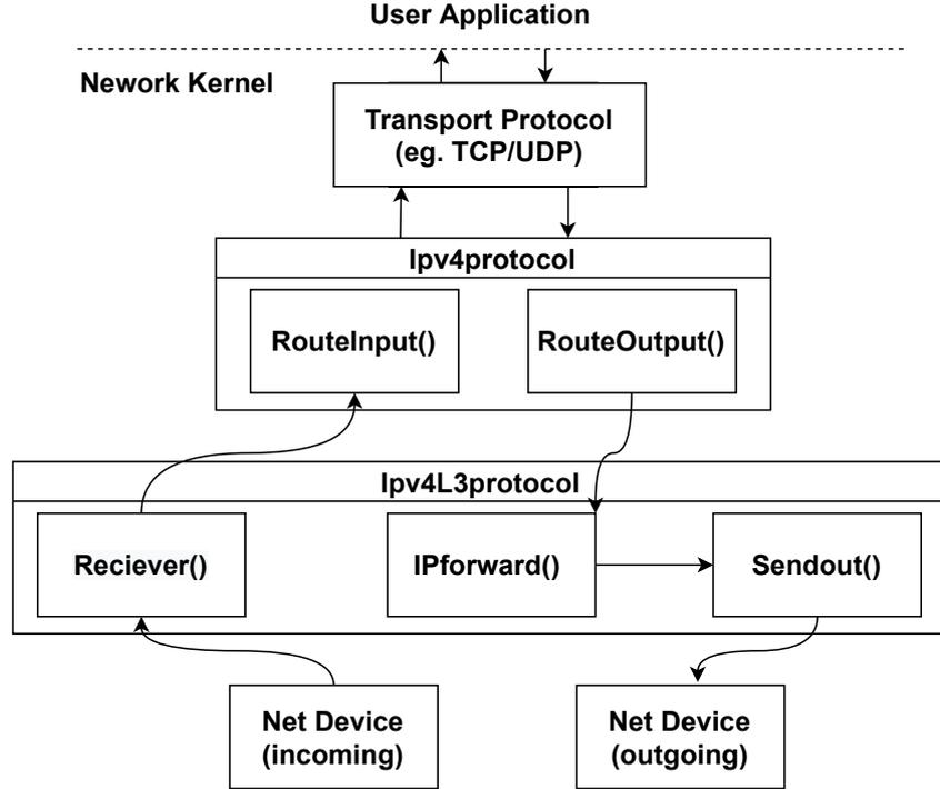
Fig. 3.1: hierarchy of packet processing in a network node.
