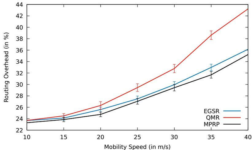
**Fig. 4.56:** Comparison between EGSR, QMR and proposed protocol MPRP for routing overhead including error bars with mobility speed.
