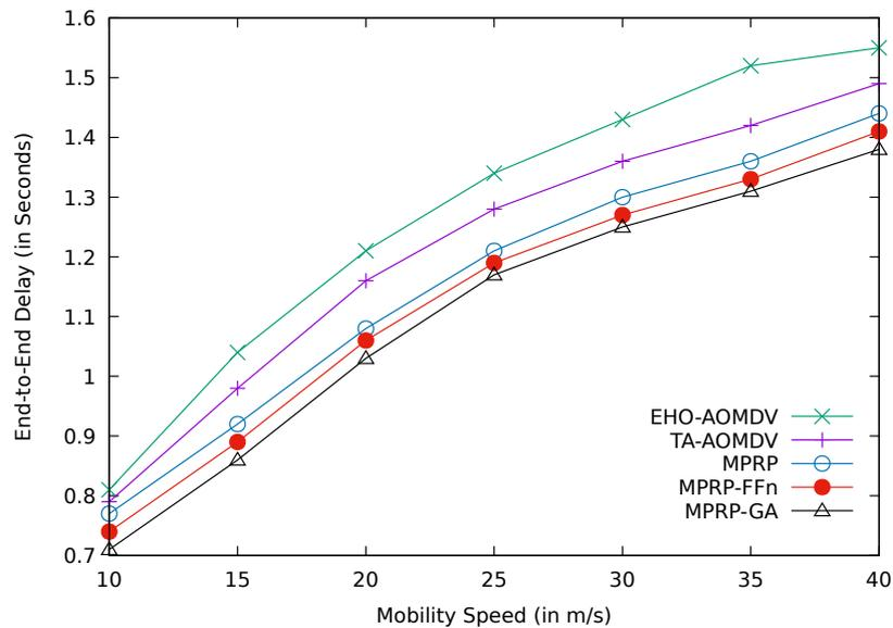
**Fig. 5.14:** Comparison between the proposed protocols of MPRP-GA and MPRP-FFn with MPRP, TA-AOMDV and EHO-AOMDV for average E2E over various mobility speeds.
