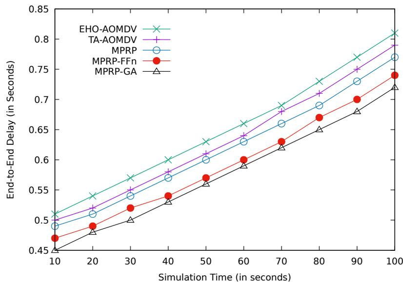
**Fig. 5.9:** Comparison between the proposed protocols of MPRP-GA and MPRP-FFn with MPRP, TA-AOMDV and EHO-AOMDV for average E2E over various simulation times.
