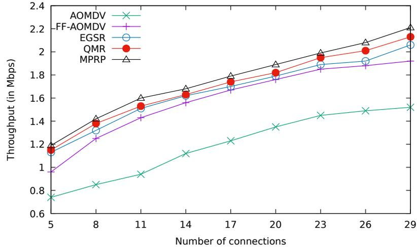
**Fig. 4.15:** Comparison between AOMDV, FF-AOMDV, EGSR, QMR and proposed protocol MPRP for throughput with different numbers of OBU nodes sending data to one RSU.
