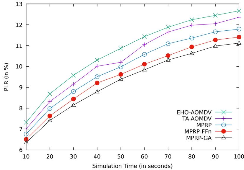
**Fig. 5.8:** Comparison between the proposed protocols of MPRP-GA and MPRP-FFn with MPRP, TA-AOMDV and EHO-AOMDV for PLR over various simulation times.
