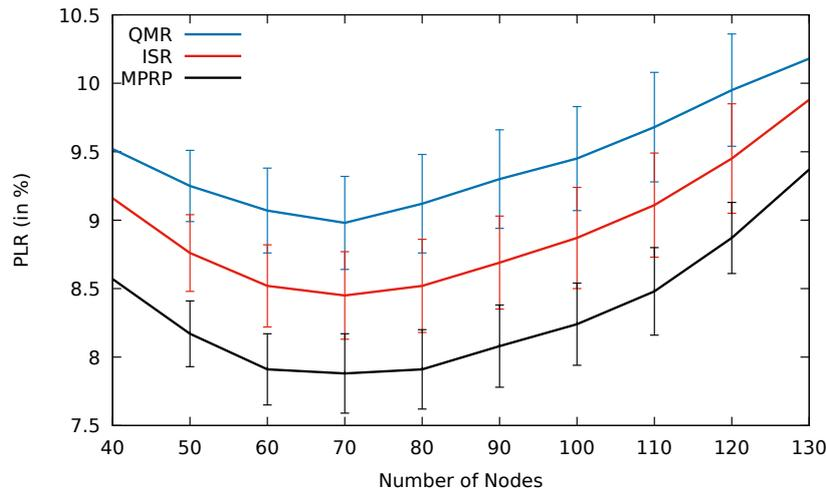
**Fig. 4.67:** Comparison between QMR, ISR and proposed protocol MPRP for PLR including error bars with number of nodes.
