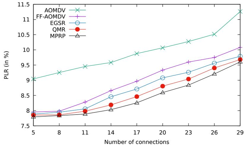
**Fig. 4.18:** Comparison between AOMDV, FF-AOMDV, EGSR, QMR and proposed protocol MPRP for PLR with different numbers of OBU nodes receiving data from one RSU.
