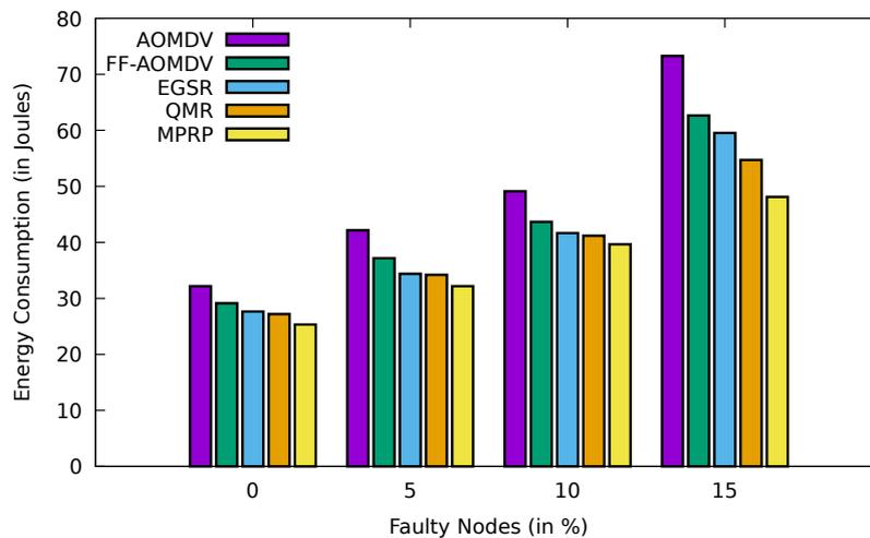
**Fig. 4.37:** Comparison between AOMDV, FF-AOMDV, EGSR, QMR and proposed protocol MPRP for energy consumption with faulty node.
