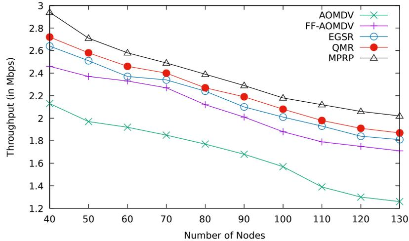
**Fig. 4.38:** Comparison between AOMDV, FF-AOMDV, EGSR, QMR and proposed protocol MPRP for throughput with number of nodes.
