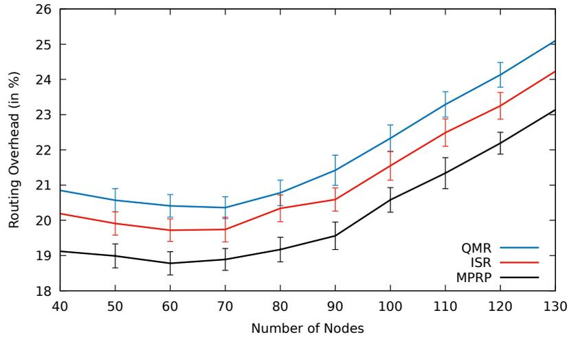
**Fig. 4.69:** Comparison between QMR, ISR and proposed protocol MPRP for routing overhead including error bars with number of nodes.
