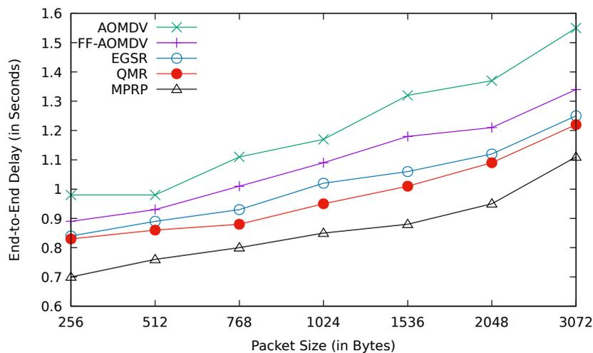
**Fig. 4.28:** Comparison between AOMDV, FF-AOMDV, EGSR, QMR and proposed protocol MPRP for end-to-end delay with different Packet sizes.
