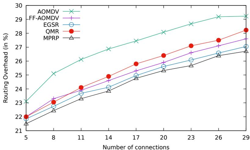
**Fig. 4.24:** Comparison between AOMDV, FF-AOMDV, EGSR, QMR and proposed protocol MPRP for routing overhead delay with different numbers of OBU nodes receiving data from one RSU
