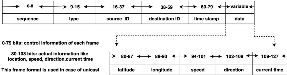
Fig. 4.4: Emergency packet format.
