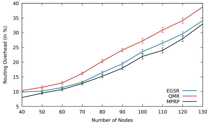
**Fig. 4.55:** Comparison between EGSR, QMR and proposed protocol MPRP for routing overhead including error bars with number of nodes.
