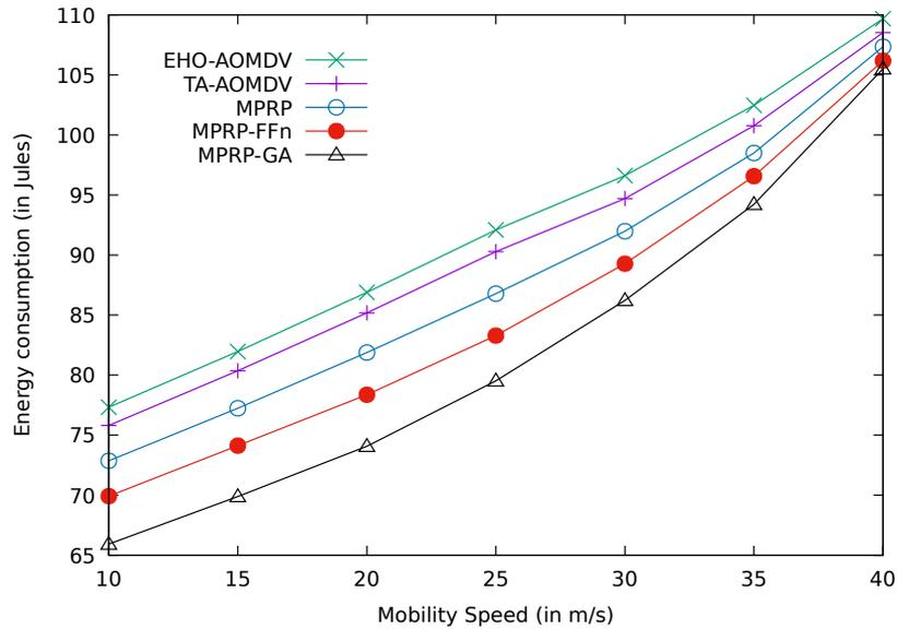
**Fig. 5.16:** Comparison between the proposed protocols of MPRP-GA and MPRP-FFn with MPRP, TA-AOMDV and EHO-AOMDV for energy consumption over various mobility speeds.
