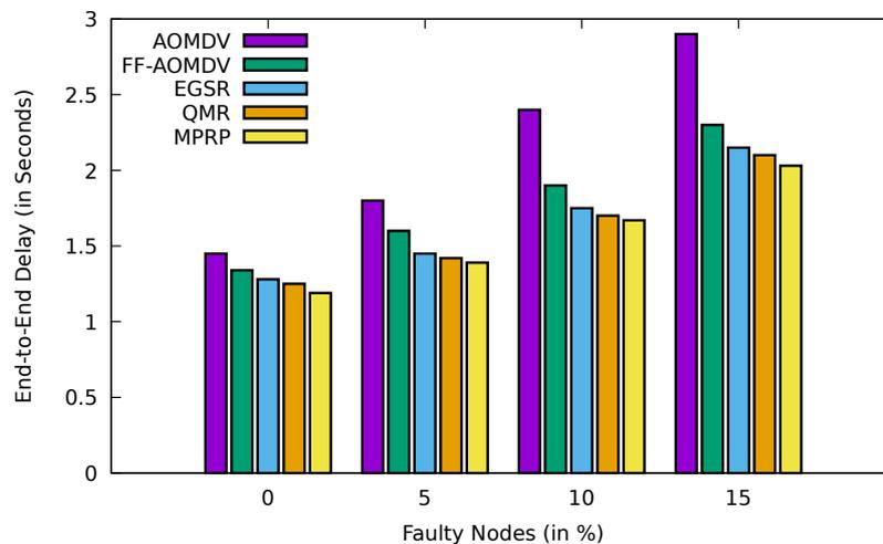
**Fig. 4.35:** Comparison between AOMDV, FF-AOMDV, EGSR, QMR and proposed protocol MPRP for end-to-end delay with faulty node.
