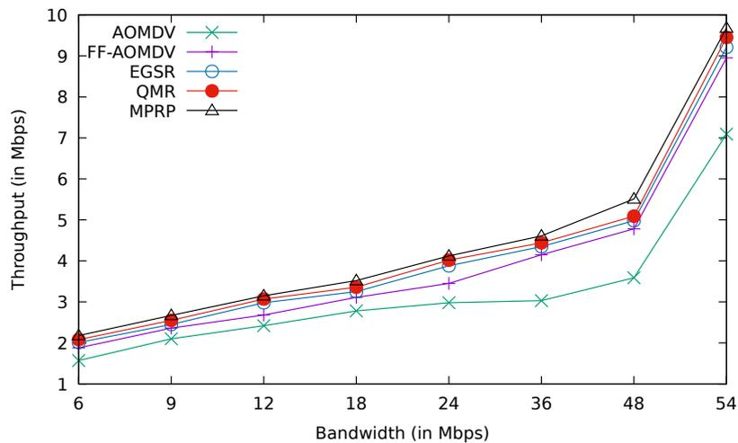
**Fig. 4.30:** Comparison between AOMDV, FF-AOMDV, EGSR, QMR and proposed protocol MPRP for throughput with bandwidth.
