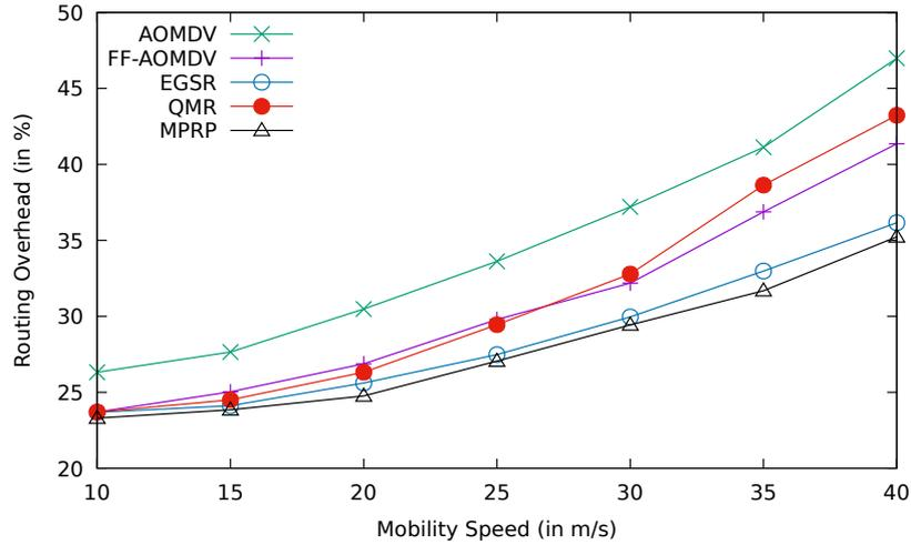
**Fig. 4.48:** Comparison between AOMDV, FF-AOMDV, EGSR, QMR and proposed protocol MPRP for routing overhead with mobility speed.
