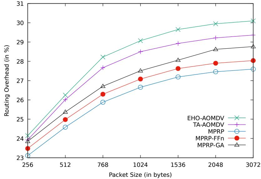
**Fig. 5.30:** Comparison between the proposed protocols of MPRP-GA and MPRP-FFn with MPRP, TA-AOMDV and EHO-AOMDV for routing overhead over various packet sizes.
