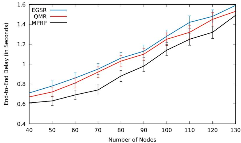
**Fig. 4.51:** Comparison between EGSR, QMR and proposed protocol MPRP for end-to-end delay including error bars with number of nodes.
