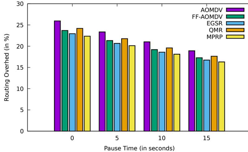
**Fig. 4.14:** Comparison between AOMDV, FF-AOMDV, EGSR, QMR and proposed protocol MPRP for routing overhead with pause time.
