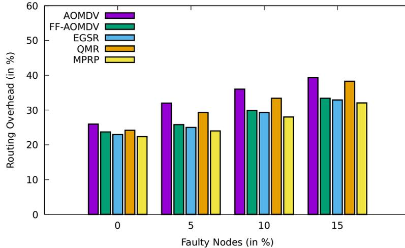
**Fig. 4.36:** Comparison between AOMDV, FF-AOMDV, EGSR, QMR and proposed protocol MPRP for routing overhead with faulty node.
