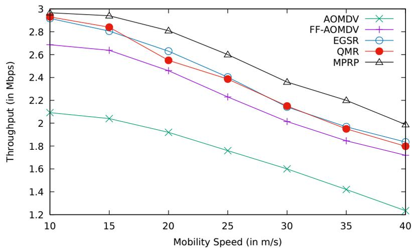
**Fig. 4.46:** Comparison between AOMDV, FF-AOMDV, EGSR, QMR and proposed protocol MPRP for throughput with mobility speed.
