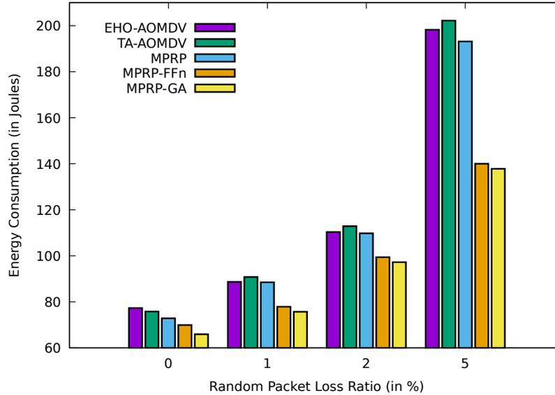
**Fig. 5.26:** Comparison between the proposed protocols of MPRP-GA and MPRP-FFn with MPRP, TA-AOMDV and EHO-AOMDV for energy consumption over various random loss ratio.
