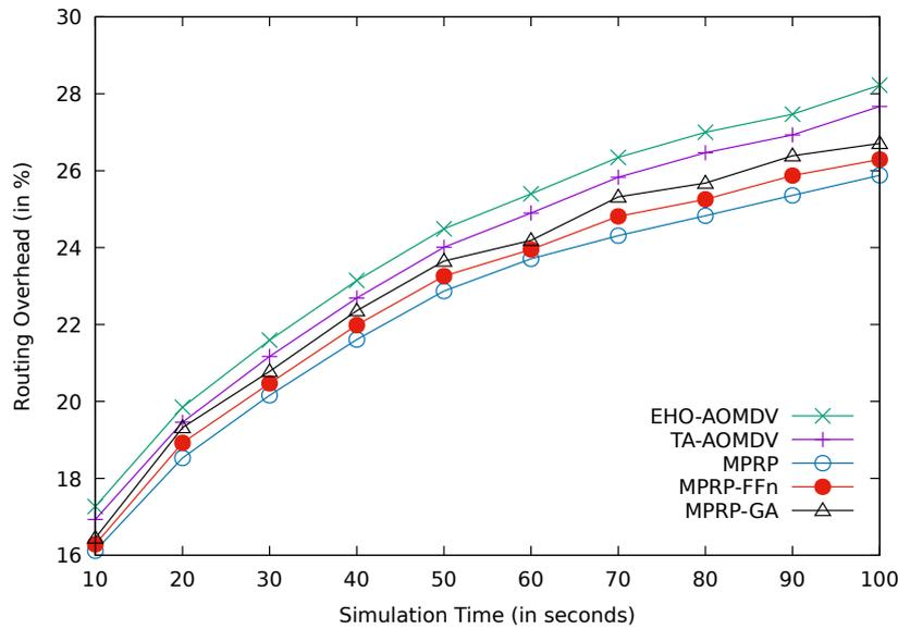
**Fig. 5.10:** Comparison between the proposed protocols of MPRP-GA and MPRP-FFn with MPRP, TA-AOMDV and EHO-AOMDV for routing overhead over various simulation times.
