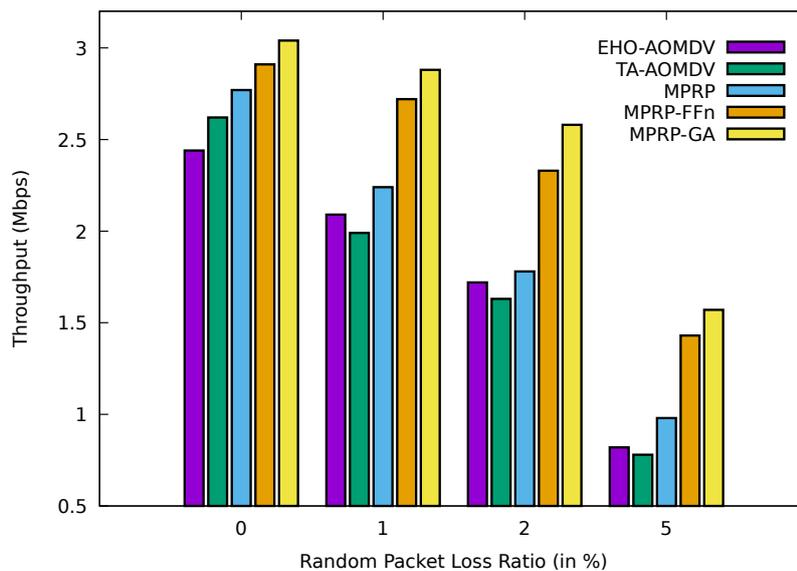
**Fig. 5.22:** Comparison between the proposed protocols of MPRP-GA and MPRP-FFn with MPRP, TA-AOMDV and EHO-AOMDV for throughput over various random loss ratio.
