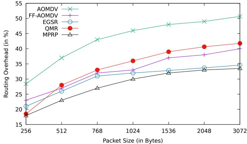
**Fig. 4.29:** Comparison between AOMDV, FF-AOMDV, EGSR, QMR and proposed protocol MPRP for routing overhead with different Packet sizes.
