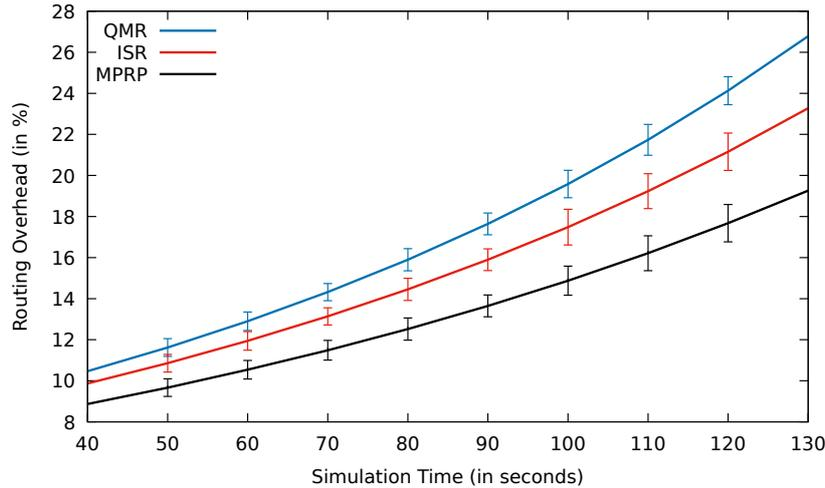
**Fig. 4.61:** Comparison between EGSR, ISR and proposed protocol MPRP for routing overhead including error bars with simulation time.
