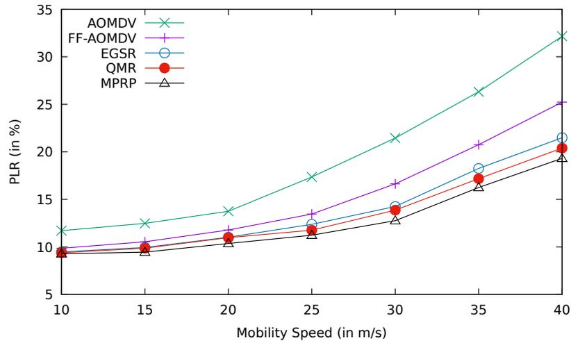
**Fig. 4.43:** Comparison between AOMDV, FF-AOMDV, EGSR, QMR and proposed protocol MPRP for PLR with mobility speed.
