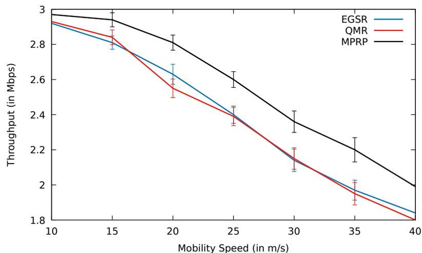
**Fig. 4.52:** Comparison between EGSR, QMR and proposed protocol MPRP for throughput including error bars with mobility speed.
