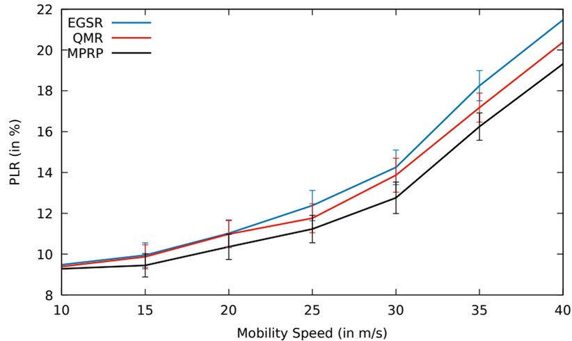
**Fig. 4.53:** Comparison between EGSR, QMR and proposed protocol MPRP for PLR including error bars with mobility speed.
