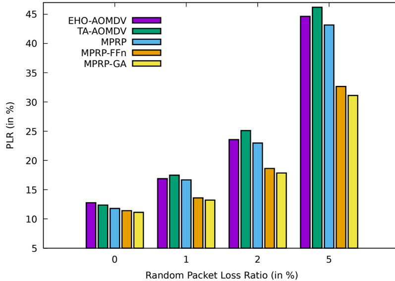
**Fig. 5.23:** Comparison between the proposed protocols of MPRP-GA and MPRP-FFn with MPRP, TA-AOMDV and EHO-AOMDV for PLR over various random loss ratio.
