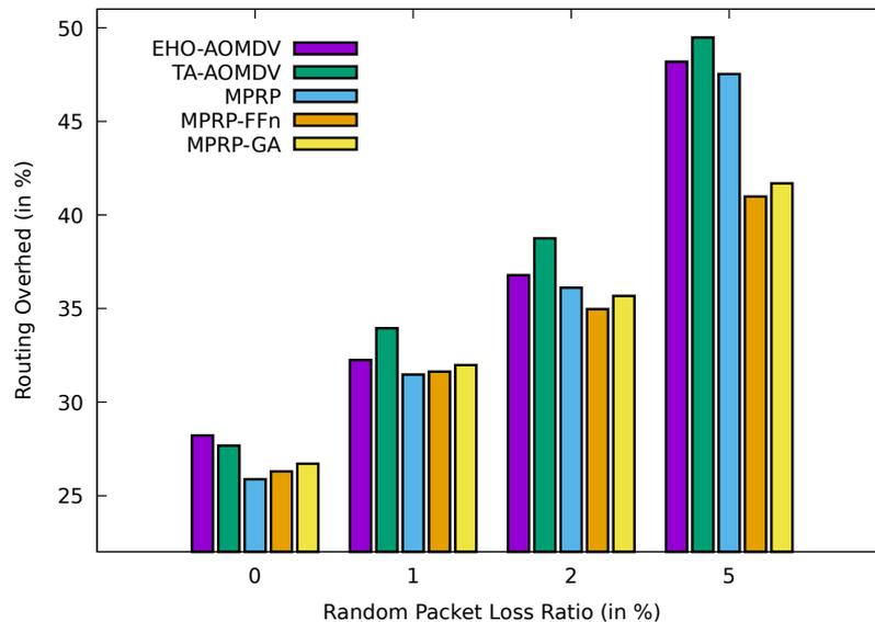
**Fig. 5.25:** Comparison between the proposed protocols of MPRP-GA and MPRP-FFn with MPRP, TA-AOMDV and EHO-AOMDV for routing overhead over various random loss ratio.
