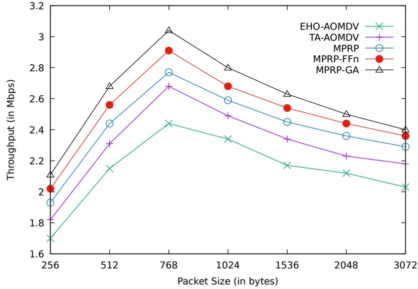
**Fig. 5.27:** Comparison between the proposed protocols of MPRP-GA and MPRP-FFn with MPRP, TA-AOMDV and EHO-AOMDV for throughput over various packet sizes.
