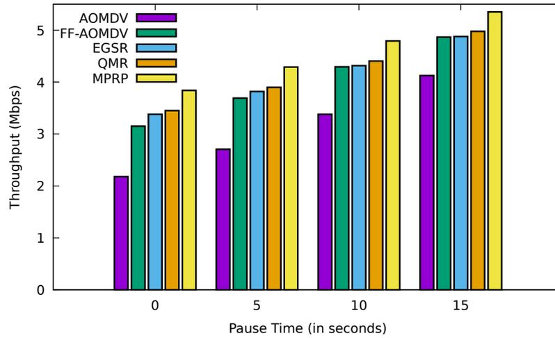
**Fig. 4.10:** Comparison between AOMDV, FF-AOMDV, EGSR, QMR and proposed protocol MPRP for throughput with pause time.
