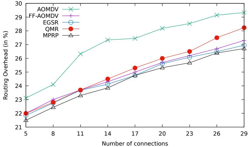
**Fig. 4.23:** Comparison between AOMDV, FF-AOMDV, EGSR, QMR and proposed protocol MPRP for routing overhead with different numbers of OBU nodes sending data to one RSU.
