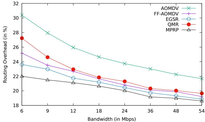
**Fig. 4.32:** Comparison between AOMDV, FF-AOMDV, EGSR, QMR and proposed protocol MPRP for routing overhead with band width.
