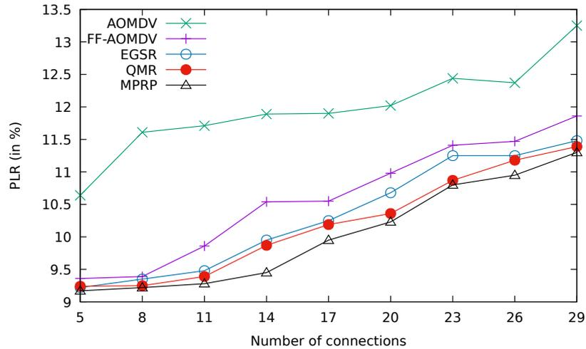
**Fig. 4.17:** Comparison between AOMDV, FF-AOMDV, EGSR, QMR and proposed protocol MPRP for PLR with different numbers of OBU nodes sending data to one RSU.
