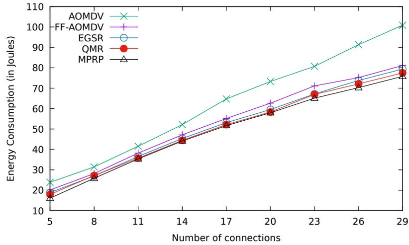
**Fig. 4.19:** Comparison between AOMDV, FF-AOMDV, EGSR, QMR and proposed protocol MPRP for energy consumption with different numbers of OBU nodes sending data to one RSU.
