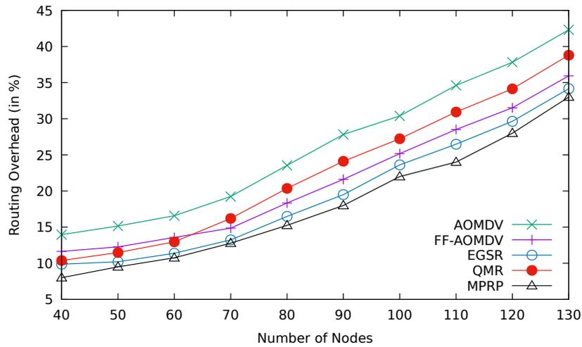
**Fig. 4.47:** Comparison between AOMDV, FF-AOMDV, EGSR, QMR and proposed protocol MPRP for routing overhead with mobility speed.
