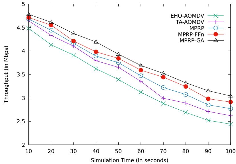
**Fig. 5.7:** Comparison between the proposed protocols of MPRP-GA and MPRP-FFn with MPRP, TA-AOMDV and EHO-AOMDV for throughput over various simulation times.
