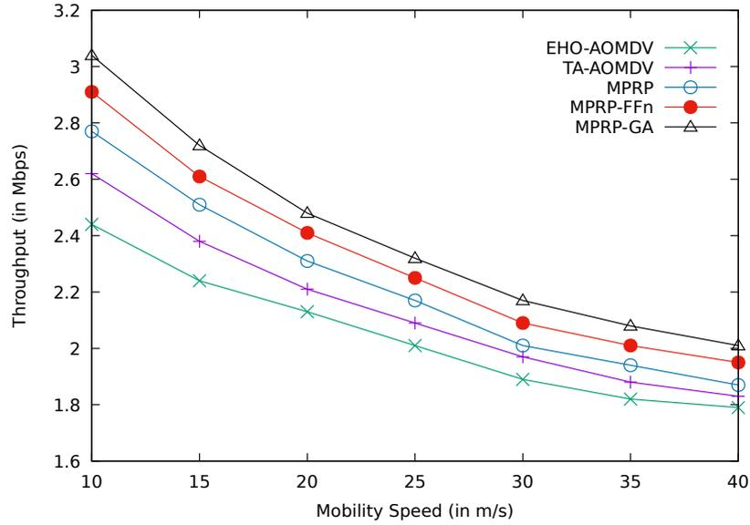
**Fig. 5.12:** Comparison between the proposed protocols of MPRP-GA and MPRP-FFn with MPRP, TA-AOMDV and EHO-AOMDV for throughput over various mobility speeds.
