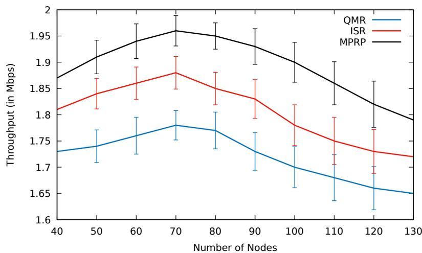
**Fig. 4.66:** Comparison between QMR, ISR and proposed protocol MPRP for throughput including error bars with number of nodes.
