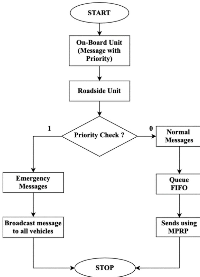
**Fig. 4.2:** Flow diagram of message handling.
