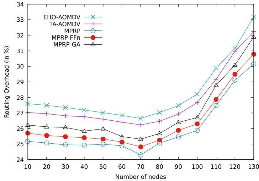
**Fig. 5.20:** Comparison between the proposed protocols of MPRP-GA and MPRP-FFn with MPRP, TA-AOMDV and EHO-AOMDV for routing overhead over various number of nodes.
