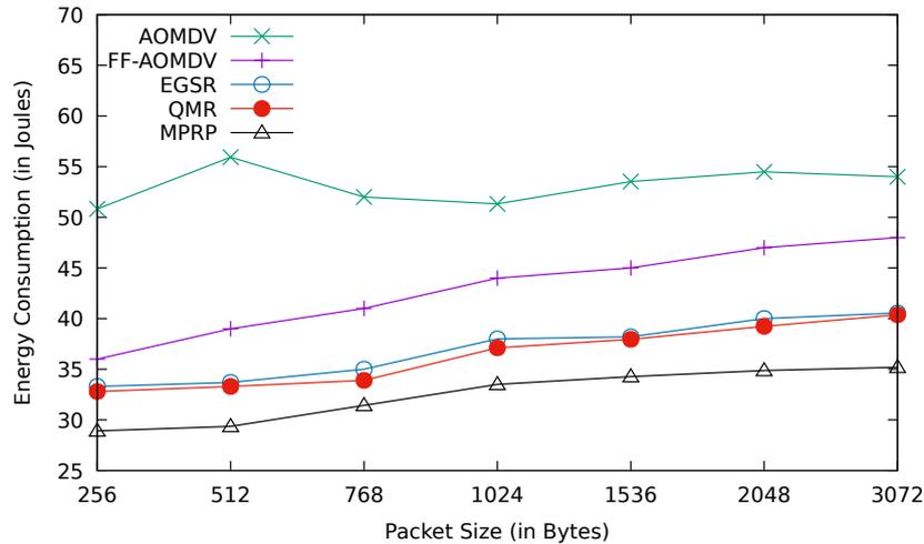
**Fig. 4.27:** Comparison between AOMDV, FF-AOMDV, EGSR, QMR and proposed protocol MPRP for energy consumption with different Packet sizes.
