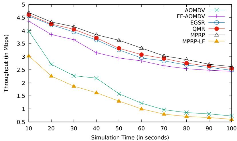
Fig. 4.6: Comparison between AOMDV, FF-AOMDV, EGSR, QMR and proposed protocol MPRP and MPRP-LF for throughput with simulation time.
