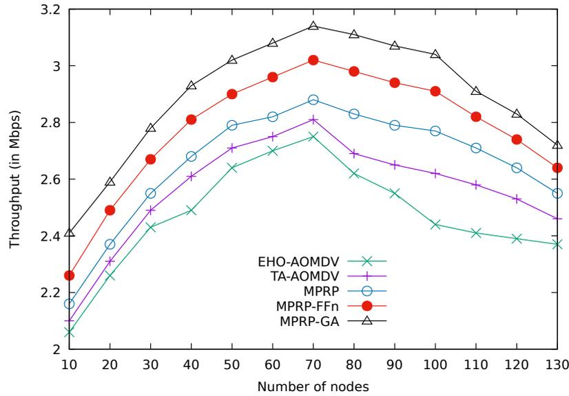
**Fig. 5.17:** Comparison between the proposed protocols of MPRP-GA and MPRP-FFn with MPRP, TA-AOMDV and EHO-AOMDV for throughput over various number of nodes.
