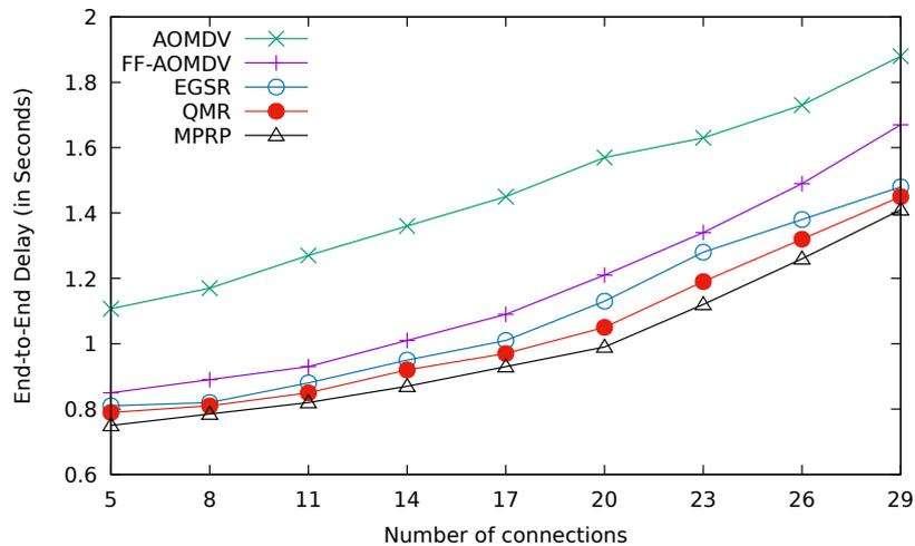
**Fig. 4.22:** Comparison between AOMDV, FF-AOMDV, EGSR, QMR and proposed protocol MPRP for end-to-end delay with different numbers of OBU nodes receiving data from one RSU.
