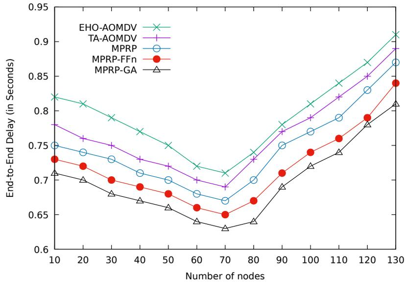
**Fig. 5.19:** Comparison between the proposed protocols of MPRP-GA and MPRP-FFn with MPRP, TA-AOMDV and EHO-AOMDV for average E2E over various number of nodes.
