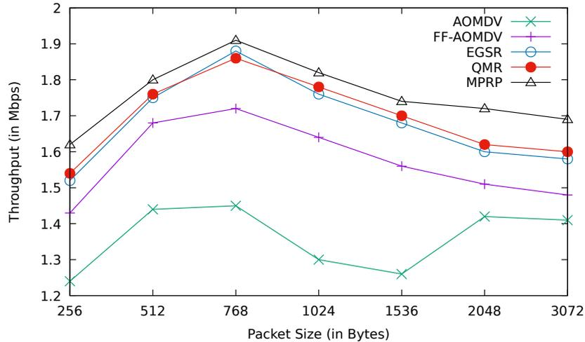
**Fig. 4.25:** Comparison between AOMDV, FF-AOMDV, EGSR, QMR and proposed protocol MPRP for throughput with different Packet sizes.
