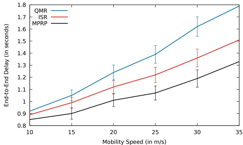
**Fig. 4.64:** Comparison between QMR, ISR and proposed protocol MPRP for end-to-end delay including error bars with mobility speed.
