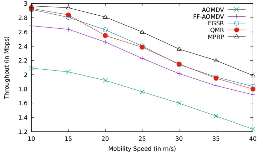
**Fig. 4.42:** Comparison between AOMDV, FF-AOMDV, EGSR, QMR and proposed protocol MPRP for throughput with mobility speed.
