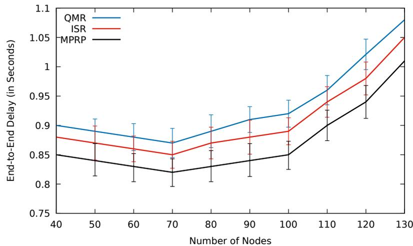
**Fig. 4.68:** Comparison between QMR, ISR and proposed protocol MPRP for end-to-end delay including error bars with number of nodes.
