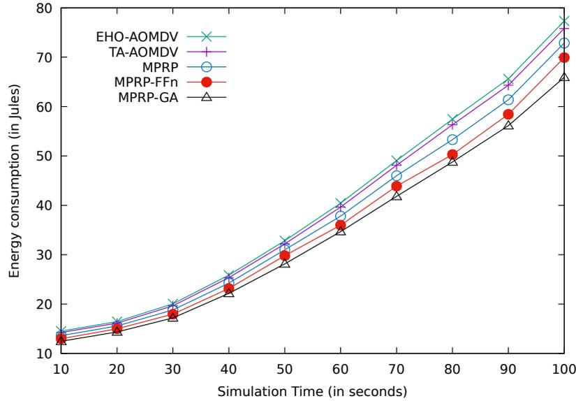
**Fig. 5.11:** Comparison between the proposed protocols of MPRP-GA and MPRP-FFn with MPRP, TA-AOMDV and EHO-AOMDV for energy consumption over various simulation times.
