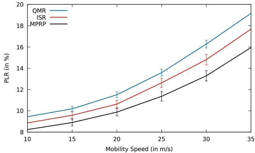
**Fig. 4.63:** Comparison between QMR, ISR and proposed protocol MPRP for PLR including error bars with mobility speed.
