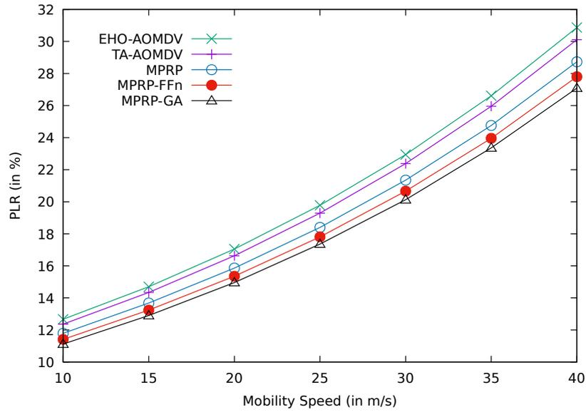
**Fig. 5.13:** Comparison between the proposed protocols of MPRP-GA and MPRP-FFn with MPRP, TA-AOMDV and EHO-AOMDV for PLR over various mobility speeds.
