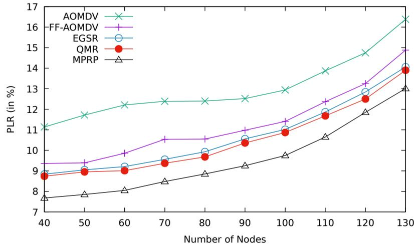
**Fig. 4.39:** Comparison between AOMDV, FF-AOMDV, EGSR, QMR and proposed protocol MPRP for PLR with number of nodes.
