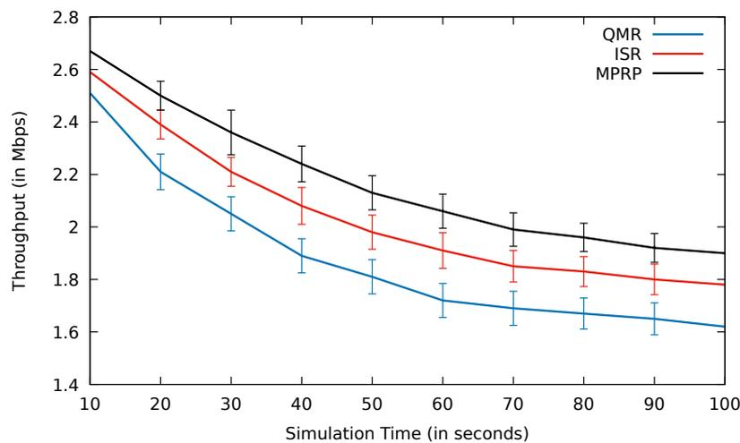
Fig. 4.58: Comparison between EGSR, ISR and proposed protocol MPRP for throughput including error bars with simulation time.
