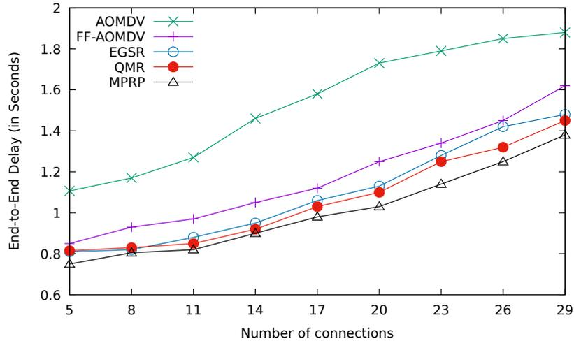
**Fig. 4.21:** Comparison between AOMDV, FF-AOMDV, EGSR, QMR and proposed protocol MPRP for end-to-end delay with different numbers of OBU nodes sending data to one RSU.
