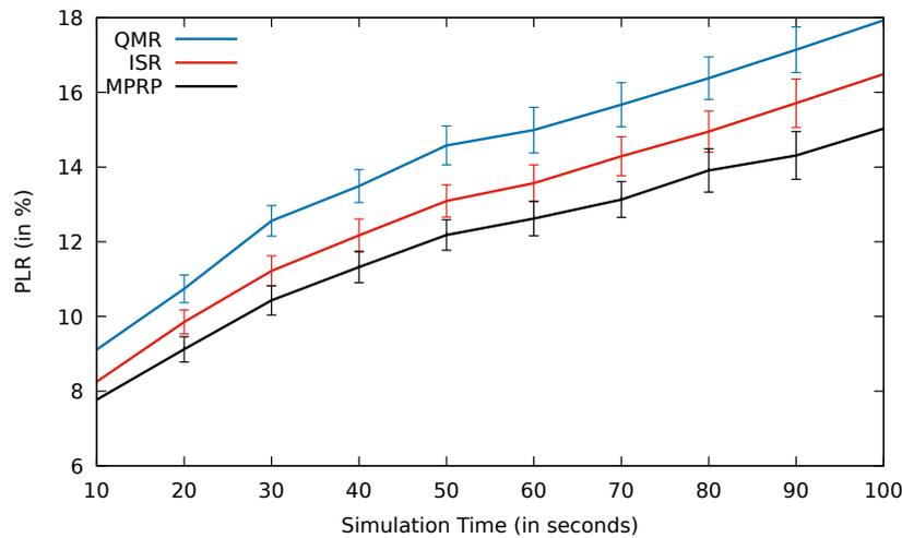
**Fig. 4.59:** Comparison between EGSR, ISR and proposed protocol MPRP for PLR including error bars with simulation time.
