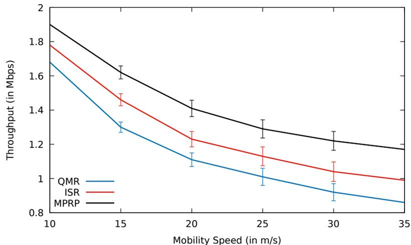
**Fig. 4.62:** Comparison between QMR, ISR and proposed protocol MPRP for throughput including error bars with mobility speed.
