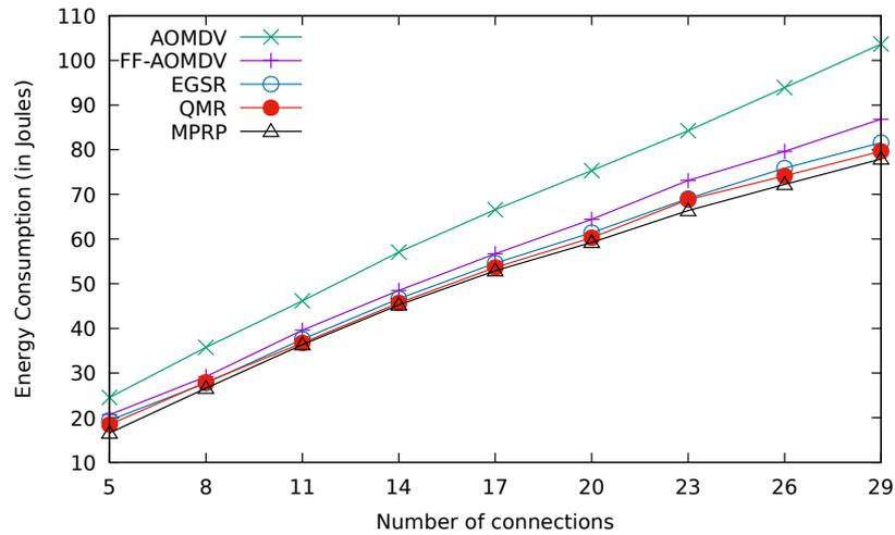
**Fig. 4.20:** Comparison between AOMDV, FF-AOMDV, EGSR, QMR and proposed protocol MPRP for energy consumption with different numbers of OBU nodes receiving data from one RSU.
