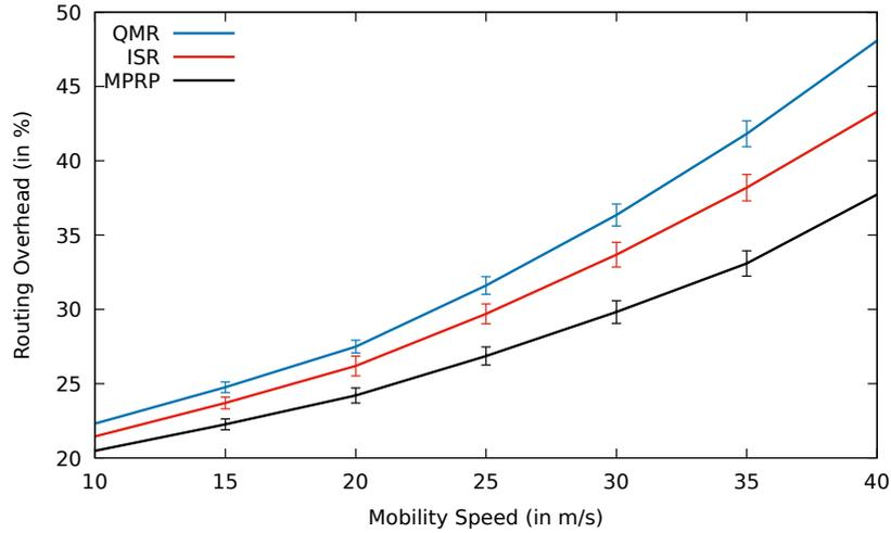
**Fig. 4.65:** Comparison between QMR, ISR and proposed protocol MPRP for routing overhead including error bars with mobility speed.
