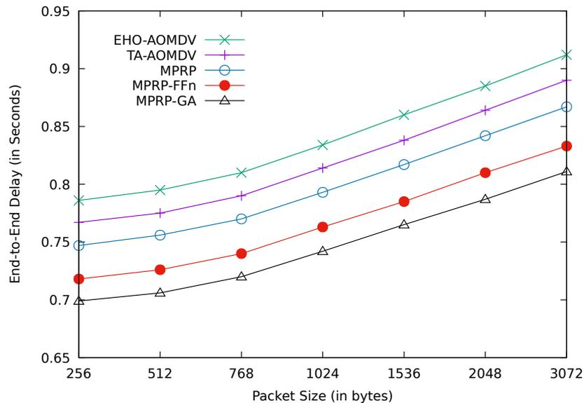
**Fig. 5.29:** Comparison between the proposed protocols of MPRP-GA and MPRP-FFn with MPRP, TA-AOMDV and EHO-AOMDV for average E2E over various packet sizes.
