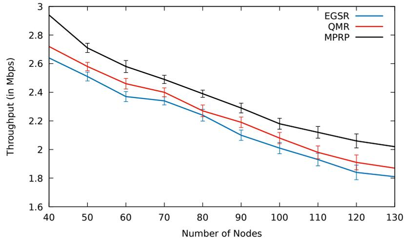
**Fig. 4.49:** Comparison between EGSR, QMR and proposed protocol MPRP for throughput including error bars with number of nodes.
