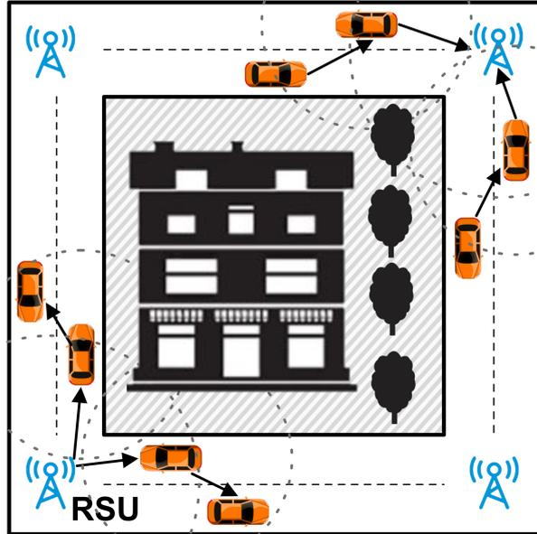
Fig. 4.5: Scenario 1: data communications in one road segment.
