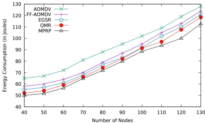
**Fig. 4.41:** Comparison between AOMDV, FF-AOMDV, EGSR, QMR and proposed protocol MPRP for energy consumption with number of nodes.
