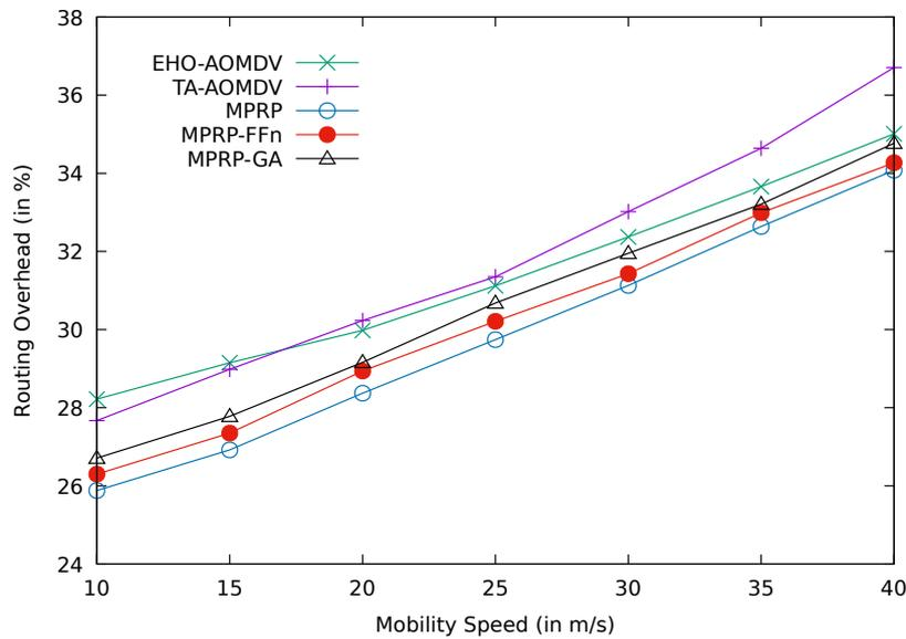
**Fig. 5.15:** Comparison between the proposed protocols of MPRP-GA and MPRP-FFn with MPRP, TA-AOMDV and EHO-AOMDV for routing overhead over various mobility speeds.
