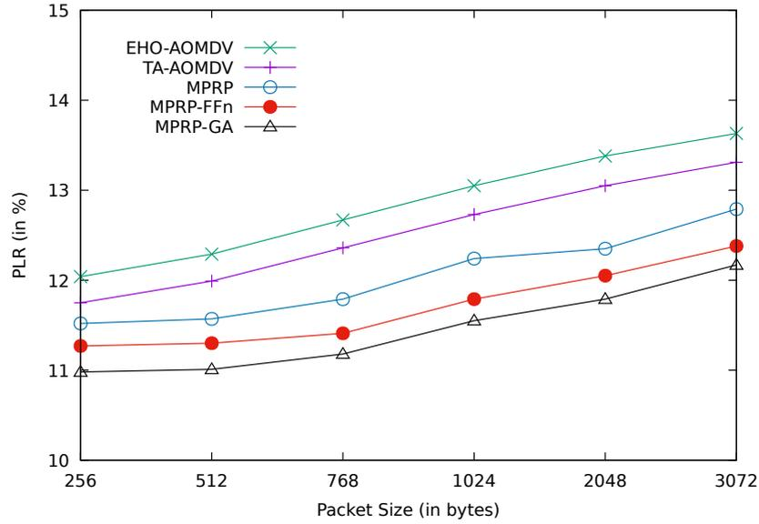
**Fig. 5.28:** Comparison between the proposed protocols of MPRP-GA and MPRP-FFn with MPRP, TA-AOMDV and EHO-AOMDV for PLR over various packet sizes.
