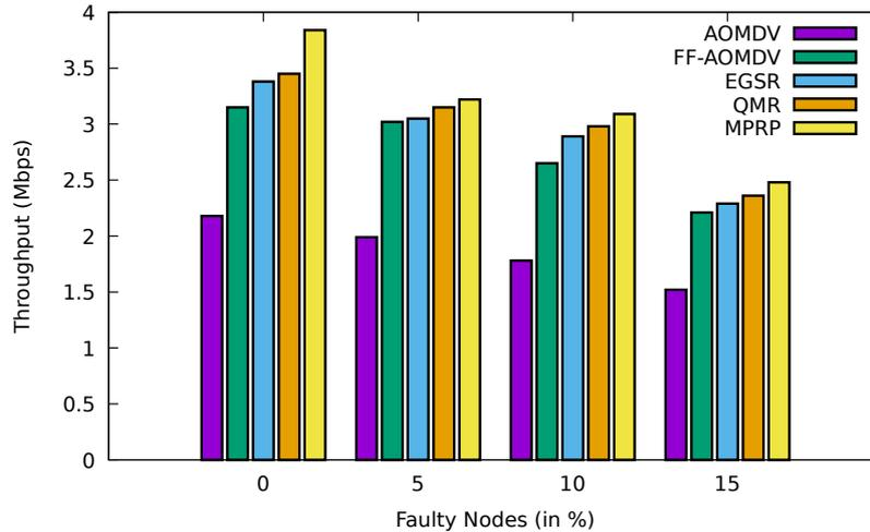
**Fig. 4.33:** Comparison between AOMDV, FF-AOMDV, EGSR, QMR and proposed protocol MPRP for throughput with faulty node.
