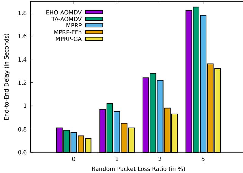
**Fig. 5.24:** Comparison between the proposed protocols of MPRP-GA and MPRP-FFn with MPRP, TA-AOMDV and EHO-AOMDV for average E2E over various random loss ratio.
