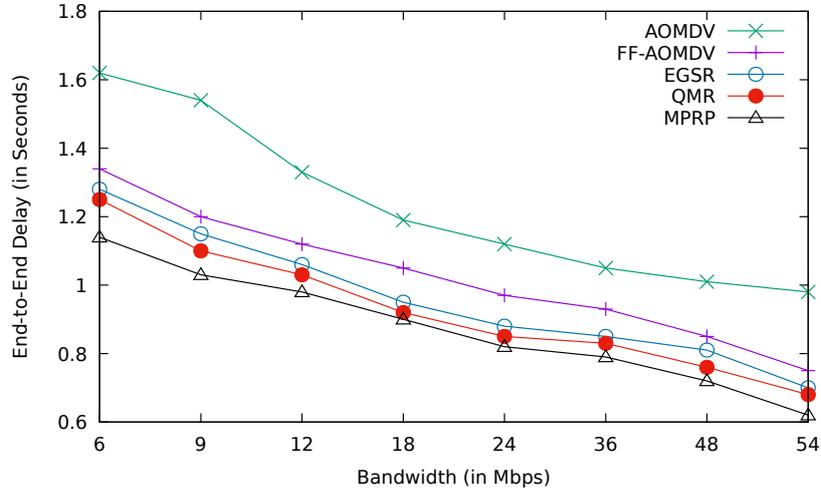
**Fig. 4.31:** Comparison between AOMDV, FF-AOMDV, EGSR, QMR and proposed protocol MPRP for end-to-end delay with bandwidth.
