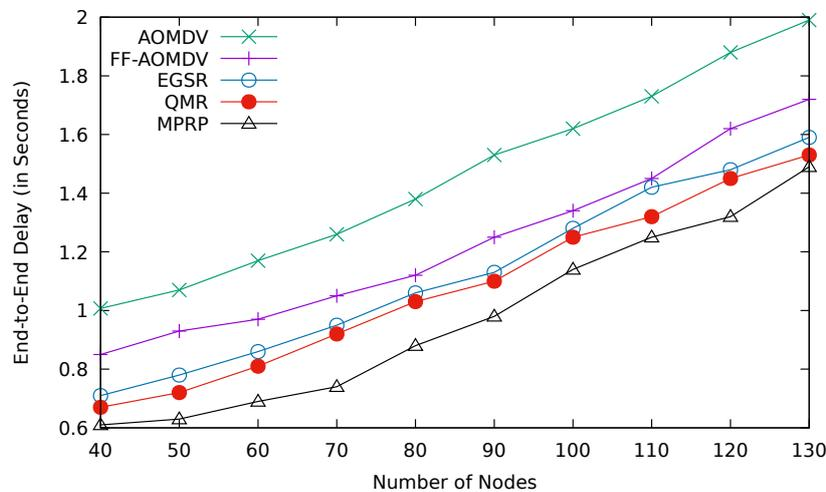
**Fig. 4.40:** Comparison between AOMDV, FF-AOMDV, EGSR, QMR and proposed protocol MPRP for end-to-end delay with number of nodes.
