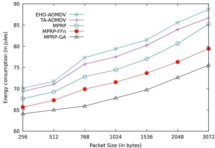
**Fig. 5.31:** Comparison between the proposed protocols of MPRP-GA and MPRP-FFn with MPRP, TA-AOMDV and EHO-AOMDV for energy consumption over various packet sizes.
