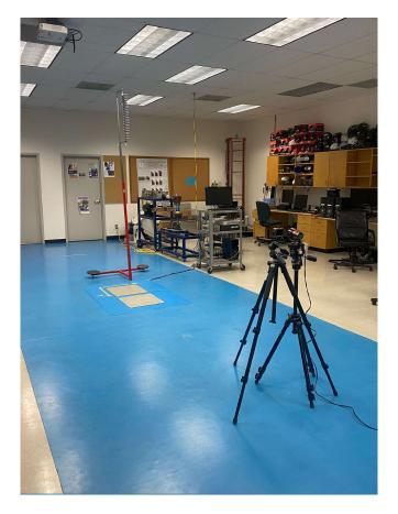
*Note*. The GoPro© camera and Vertec<sup>TM</sup> set-up for the vertical jump test surrounding the AMTI© force platform.
