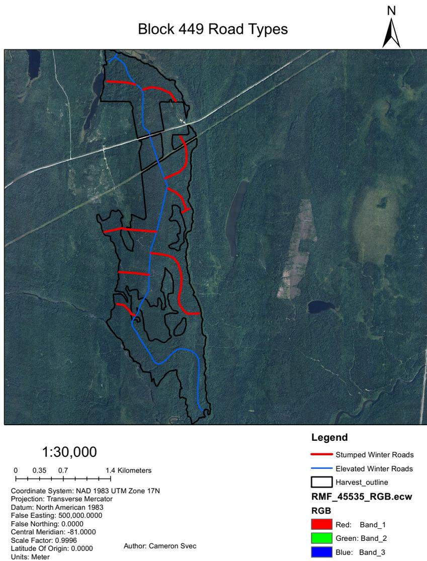
Figure 21. Road network construction method for scenario one on block 449
