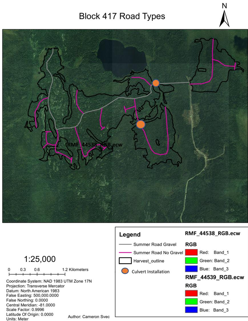
Figure 19. Road network construction methods for scenario two on block 417
