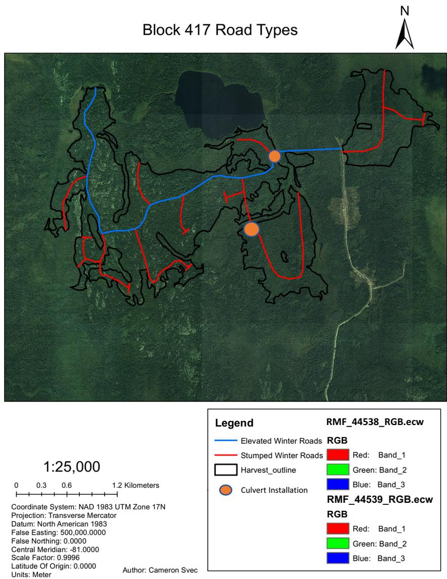
Figure 18. Road network construction method for scenario one on block 417
