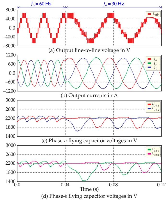
Figure 2.10. Step response with change in output frequency ( $m_a = 0.9$  and PF = 0.80 (lag)).
