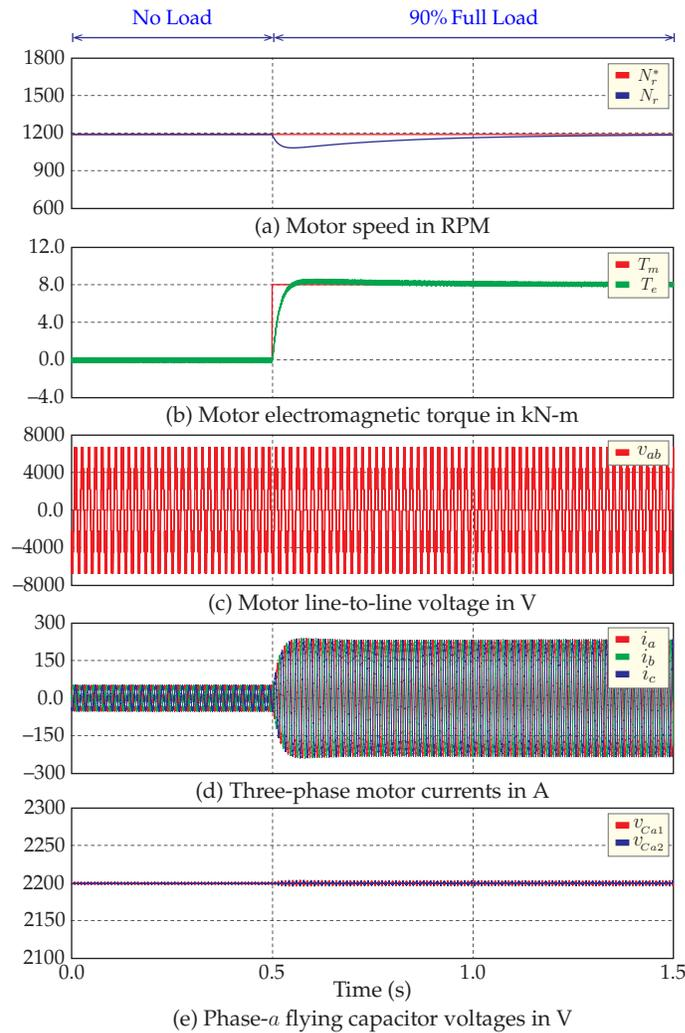
Figure 3.8. Transient performance of the proposed MV drive.
