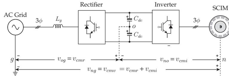
Figure 1.3. Common mode voltage in MV drive.
