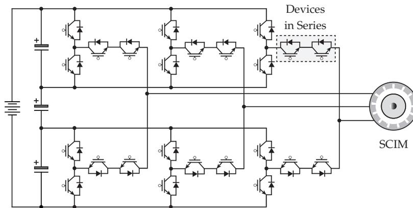
Figure 1.10. Four-level HANPC converter fed MV drive.
