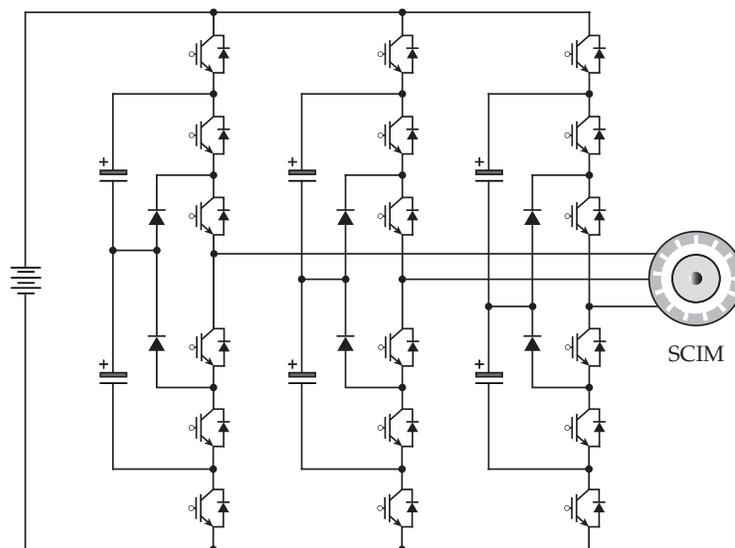
Figure 1.9. Four-level NNPC converter fed MV drive.
