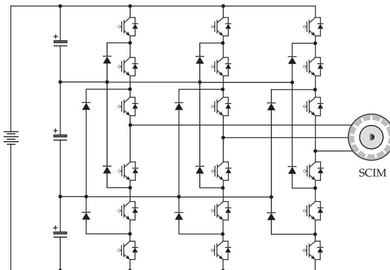
Figure 1.6. Four-level DCC fed MV drive.
