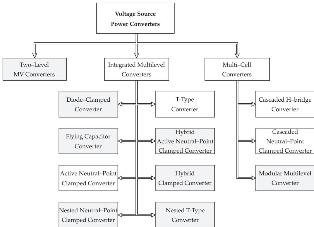
Figure 1.4. Classification of voltage source power converters for MV drives.
