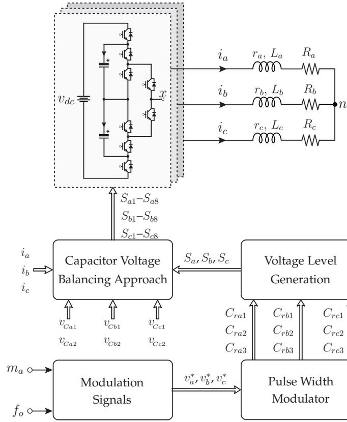
Figure 2.5. Control block diagram of the proposed 4L-MLC.
