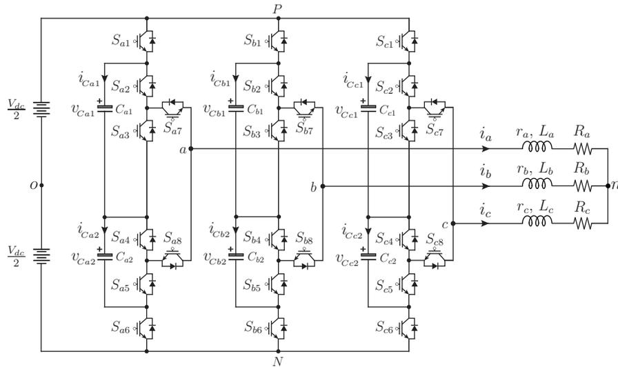
Figure 2.1. Proposed 4L-MLC with a passive load.
