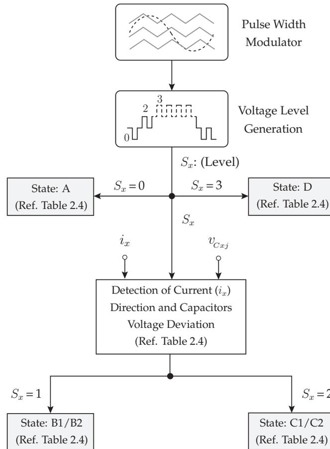
Figure 2.7. Implementation of the proposed voltage balancing approach.
