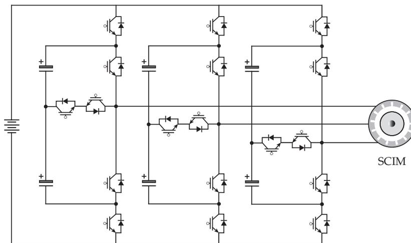
Figure 1.12. Four-level nested T-type converter fed MV drive.
