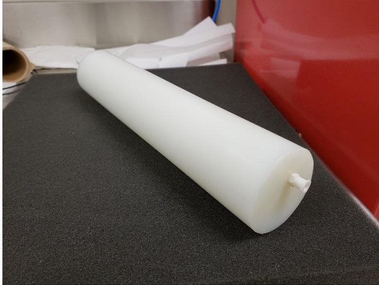
Fig. 9: Scatter phantom which is used in the determination of system count rates.
