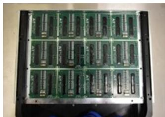
Fig. 14: Top view of 3×4 array of sensor modules inside a detector head.
