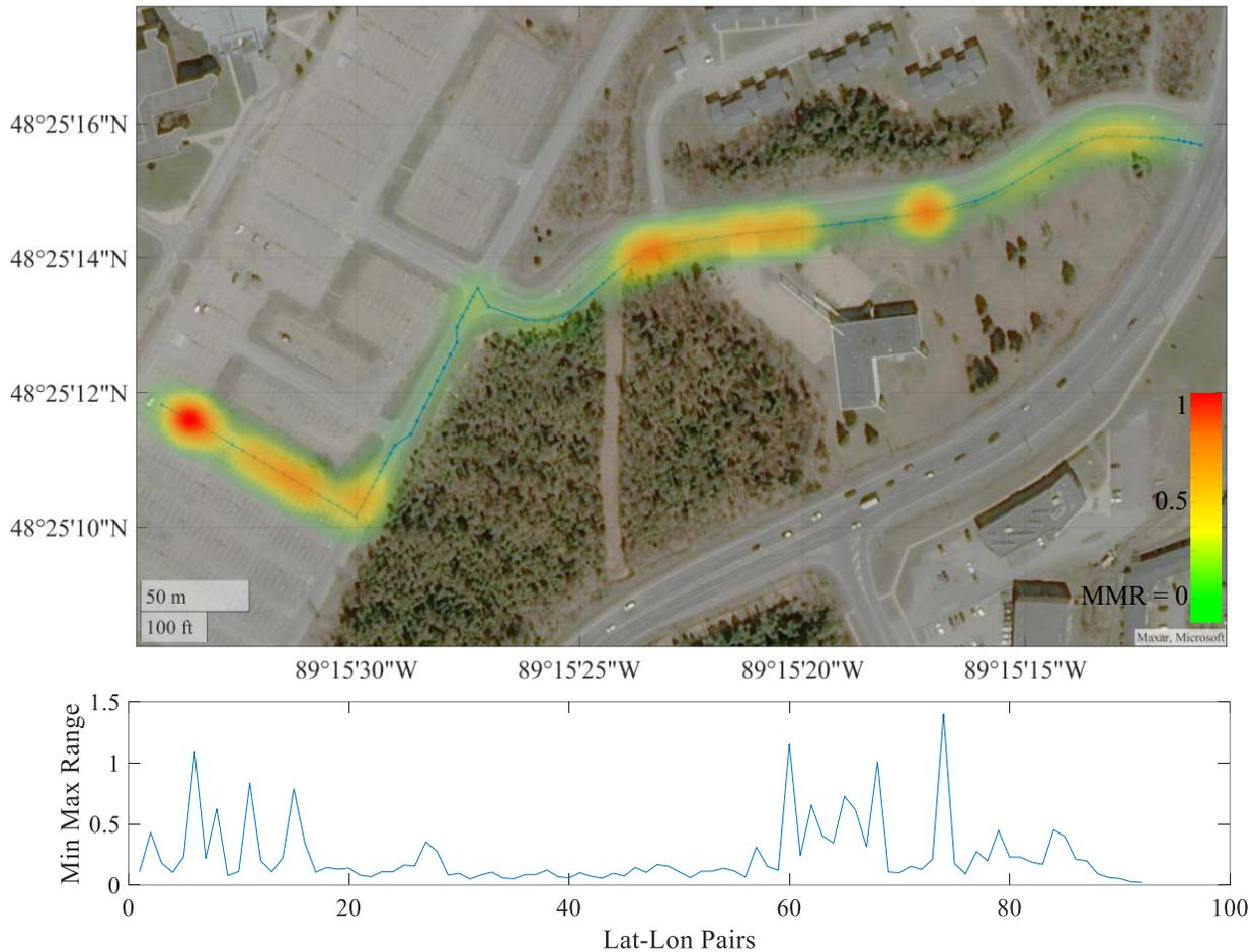
**Figure 26. A geographic density plot using the MMR roughness metric**
