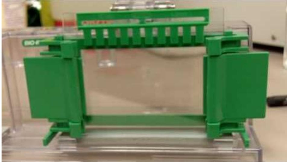
Figure 3.3: Assembled SDS-PAGE gel for Western blotting
