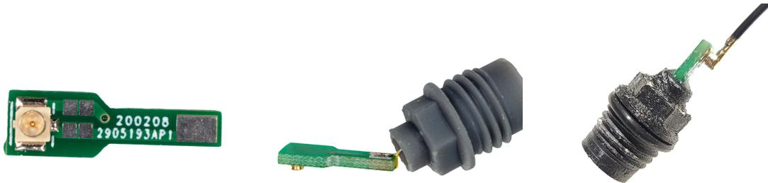
Figure 3.13: Picture of PCB mounted in casing.
