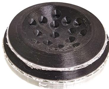
Figure 3.16: Picture of FDM printed polycarbonate shell before post-processing.
