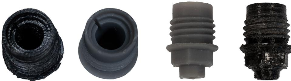
Figure 3.11: Picture of Tx casings, where the black casings on the far left and right are polycarbonate.
