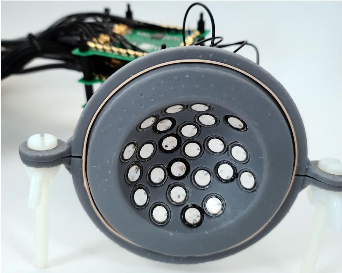
Figure 3.10: Picture of assembled array shell and Txs.
