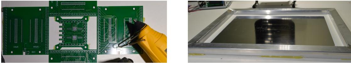
Figure 3.23: Positioning stencil for solder paste on driver PCB.
