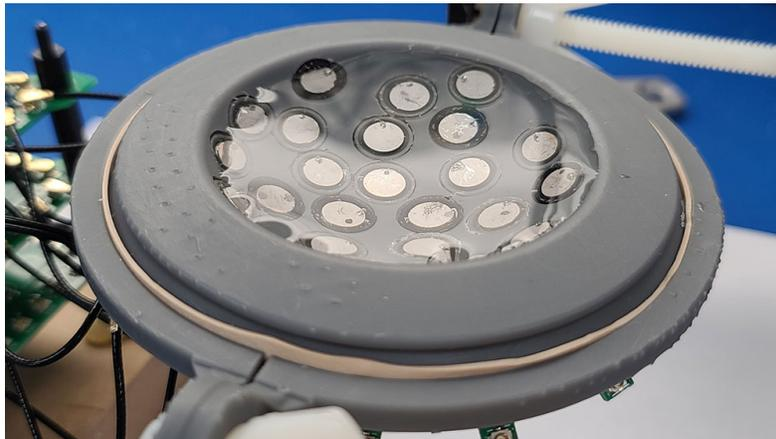
Figure 3.14: Picture of assembled array shell and Tx's.
