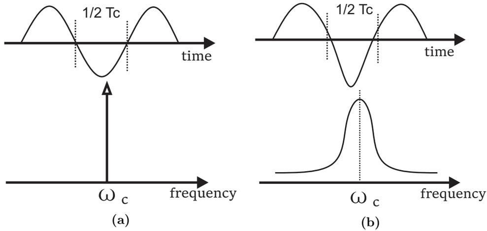
**Figure 2.2:** (a)Noiseless signal, (b)Noisy signal
