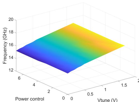
(b) Frequency versus  $V_{tune}$  versus power control setting
