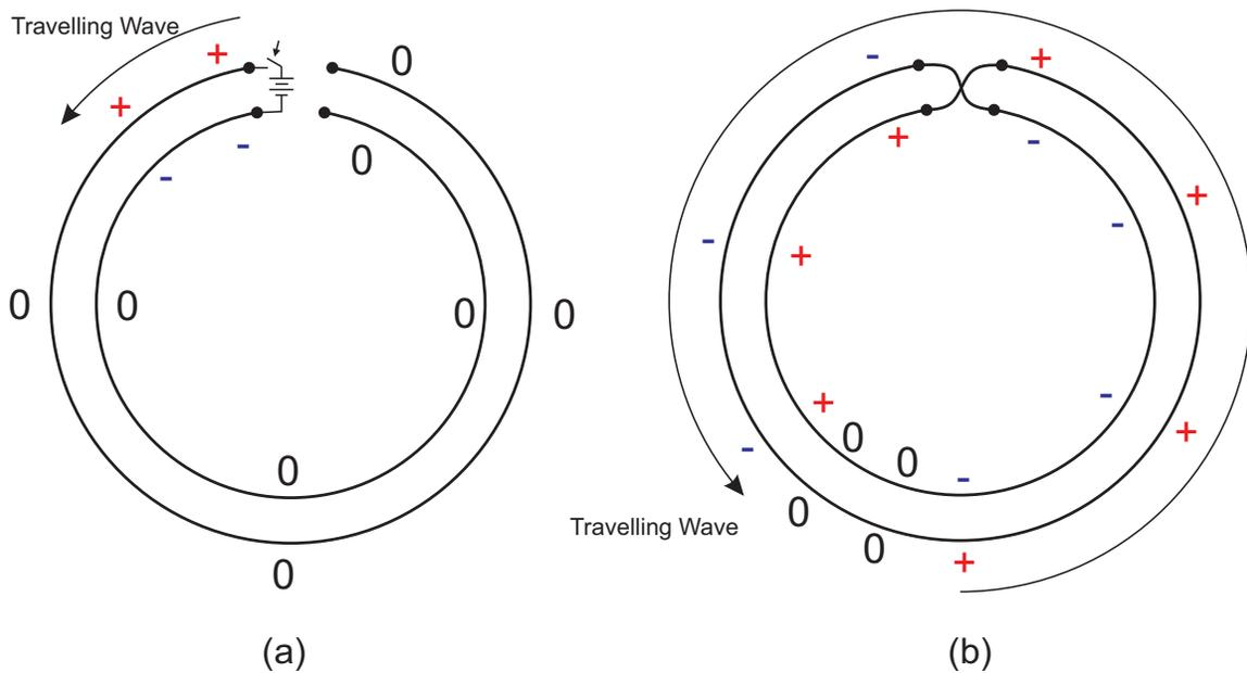
**Figure 2.11:** (a) An open loop differential TL gets energy from a battery via a switch, (b) The open circuit been replaced by a cross-connection
