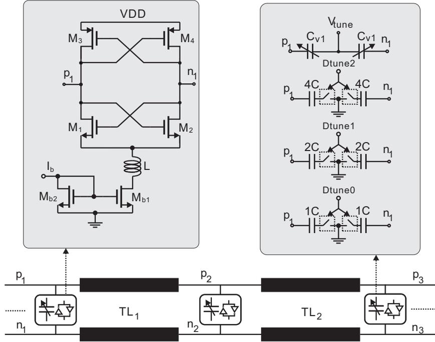
**Figure 4.4:** RTWO(a) with current drive latches.  $M_{1,2} = 12 \text{ fingers} \cdot 1.2 \mu\text{m}/130\text{nm}$ ,  $M_{3,4} = 12 \text{ fingers} \cdot 2.4 \mu\text{m}/130\text{nm}$ ,  $L = 900\text{pH}$ ,  $M_{b1,b2} = 32 \text{ fingers} \cdot 16 \mu\text{m}/260\text{nm}$ ,  $V_{\text{tune}} = 0$  to  $1.2$  V,  $C_{v1} = 13\text{fF}$  to  $41\text{fF}$ ,  $C = 26\text{fF}$ ,  $I_b = 1.5\text{mA}$  to  $3.5\text{mA}$
