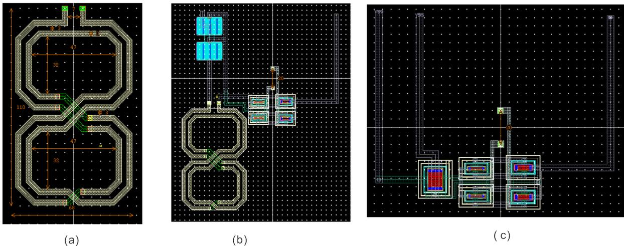
**Figure 4.15:** (a) Layout of the inductor, (b) Layout of amplifier latch and tail current source with filter RTWO design, and (c) Layout of voltage-mode latch in RTWO design.
