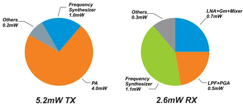
Figure 1.3: Measured power consumption in RF transceiver[1]
