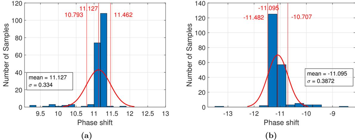
**Figure 3.15:** Two hundred points Monte Carlo simulations for both directions control. (a) Clockwise control, and (b) Counterclockwise control
