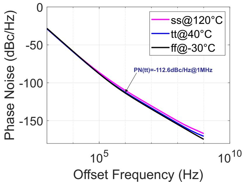
Figure 4.22: RTWO(b) PN across three corners at 13.75-GHz with 18-mW power
