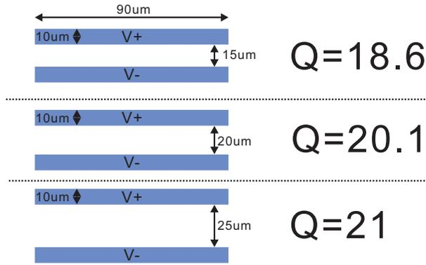
**Figure 3.7:** Compare the couple TLs with different gapping distance
