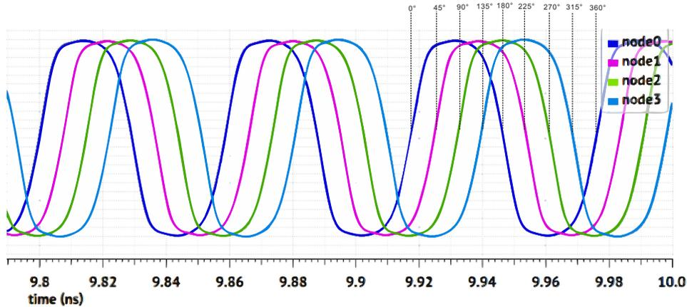
**Figure 2.12:** Time domain waveform of a 4-nodes RTWO.
