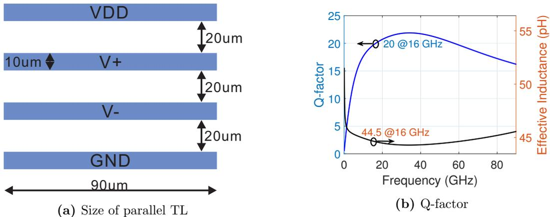
**Figure 3.5:** Size of parallel lines and Quality factor
