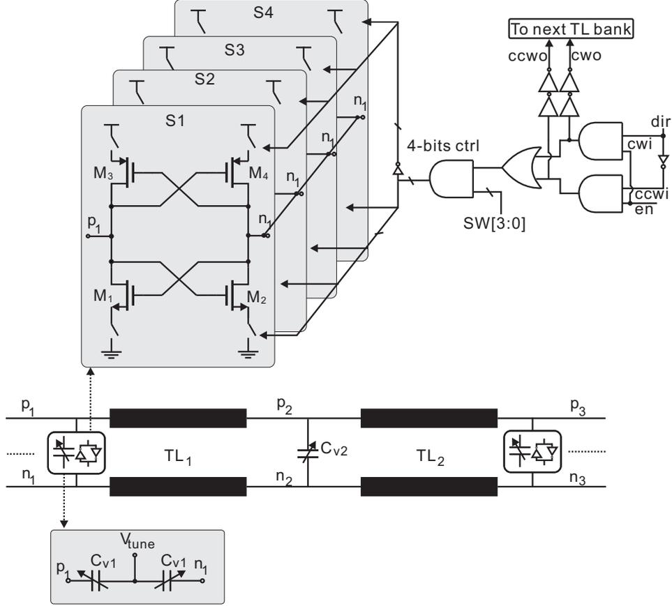
**Figure 3.9:** Two transmission line segments. S1:  $W_N = 2.24 \mu\text{m}$ ,  $W_P = 8.32 \mu\text{m}$ , S2:  $W_N = 1.12 \mu\text{m}$ ,  $W_P = 4.16 \mu\text{m}$ , S3:  $W_N = 0.56 \mu\text{m}$ ,  $W_P = 2.08 \mu\text{m}$ , S4:  $W_N = 0.28 \mu\text{m}$ ,  $W_P = 1.04 \mu\text{m}$ ,  $C_{v1}$ :  $W/L = 25.6 \mu\text{m}/6.5 \mu\text{m}$ ,  $C_{v2}$ :  $W/L = 12.8 \mu\text{m}/6.5 \mu\text{m}$ ,  $V_{\text{tune}} = 0$  to  $-3$  V.
