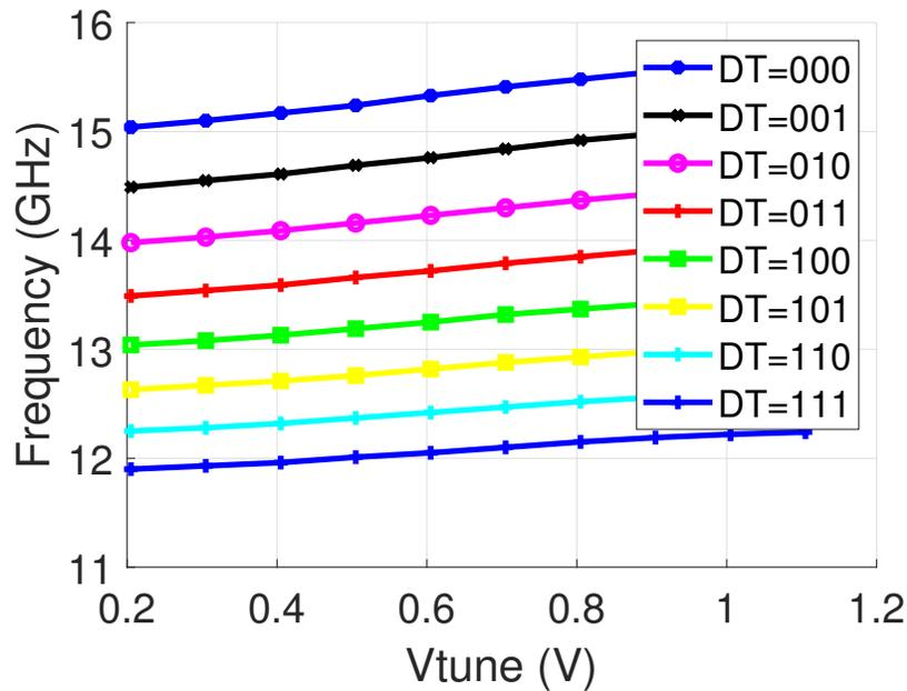
**Figure 4.17:** RTWO(a) frequency tuning(11.89-GHz to 15.67-GHz) under  $TT@40^\circ$
