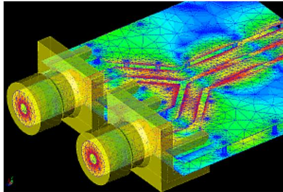
**Figure 1.7:** Mesh network of EM simulation[3]: The lines separate the grid, and the colour shows the magnetic field.
