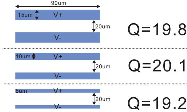
**Figure 3.6:** Compare the couple TLs with different wire width
