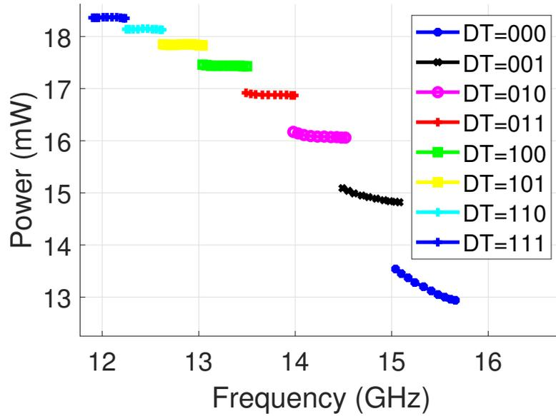
**Figure 4.19:** RTWO(a) power consumption within tuning range(13mW to 18.4mW) under  $TT@40^\circ$
