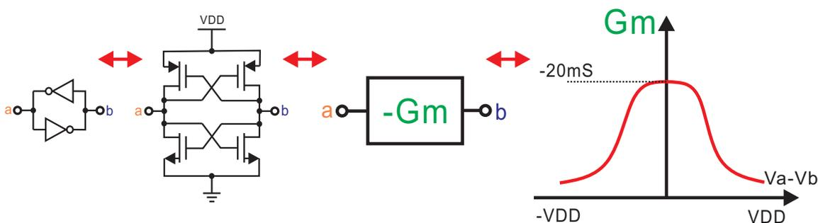
**Figure 2.8:** Cross-coupled pair and  $-G_m$
