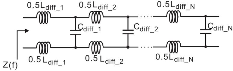
**Figure 2.10:** Lumped model of transmission line
