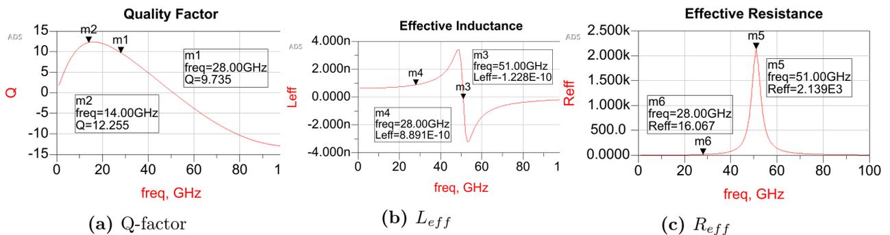
**Figure 4.12:** Properties of proposed 8-shaped inductor
