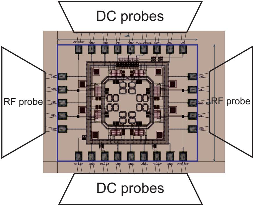
**Figure 5.2:** DUT and probes
