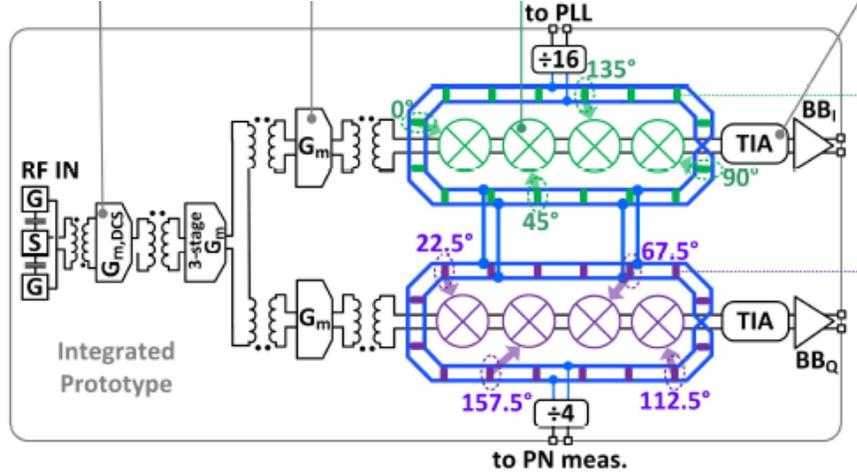
**Figure 2.16:** Block diagram of the proposed coupled-RTWO-based SHRX [32].
