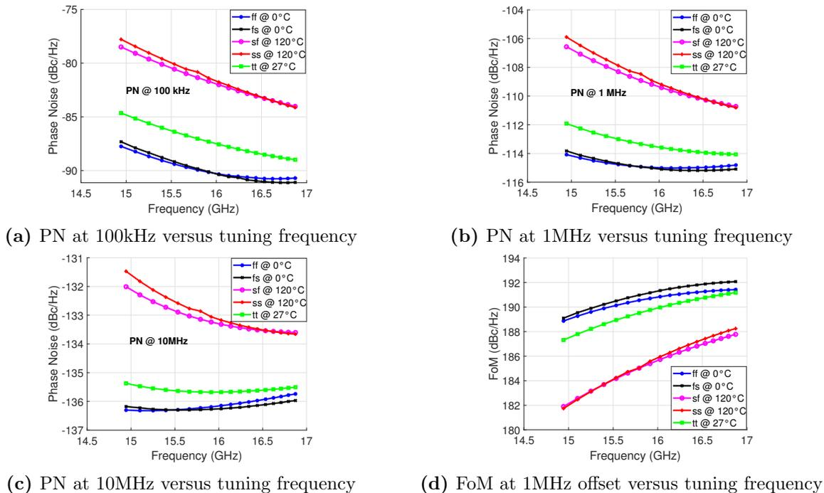
**Figure 3.14:** Frequency and phase noise simulation result
