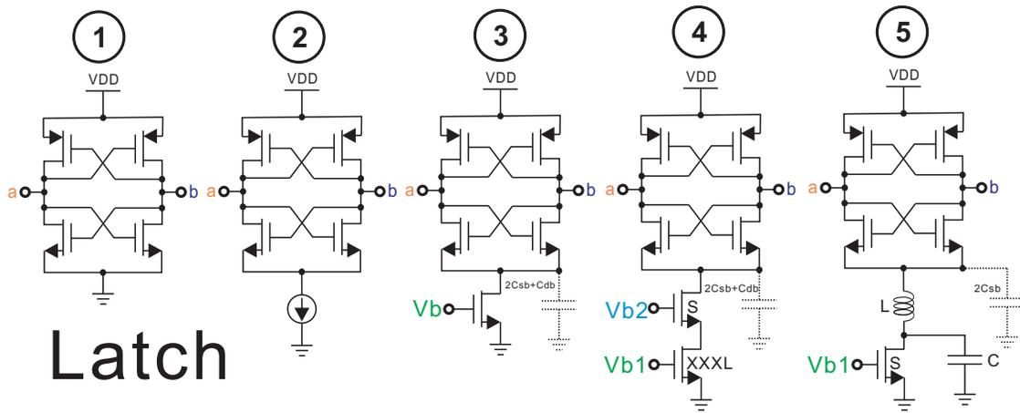
**Figure 4.7:** Different latch designs
