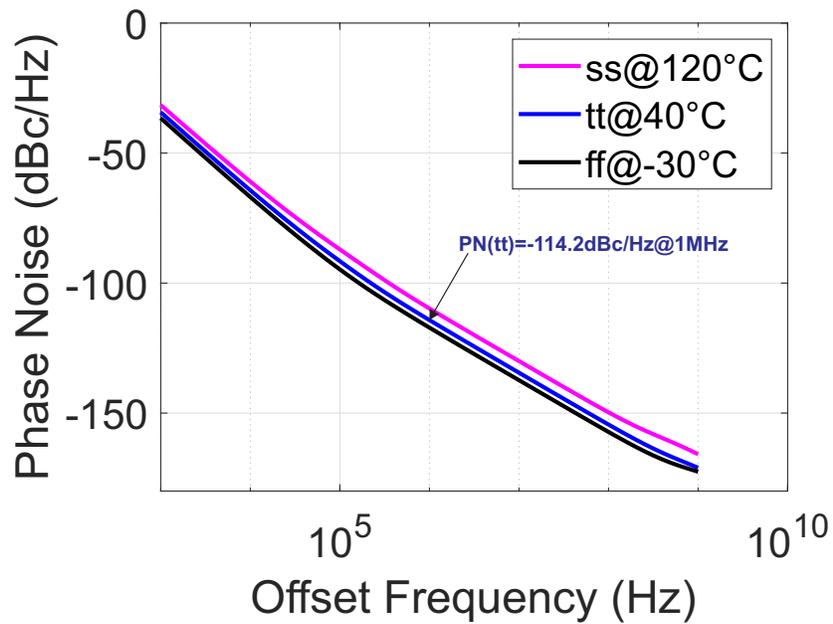
Figure 4.21: RTWO(a) PN across three corners at 13.75-GHz with 16-mW power
