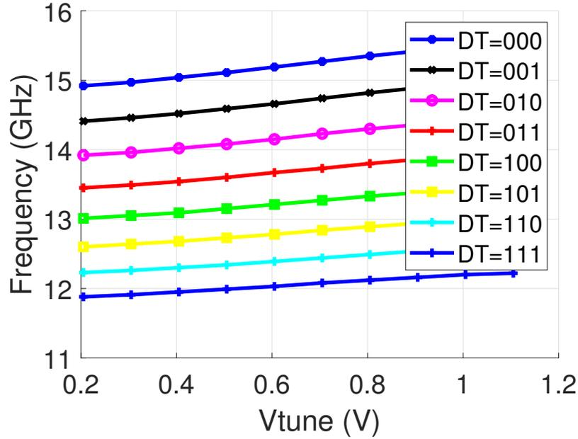
**Figure 4.18:** RTWO(b) frequency tuning(11.87-GHz to 15.55-GHz) under  $TT@40^\circ$
