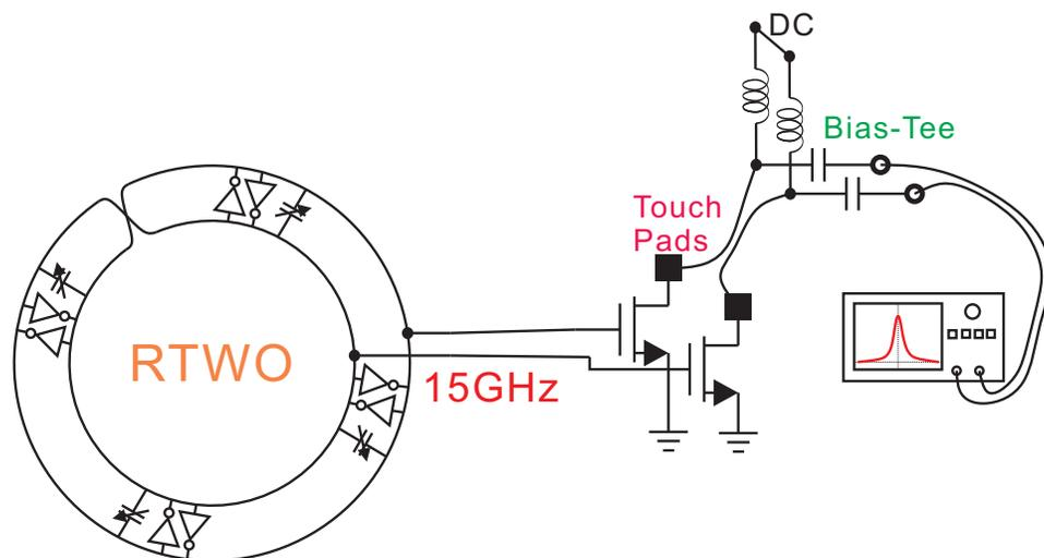
**Figure 5.3:** Testing scheme
