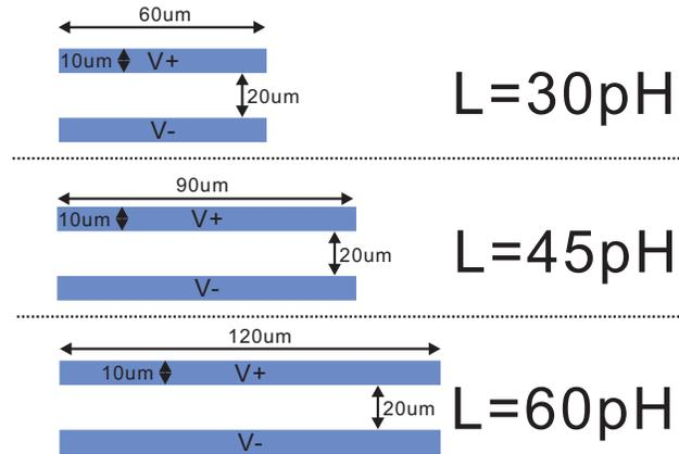
**Figure 3.8:** Compare the couple TLs with different wire length
