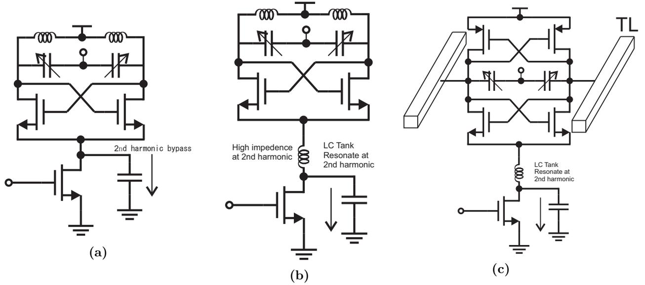
**Figure 4.8:** Tail-based VCO with noise filter
