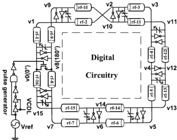
Figure 2.14: RTWO with pulse injector [4].
