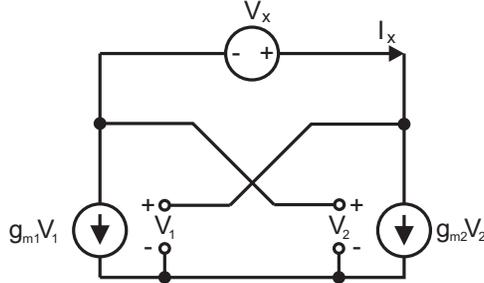
**Figure 2.7:** Equivalent of cross coupled pair
