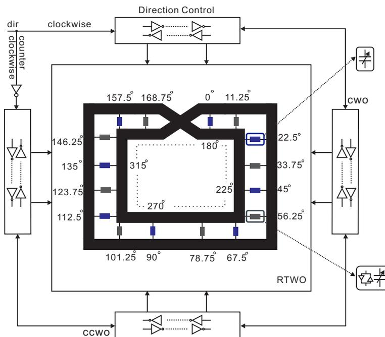
**Figure 3.2:** Proposed RTWO with direction control circuit
