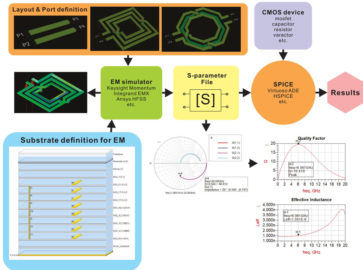
Figure 2.17: Design process with EM simulator
