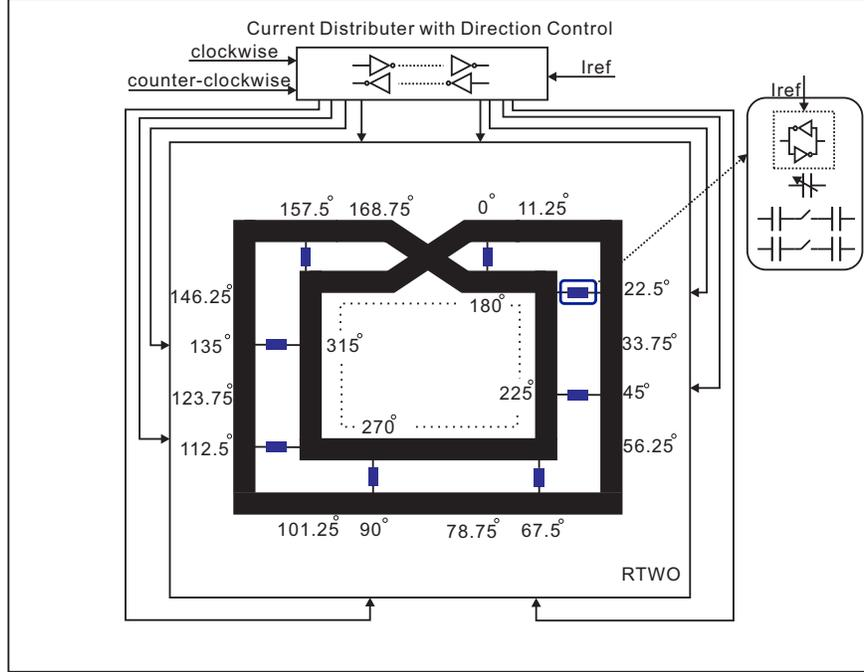
**Figure 4.1:** Circuit Topology of Both RTWO designs
