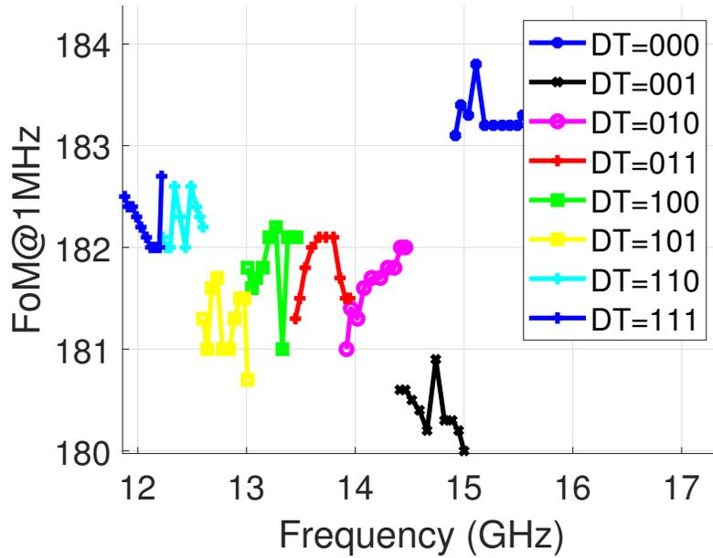
**Figure 4.24:** RTWO(b) FoM with PN@1MHz offset vs Frequency( $TT@40^\circ$ )
