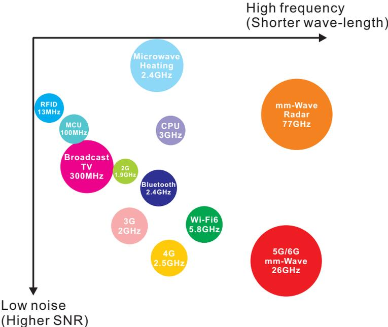
Figure 1.1: Applications of oscillator
