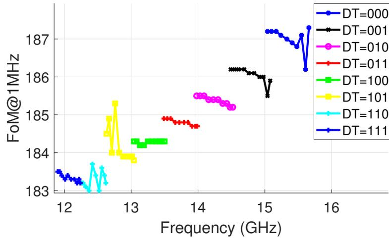
**Figure 4.23:** RTWO(a) FoM with PN@1MHz offset vs Frequency( $TT@40^\circ$ )
