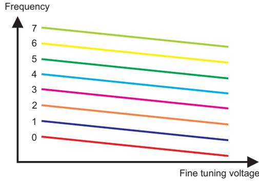
**Figure 4.6:** The curve of a 3-bits discrete tuning band with fine tuning
