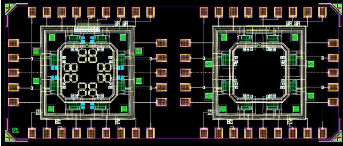
**Figure 4.16:** Full chip layout with sealing
