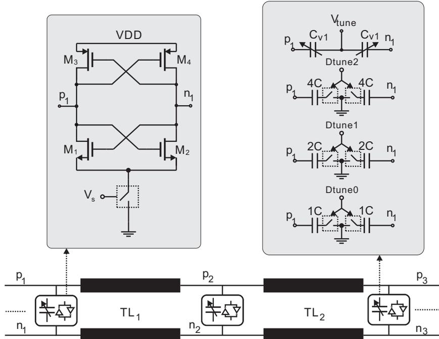
**Figure 4.5:** RTWO(b) with voltage drive latches.  $M_{1,2} = 12 \text{ fingers} \cdot 1.2 \mu\text{m}/130\text{nm}$ ,  $M_{3,4} = 12 \text{ fingers} \cdot 2.4 \mu\text{m}/130\text{nm}$ ,  $M_{\text{switch}} = 16 \text{ fingers} \cdot 8 \mu\text{m}/130\text{nm}$ ,  $V_{\text{tune}} = 0$  to  $1.2$  V,  $C_{v1} = 13\text{fF}$  to  $41\text{fF}$ ,  $C = 26\text{fF}$ ,  $V_s = 0$  or  $1.2$  V
