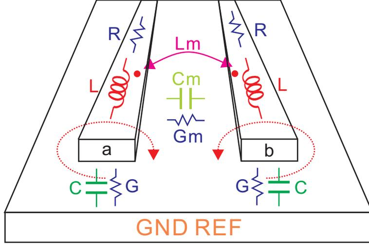
**Figure 2.9:** Transmission line RLGC model
