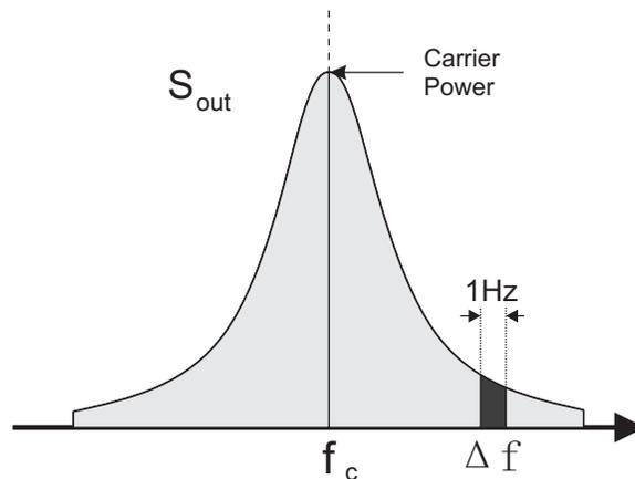
**Figure 2.3:** Specification of phase noise.
