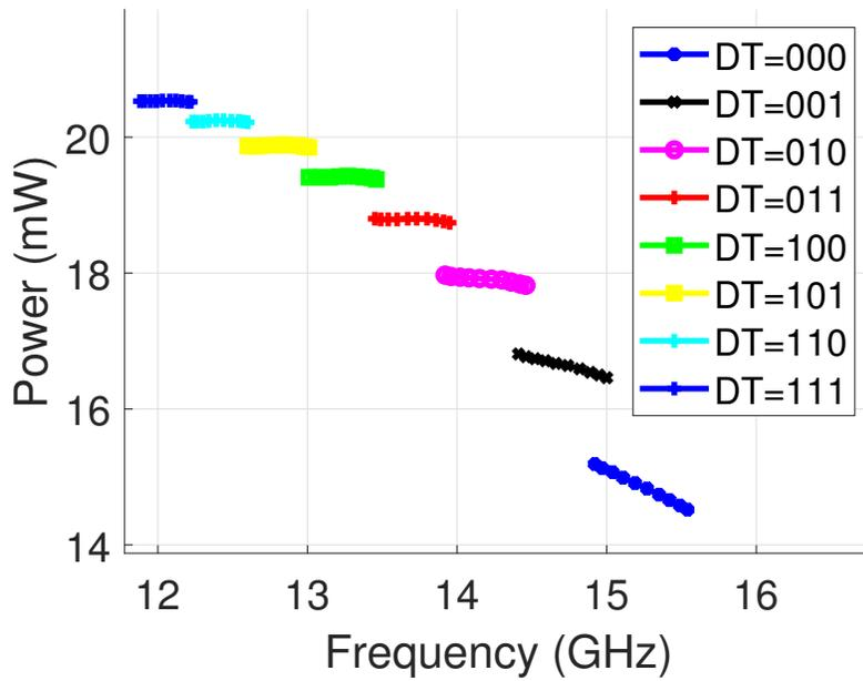
**Figure 4.20:** RTWO(b) power consumption within tuning range(14.6mW to 20.5mW) under  $TT@40^\circ$
