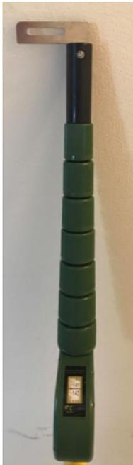
Figure 2. Height pole used to measure tree heights at the Kakabeka white spruce provenance tests.
