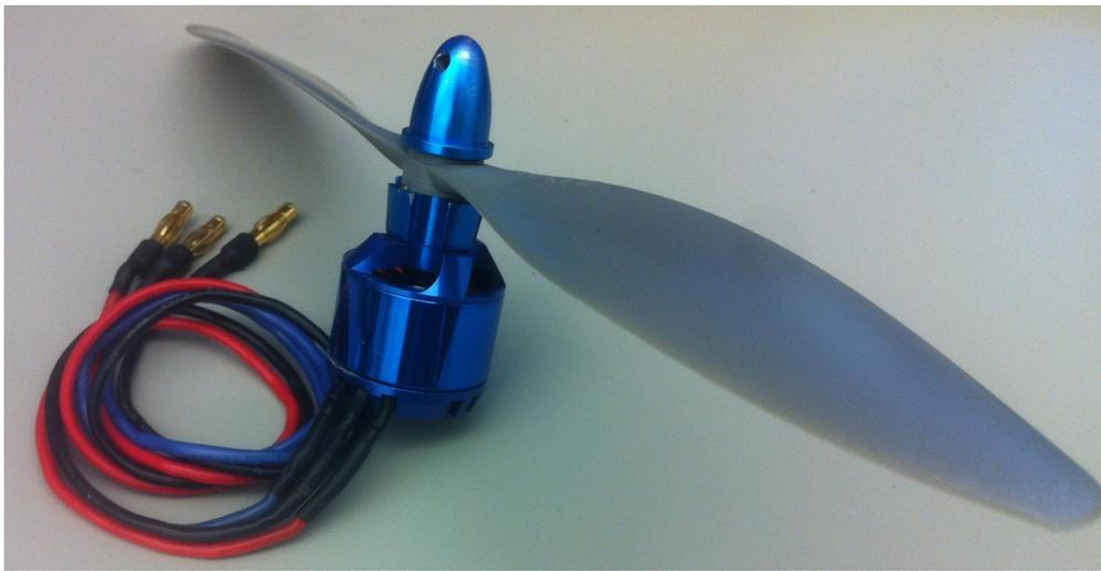
FIGURE 6.4: A2830-12 outrunner motor with 4.7in/rev propeller attached.
