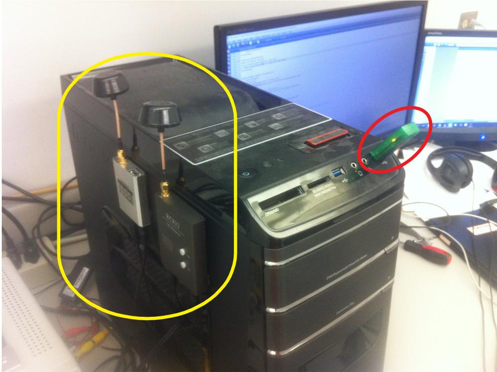
FIGURE 6.6: Base station computer with XStick (circled in red) and video receivers (circled in yellow).
