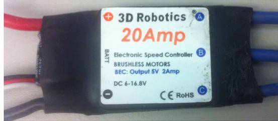
FIGURE 6.5: 20Amp ESC used for this work.
