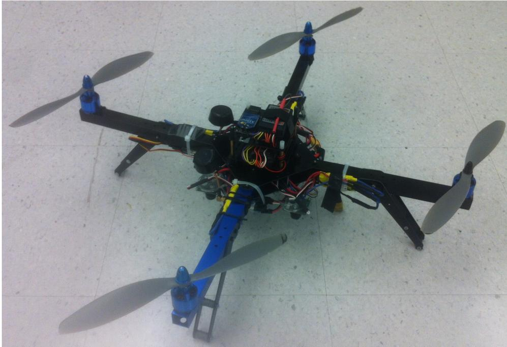
FIGURE 6.2: Quadrotor experimental platform.
