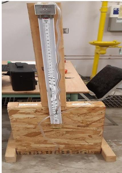
Fig. 14: Pitot tube and manometer
