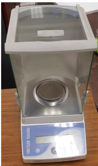
Fig. 9: Precision weighing scale
