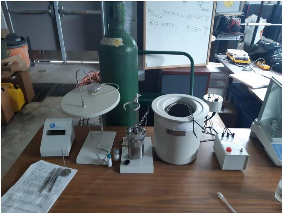
6. Bomb calorimeter setup
