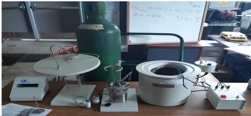
Fig. 10: Bomb Calorimeter set up
