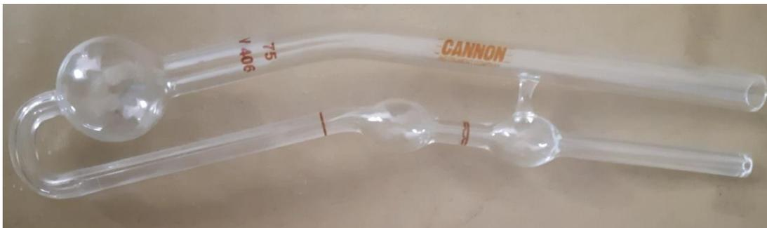
Fig. 7: Viscometer
