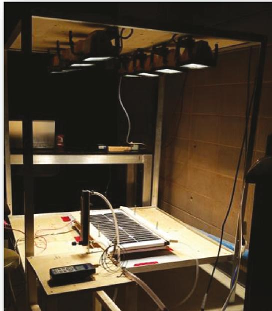
**Figure 4.4: A photograph showing the indoor experimental simulation of 40W-HPV-10TEG module using solar simulator used in this investigation.**
