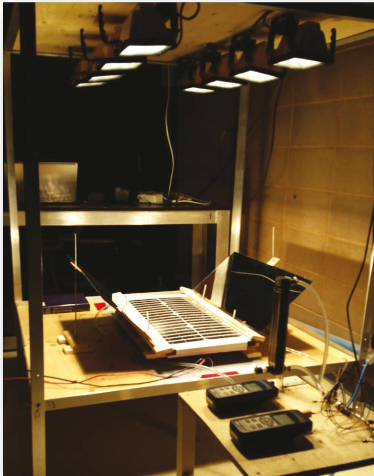
**Figure 4.18: Photograph of the concentrated hybrid photovoltaic-thermoelectric power generation module (40W-CHPV-10TEG).**
