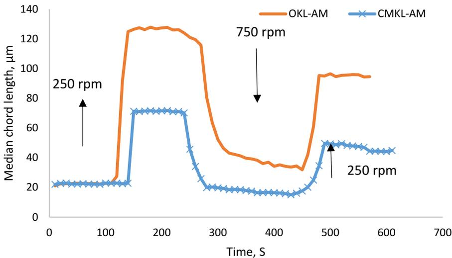
Figure 4. 8. Flocculation evolution OKL-AM, and CMKL flocculants in alumina suspension.
