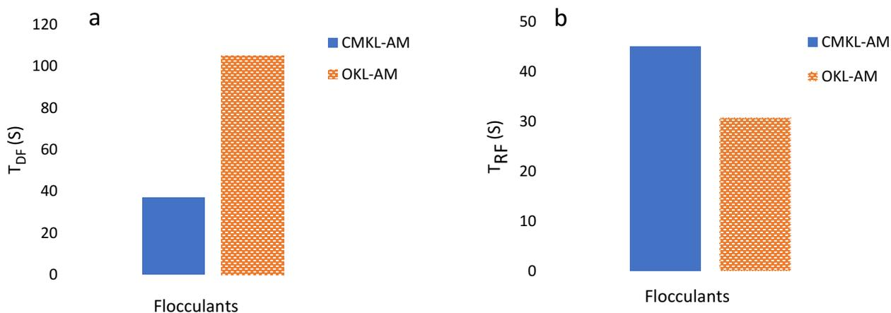
Figure 4.9. a) Flocc formation tendency ( $T_{df}$ ) and b) floccs reflocculation tendency ( $T_{rf}$ ) values for CMKL-AM, OKL-AM polymers.
