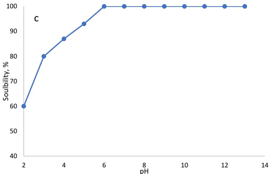
Figure 3.1. The effect of solution pH on KL-AM polymer's, a) molecular weight and charge density, b) grafting ratio and yield, c) solubility.
