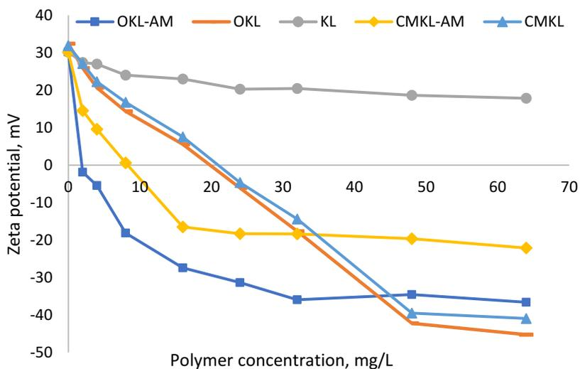
Figure 4.4. Alumina suspension's zeta potential as a function of polymer concentration, which was conducted under the conditions of pH 6, 30 min incubation at 30 °C, and 1 g/L of alumina concentration.
