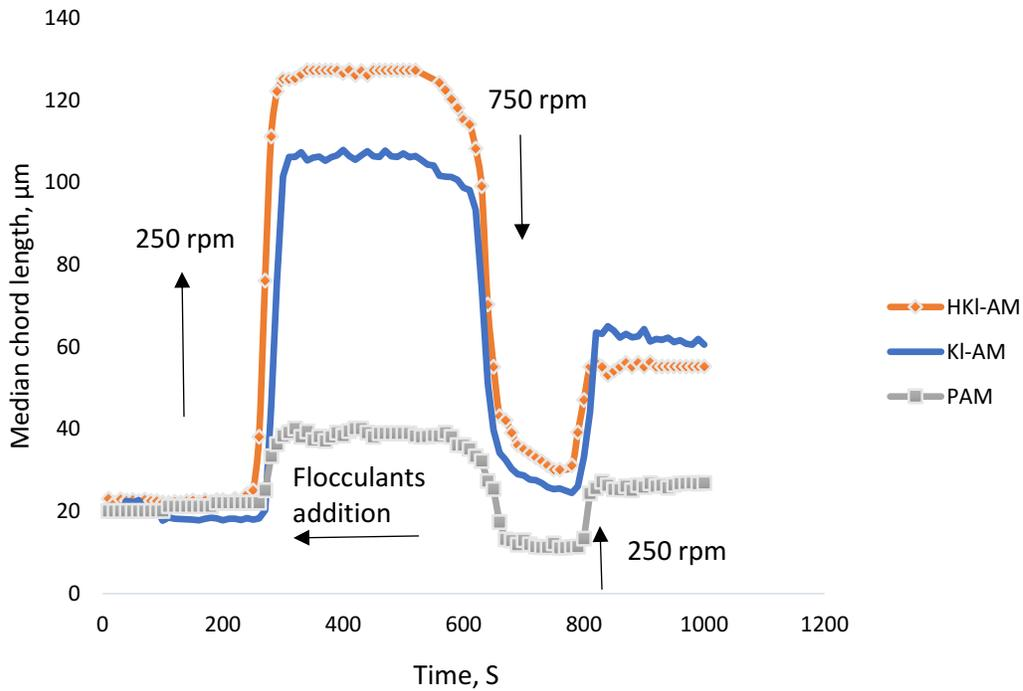
Figure 3.14. Evolution of flocculation process for different flocculants in alumina suspension.
