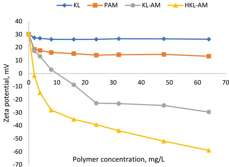
Figure 3.9. Alumina suspension’s zeta potential as a function of polymer concentration conducted under the conditions of pH 6, 30 min incubation at 30 °C, and 1 g/L of alumina concentration.
