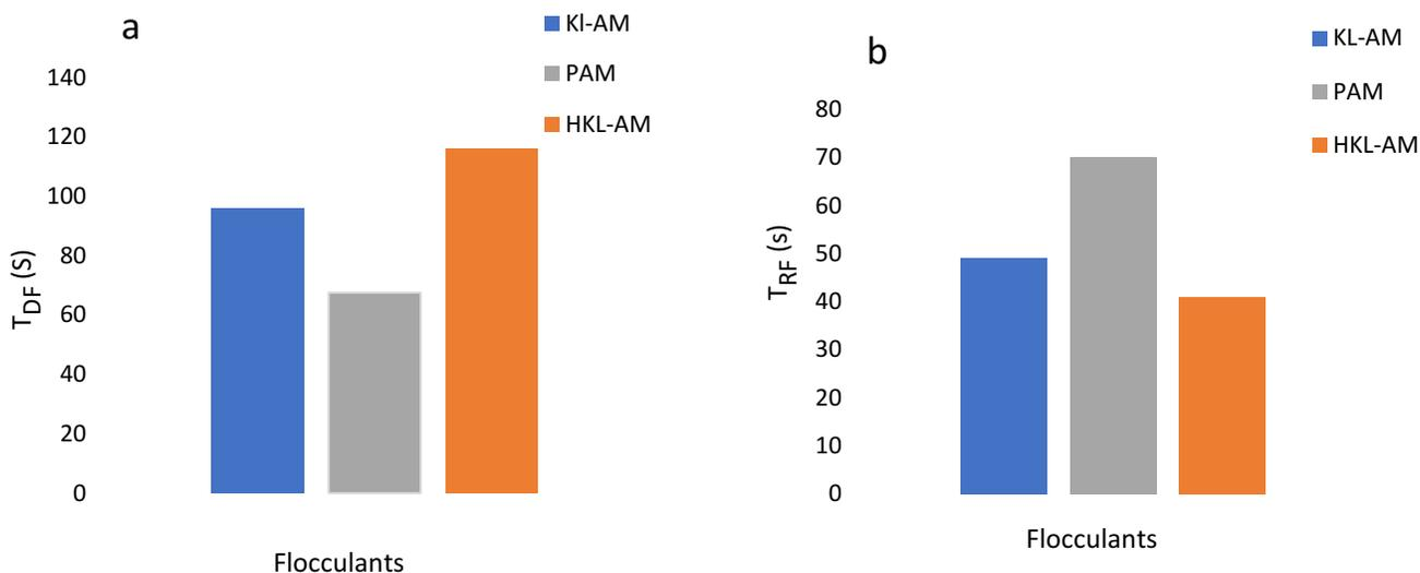
Figure 3.15. a) Flocs formation tendency ( $T_{df}$ ), and b) flocs re-flocculation tendency ( $T_{rf}$ ) values for KL-AM, PAM, and HKL-AM polymers.
