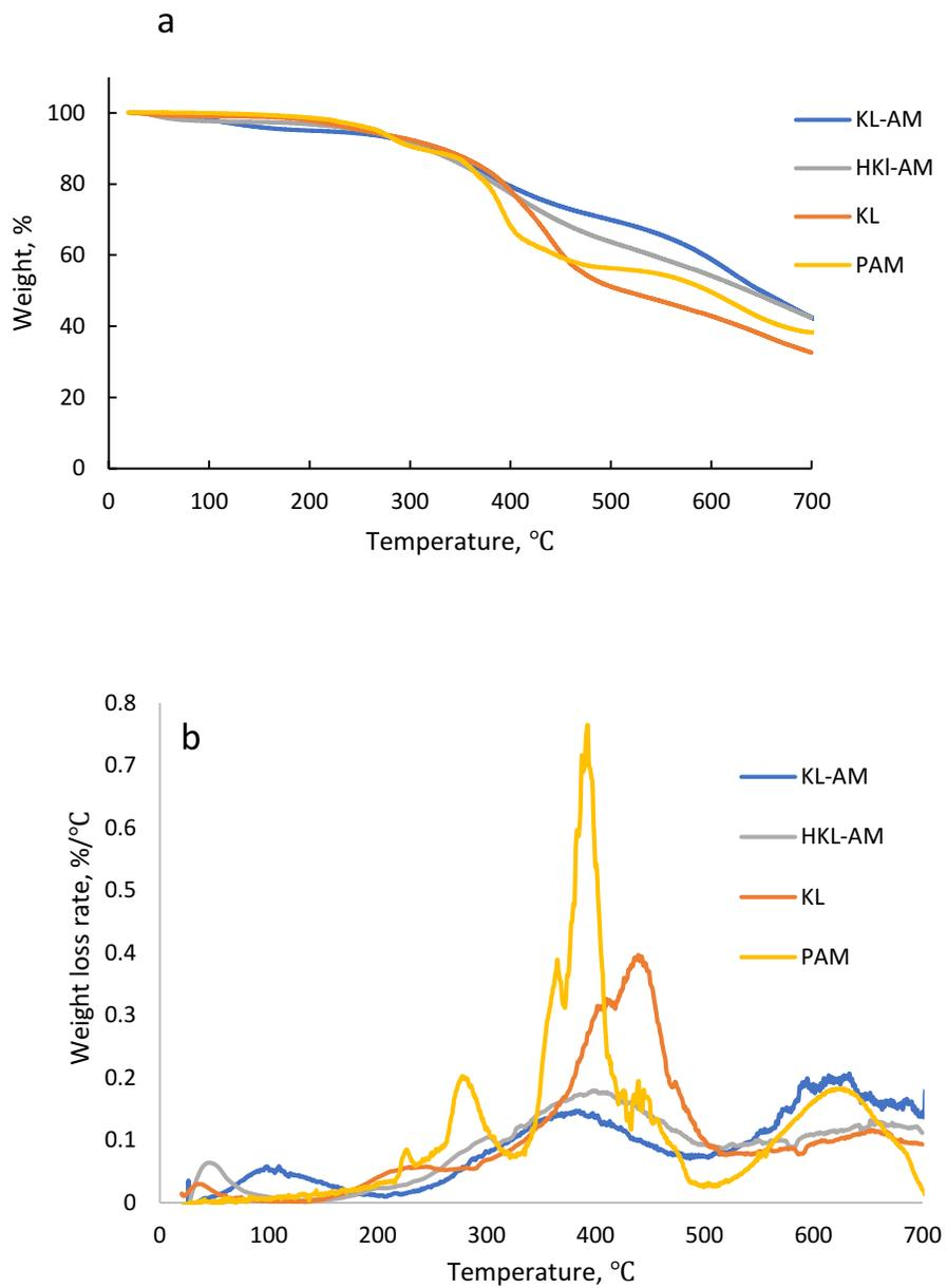
Figure 3.5. a) Weight loss and b) Weight loss rate of KL, KL-AM, and HKL-AM polymers conducted under  $N_2$  with the flow rate of 30 mL/min heated at 10 °C/min.
