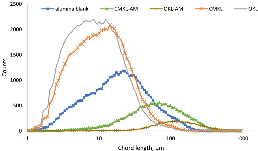
Figure 4.7. Chord length distribution of aluminum oxide particles formed under polymers optimal dosages used in relative turbidity analysis.
