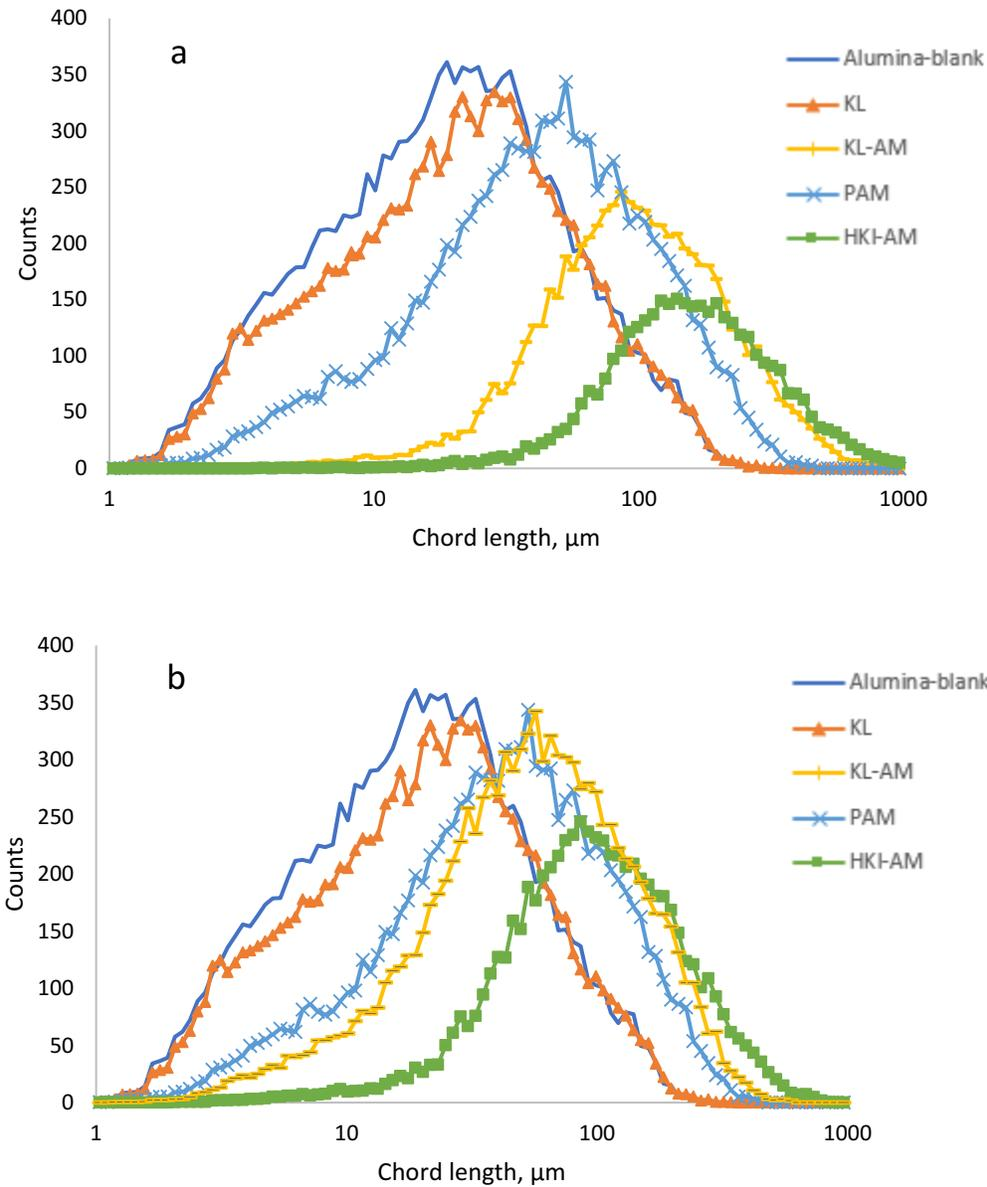
Figure 3.13. Chord length distribution of aluminum oxide flocs formed under a) polymer dosage of a) 10 mg/g, and b) 20 mg/g.
