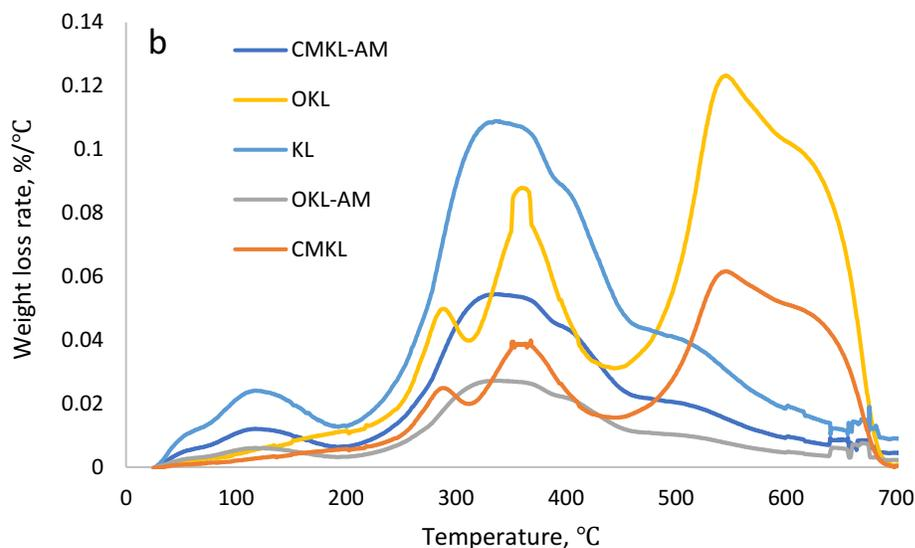
Figure 4.2. a) weight loss and b) weight loss rate of polymers at a nitrogen flow rate of 35 mL/min.
