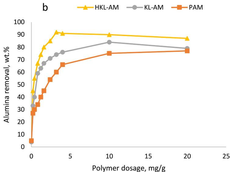
Figure 3.10. a) Influence of polymer dosage on the relative turbidity of alumina suspension, b) alumina removal as a function of polymer dosage. The experiments were conducted under the conditions of 25 °C for 2h at pH 6.
