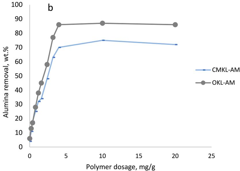
Figure 4.5. a) Influence of polymers dosages on alumina suspension relative turbidity, b) Alumina removal as a function of polymers dosage. The experiments were conducted under the conditions of 25 °C for 2h at pH 6.
