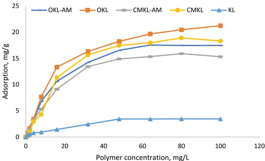
Figure. 4.3. Adsorption isotherms of KL, OKL, OKL-AM, CMKL, and CMKL-AM on alumina particles conducted at pH 6, and room temperature.
