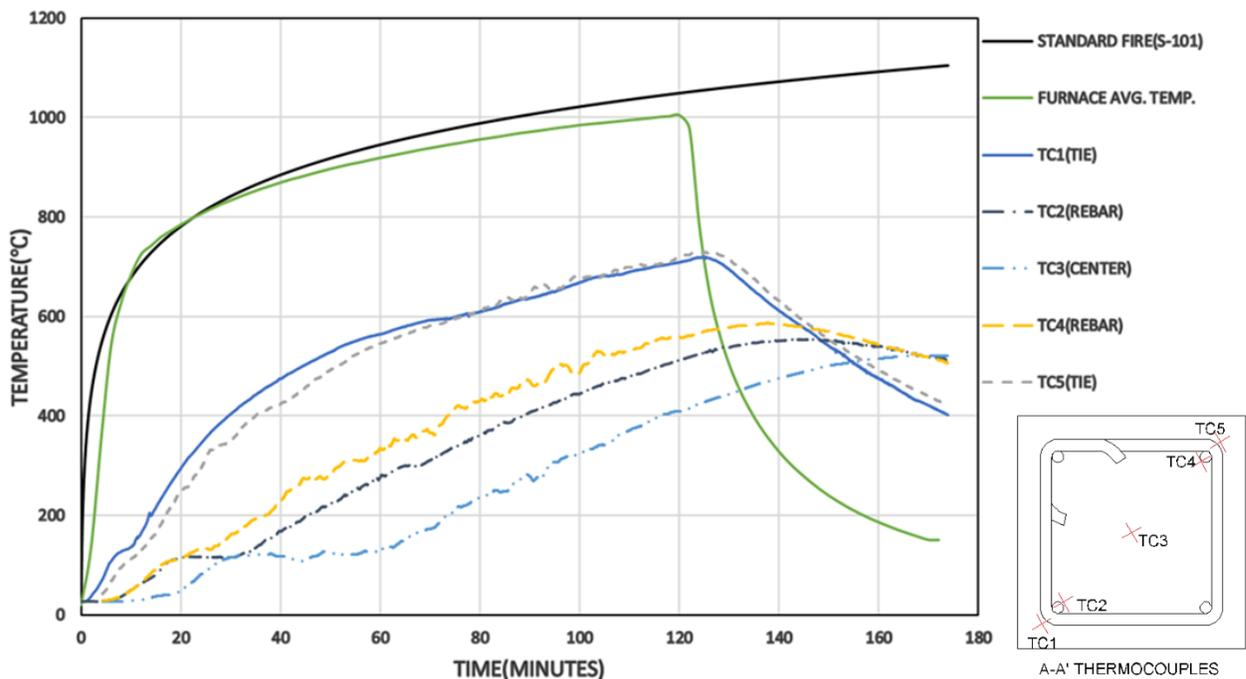
**Figure 4.6.** Time-temperature curves for a 2-hour fire duration test
