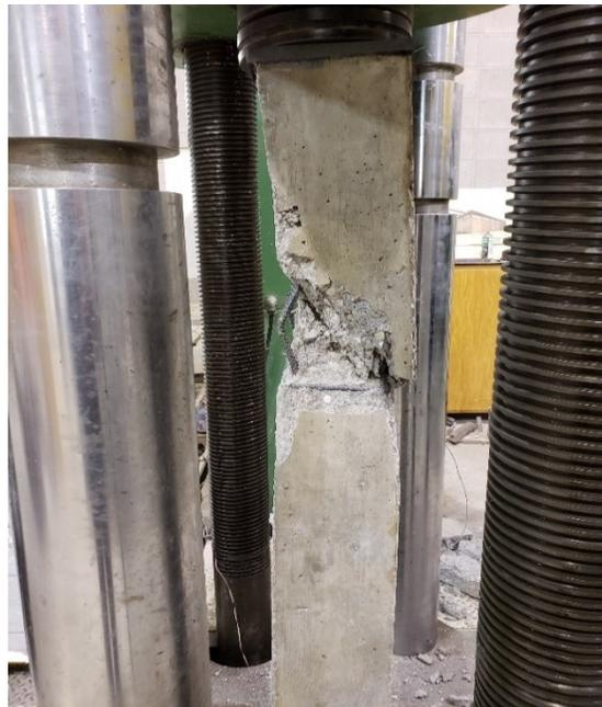
**Figure 4.1** Crushing failure of one of the two columns tested at ambient temperature
