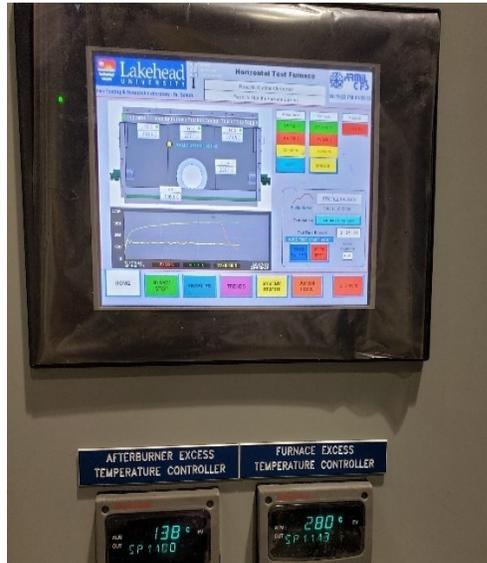
**Figure 3.10.** Human-Machine Interface (HMI) touch screen of the furnace's control panel
