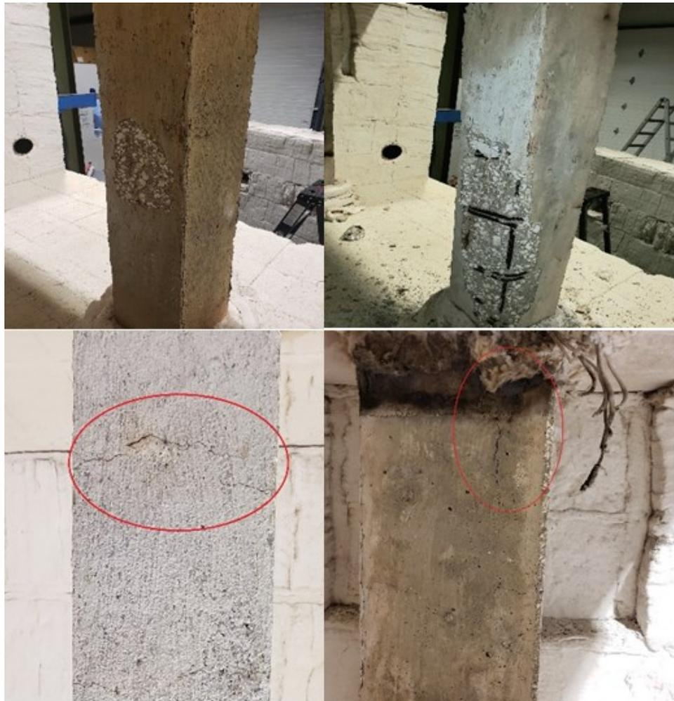
**Figure 4.8.** Column specimens subjected to 2-hour fire exposure and 60% load ratio, (a) spalling from one side; (b) crack pattern
