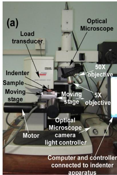
**Figure 2.5** Micro indentation apparatus
