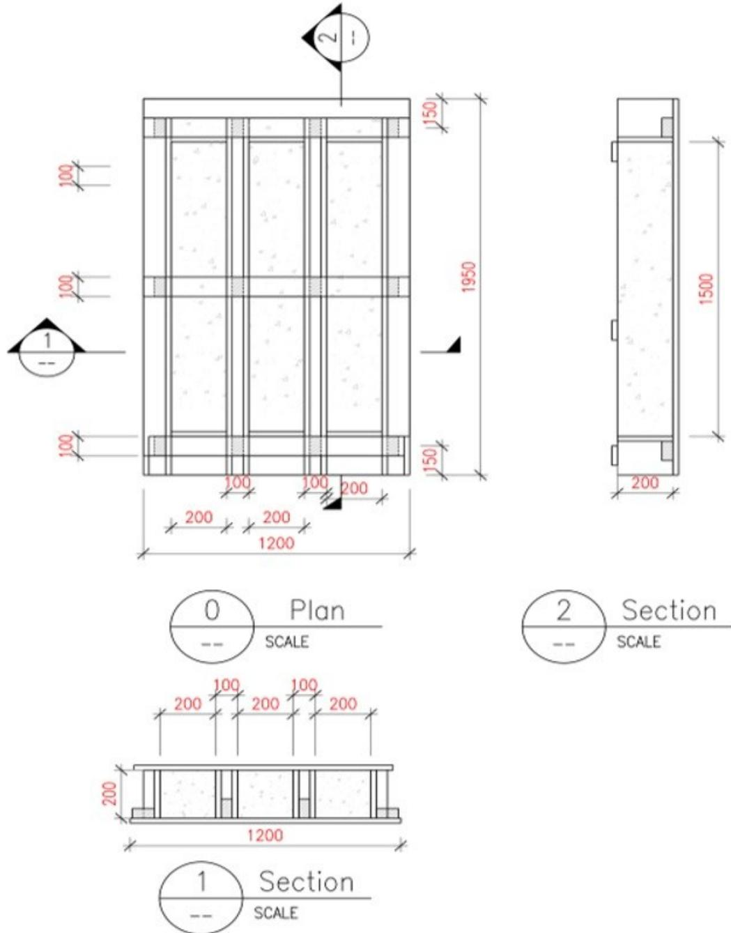
Figure C-1. Column specimens' formwork details
