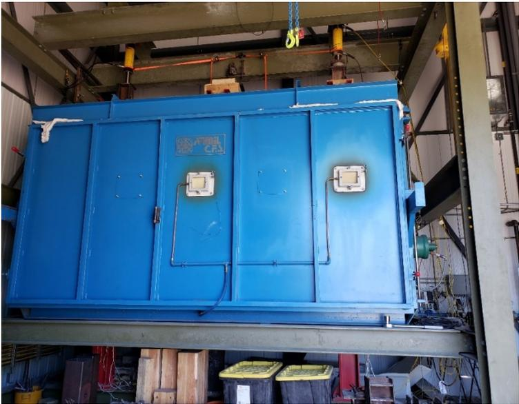
**Figure 3.9.** Large custom-designed fire testing furnace
