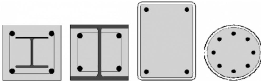
**Figure 2.3** Composite columns (Adapted from steelconstruction.info, 2018)
