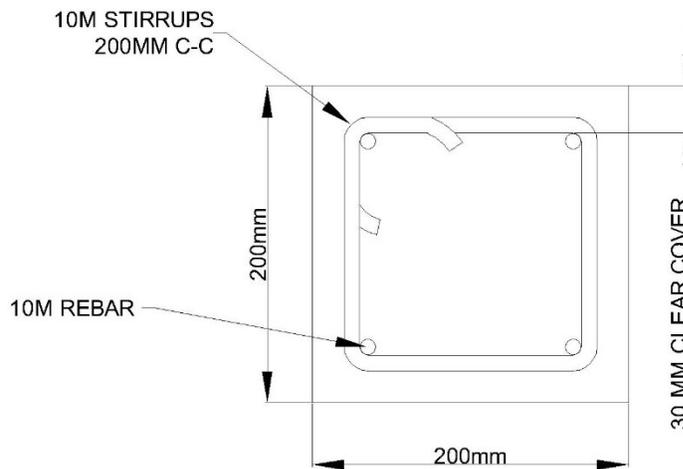
**Figure A.1** Column Cross-section
