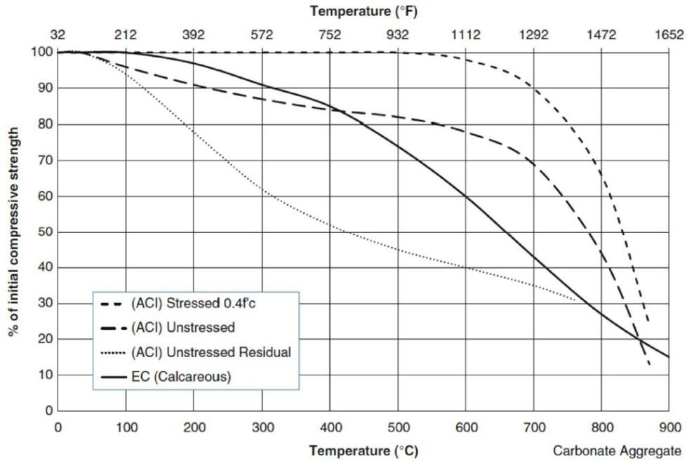
**Figure B-3.** Strength-temperature relationships for Carbonate Aggregate (Adapted from Eurocode 2)
