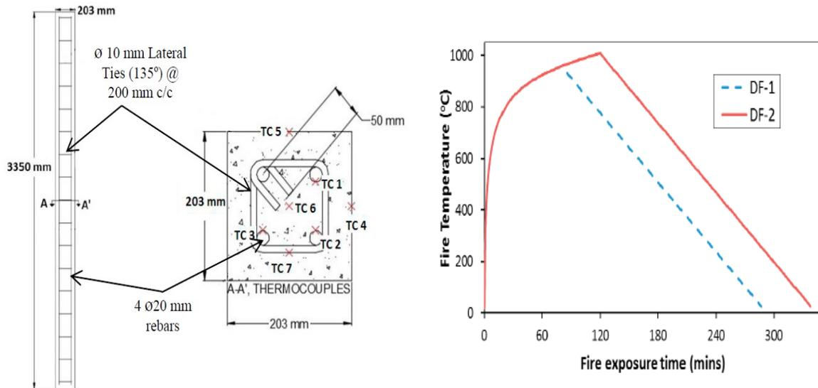
**Figure 2.10.** Reinforcement details and design fire curve (Adapted from Kodur *et al.*, 2017)
