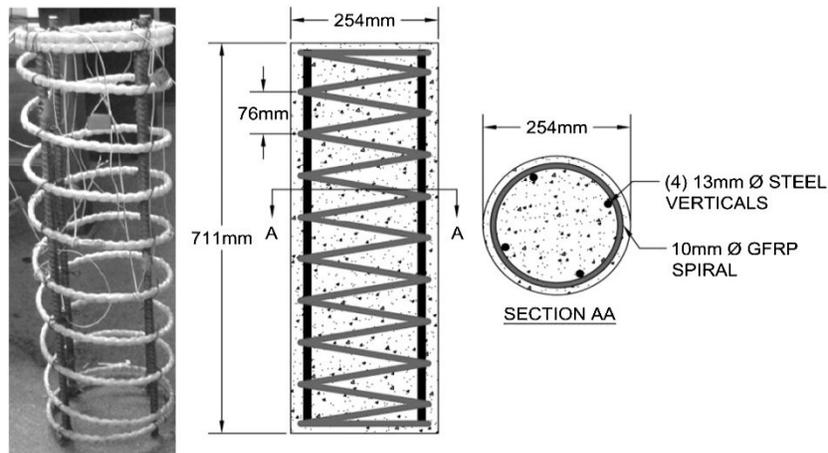
**Figure 2.2** Spirally reinforced columns (Adapted from ASCE library, 2018)
