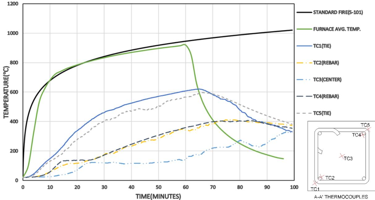
**Figure 4.4.** Time-temperature curves for a 1-hour fire duration test
