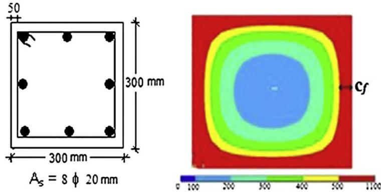
**Figure 2.14** Cross section of column and its thermal contour
