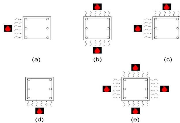
**Figure 2.9** Various surface areas of fire exposure (a) on single face; (b) on two opposite faces; (c) on two adjacent faces; (d) on half of the cross section; (e) on four faces (Adapted from Balaji *et al.*, 2016)
