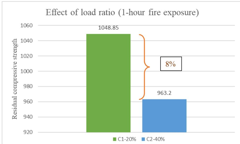
**Figure 5.3** Residual compressive strength of columns subjected to different load ratios (1-hour)
