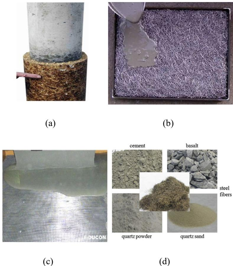
**Figure 2.19** Advanced strengthening materials (a) Polymer concrete; (b) SIFCON; (c) DUCON; (d) Single components of UPHC (Adapted from Roller *et al.*, 2013)
