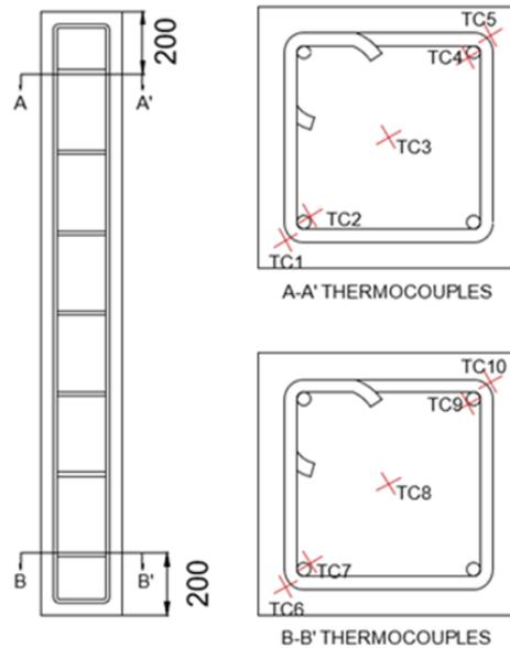
**Figure 3.3.** Thermocouples layout at two different elevations of a general test specimen
