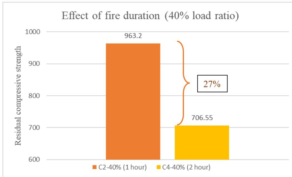
**Figure 5.6** Residual compressive strength of columns subjected to different fire durations (40% load ratio)
