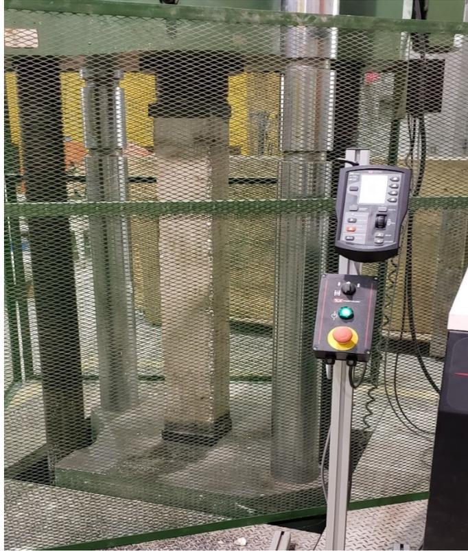
**Figure 5.1.** A general column residual strength test setup
