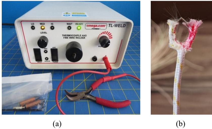
**Figure 3.4.** Thermocouples preparation, (a) Fine-gauge wire welding machine; (b) a typical thermocouple bead
