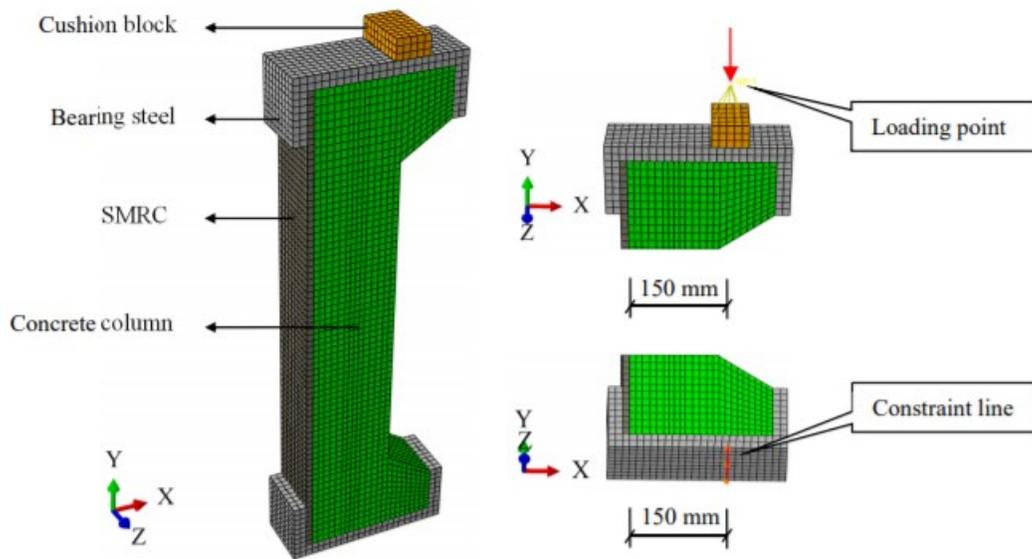
**Figure 2.16.** Finite element model and boundary condition (Adapted from Li *et al.*, 2018)
