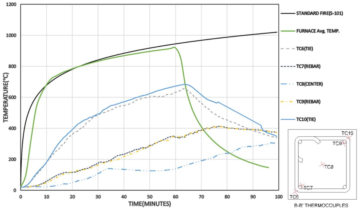
**Figure 4.5.** Time-temperature curves for a 1-hour fire duration test
