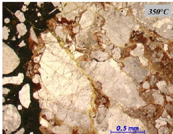
**Figure 2.6** Reddish brown coloration of siliceous aggregate at 350°C (Adapted from Annerel and Taerwe, 2009)
