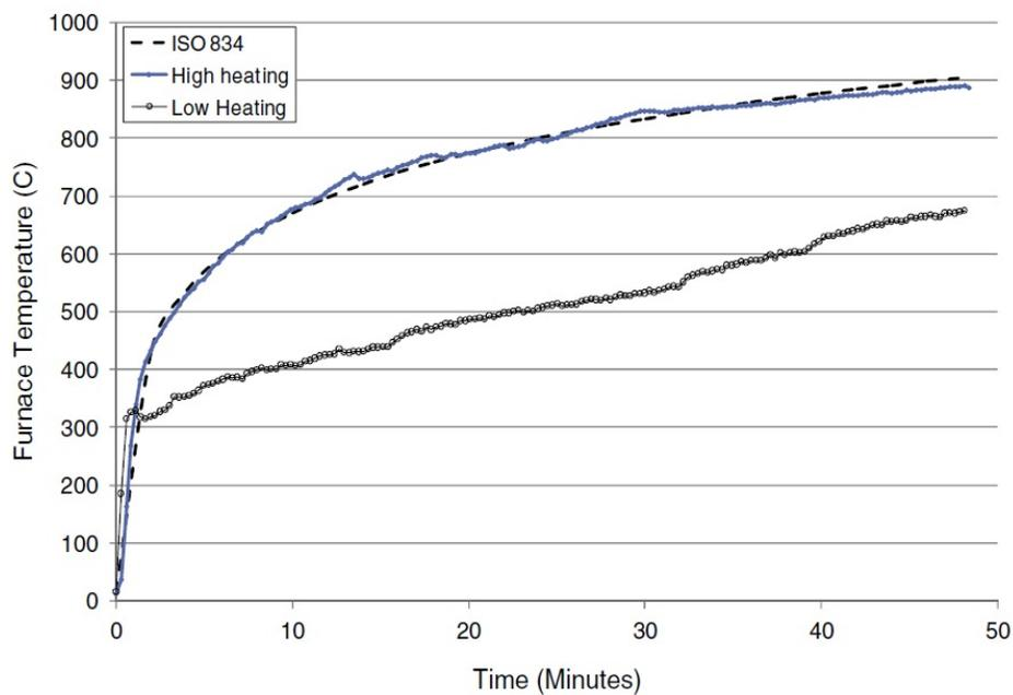
**Figure 2.8** Fire curve for experimental testing (Adapted from Ali *et al.*, 2010)
