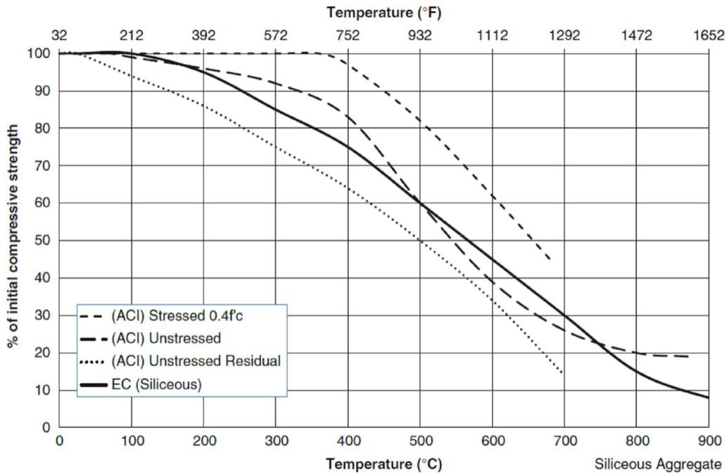
Figure B-2. Strength-temperature relationships for Siliceous Aggregate (Adapted from Eurocode 2)
