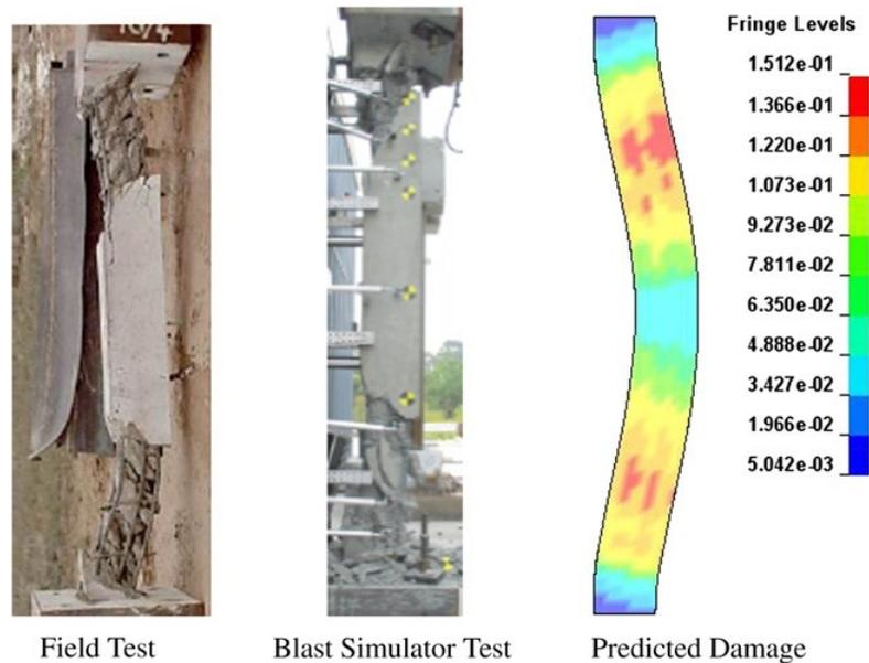
**Figure 2.17.** Comparison of numerical and experimental response of reinforced concrete columns (Adapted from Bao and Li, 2010)
