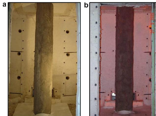
**Figure 2.20** Insulated FRP wrapped column (before and after fire exposure)
