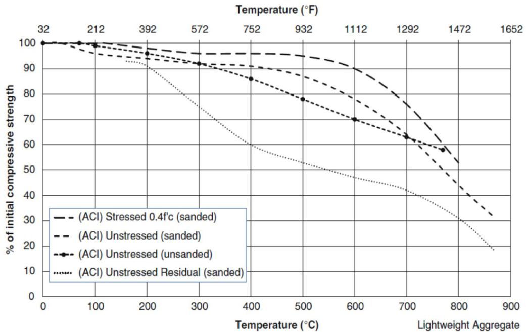
**Figure B-4.** Strength-temperature relationships for Lightweight aggregate (Adapted from Eurocode 2)
