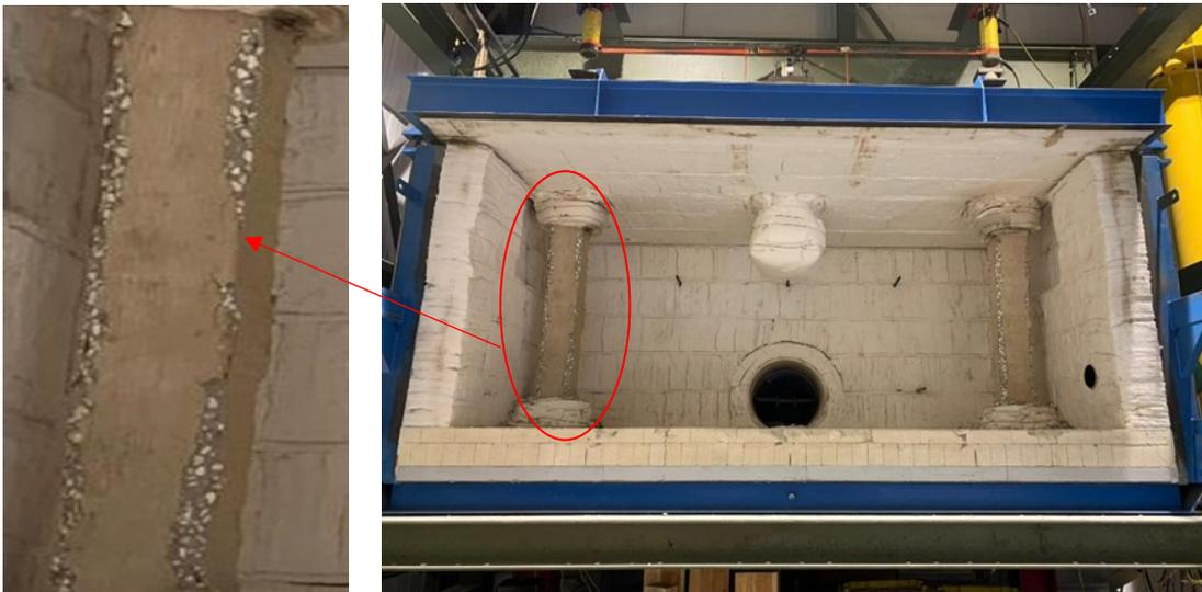
**Figure 4.9.** Column specimens underwent 2-hour fire exposure with its corners damaged
