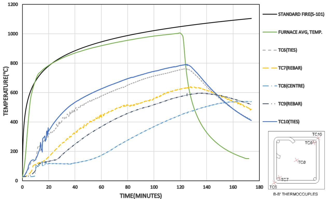
**Figure 4.7.** Time-temperature curves for a 2-hour fire duration test
