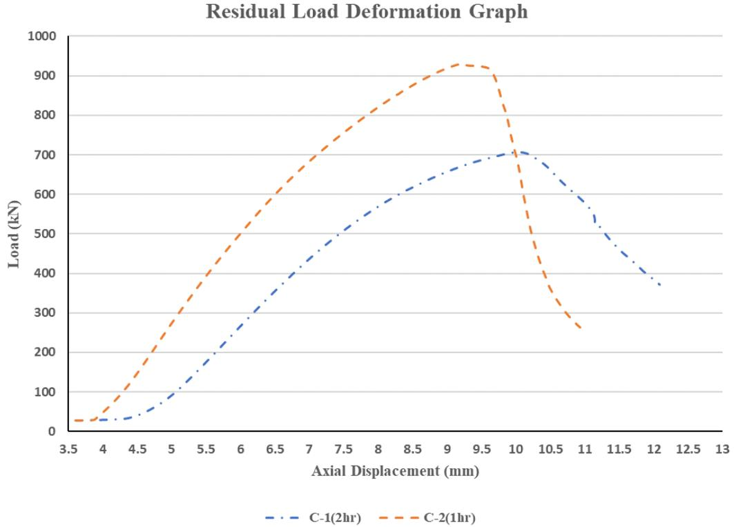
**Figure 5.2** Residual load-deformation relationships for two column specimens exposed to 1- and 2-hour fire duration, and both subjected to 40% load ratio
