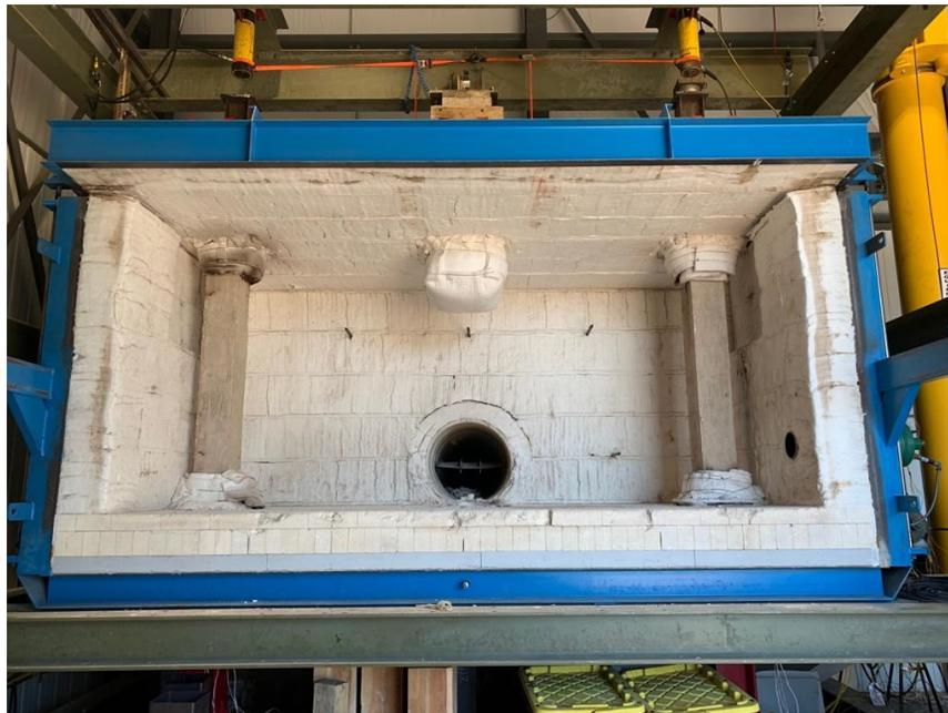
**Figure 3.13.** LUFTRL's fire testing furnace with two columns placed inside
