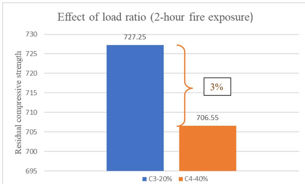
**Figure 5.4** Residual compressive strength of columns subjected to different load ratios (2-hour)
