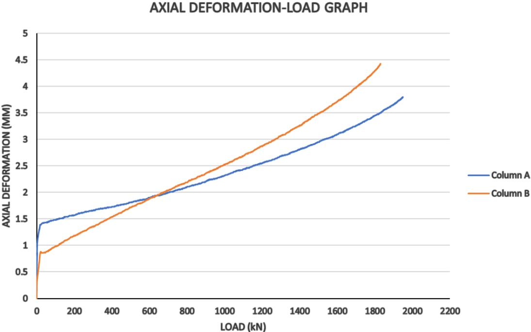
**Figure 4.2.** Ambient temperature tests axial deformation-load relationships
