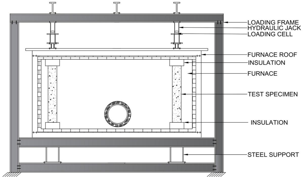
**Figure 3.12.** Schematic of a general fire test setup
