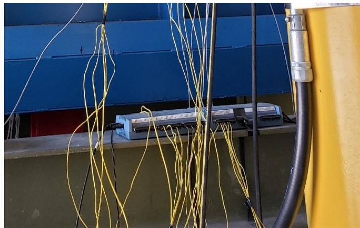
**Figure 3.14.** Thermocouple wires attached to the data acquisition system
