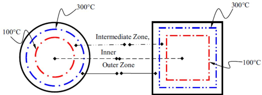
**Figure 2.12** Fire damaged zoning for circular and square columns
