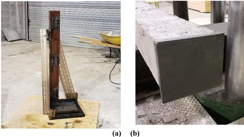
**Figure 3.7.** RC column end compound capping process, (a) capping rig; (b) prepared column end capping.
