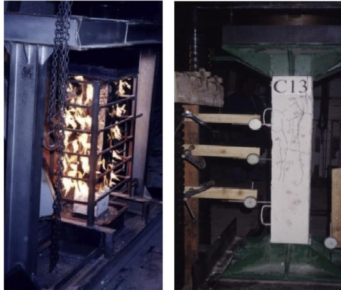
**Figure 2.11** Fire test and loading frame (Adapted from Bikhiet *et al.*, 2014)
