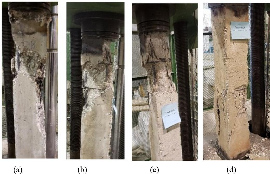
**Figure 5.7.** Failure of fire damaged columns after being loaded, (a) column of 1-hour fire duration and 20% load ratio; (b) column of 1-hour fire duration and 40% load ratio; (c) column of 2-hour fire duration and 20% load ratio; (d) column of 2-hour fire duration and 40% load ratio.
