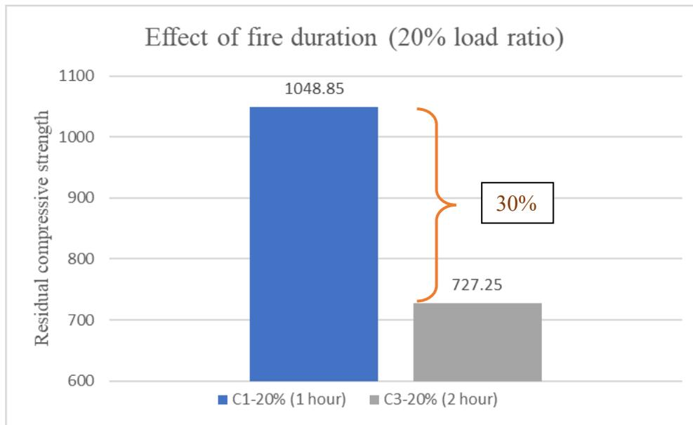
**Figure 5.5** Residual compressive strength of columns subjected to different fire durations (20% load ratio)
