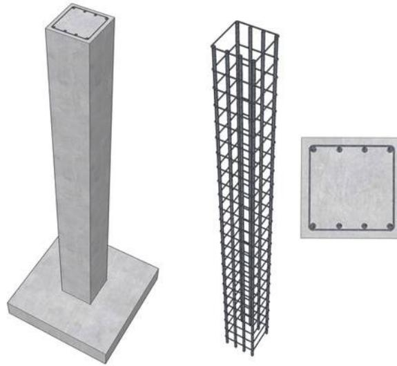
**Figure 2.1** Tied columns (Adapted from Structure point.org, 2018)
