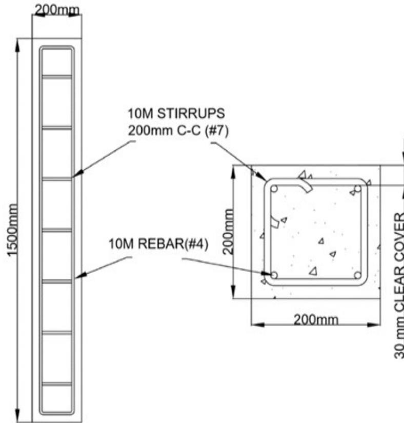
**Figure 3.1.** Dimensions and reinforcement details of reinforced concrete columns
