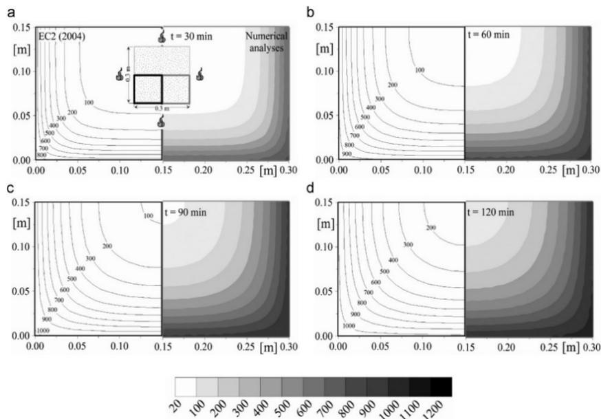
**Figure. 2.13** Square column: comparison between the thermal fields evaluated numerically (right) and given by EC2, at different fire durations: 30 (a), 60 (b), 90 (c) and 120 min (d).
