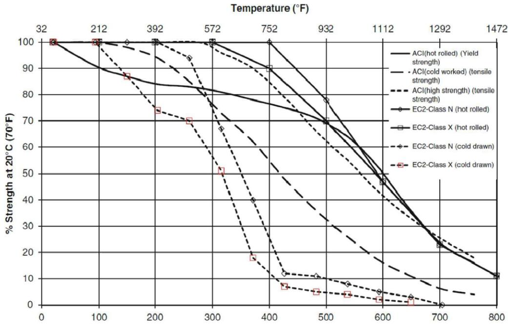
Figure B-1. Strength-temperature relationships for reinforcing steel (Adapted from Eurocode 2)
