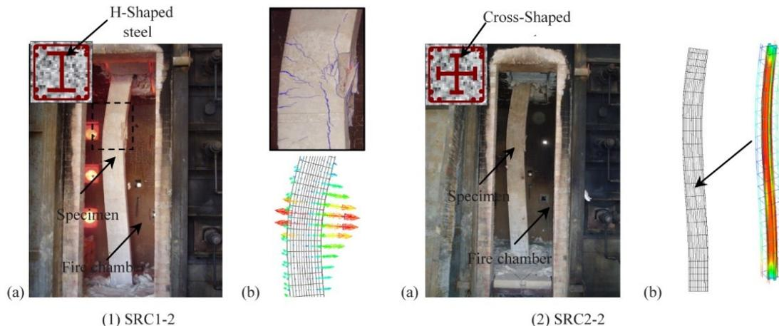
**Figure 2.7** SRC column (Adapted from Han *et al.* 2013)
