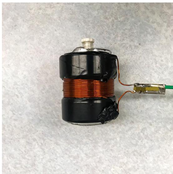
Figure 20: The Rabi detection coil. The Rabi detection circuitry outlined in Figure 17B with a 30mL water sample placed inside.
