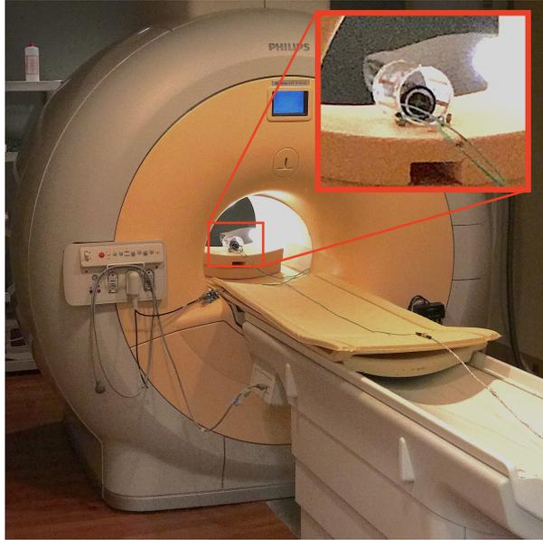
Figure 21: MRI Experiment Set Up. The Birdcage coil used to produce the  $B_1$  field is placed in the centre of the magnet and connected to the  $\lambda/8$  hybrid coupler which is then fed to the DFG of the scanner. The detection coil is placed in the centre of the birdcage coil with its output being fed through an interface to outside the scanner room to the filter circuit (Figure 19) and then to an oscilloscope where data is recorded and visualized.
