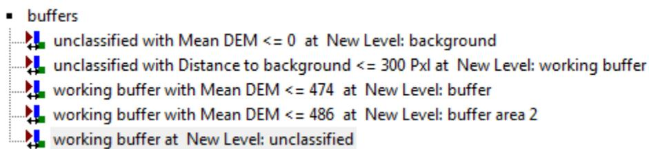
Figure 8: Process tree for classifying buffer area in eCognition.
