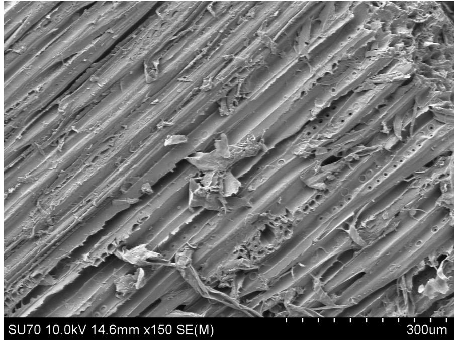
Figure 23. Tangential view of glulam displaying rays and fusiform rays.
