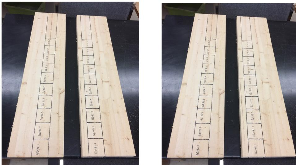
Figure 10. Labeling of the replicate blocks on the sawn boards.
