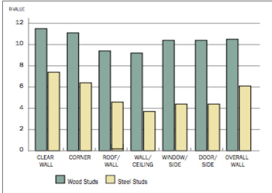
Figure 2. Thermal resistances of wall components with R-12 insulation.
