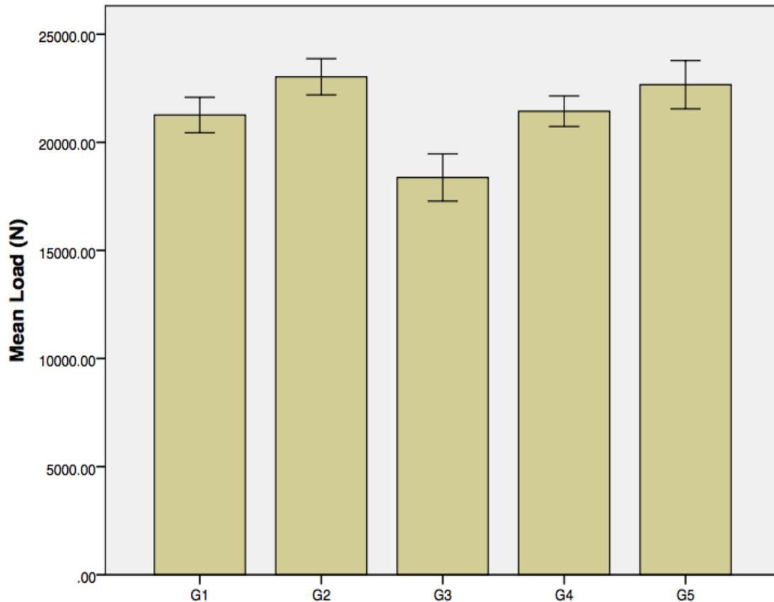
Figure 18. The average peak load (N) for each glulam bolt with error bars representing +/- one standard deviation.
