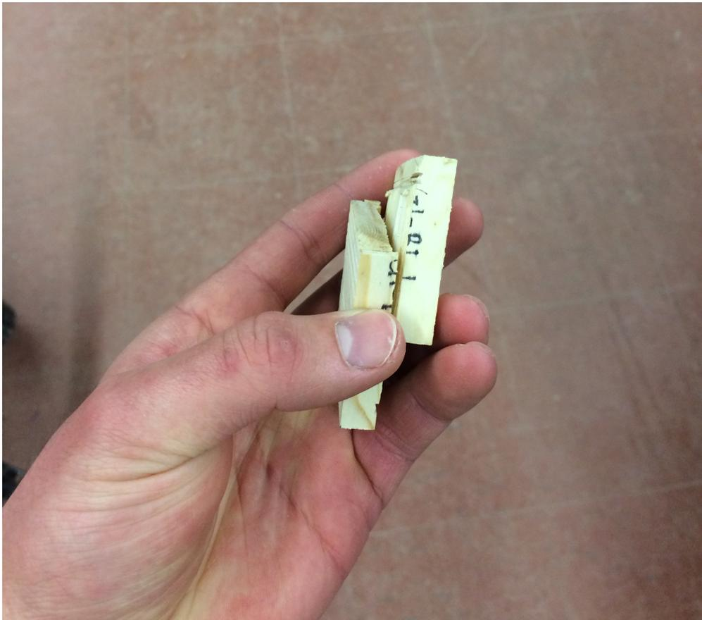
Figure 17. A replicate shorn on the glue line after the test was completed.
