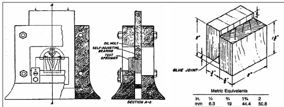
Figure 5. Shearing tool and ASTM standard dimensions for test replicates (ASTM 2008).
