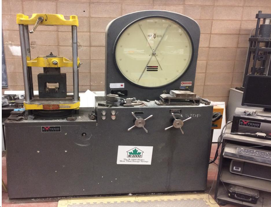
Figure 14. The Tinius Olsen testing machine and computer setup.
