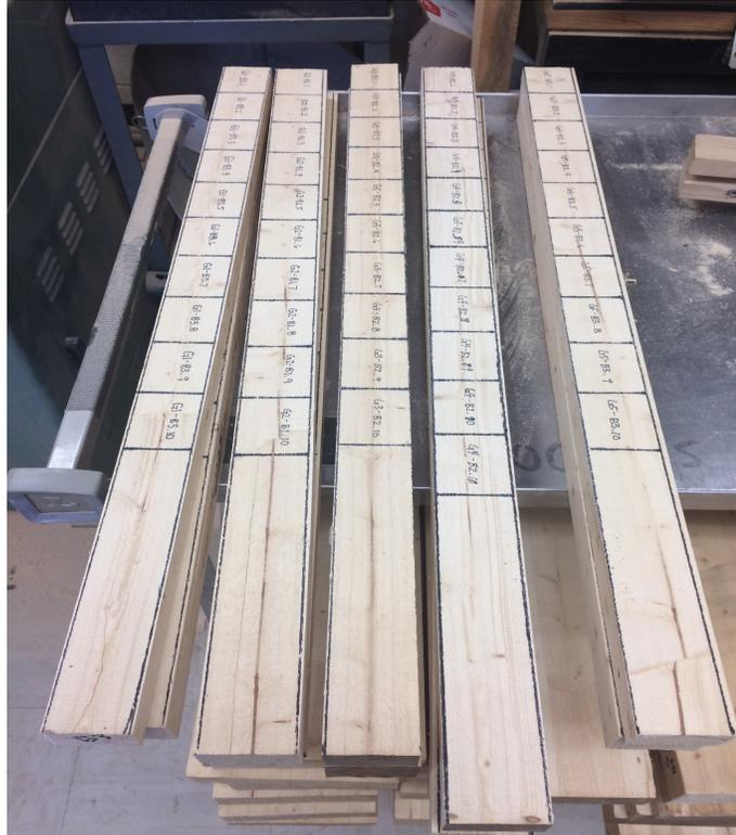
Figure 11. 2” sticks sawn using the table saw and ready to be sawn into replicates.
