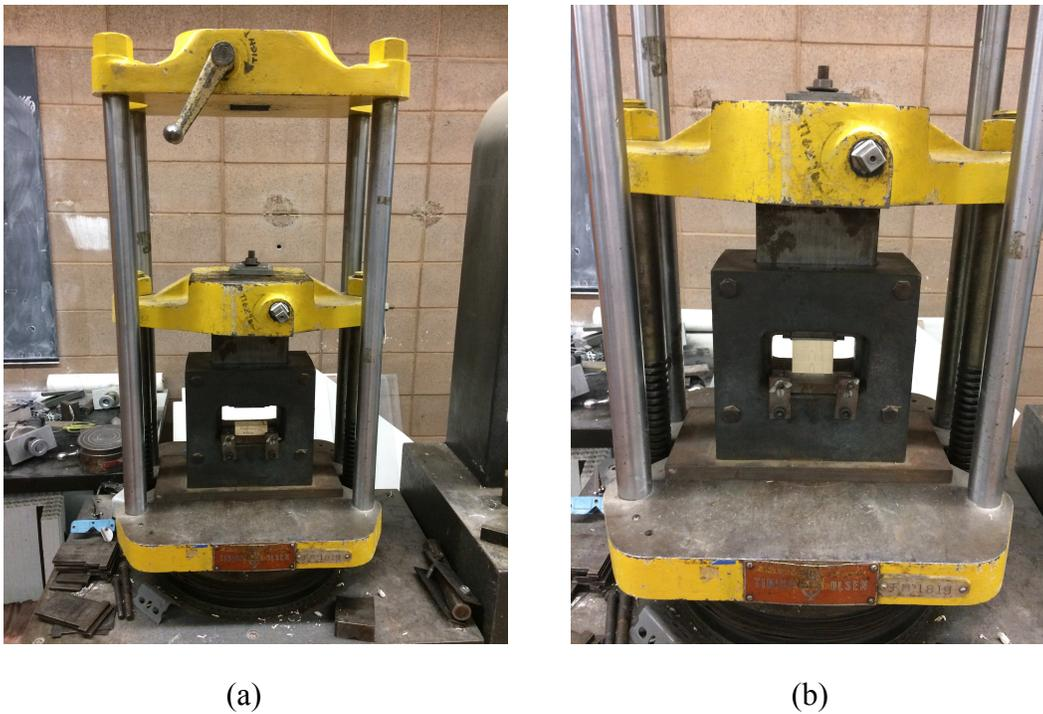
Figure 15. (a) The Tinius Olsen machine platform with the shear tool mounted on it, (b) the machine shearing a replicate.
