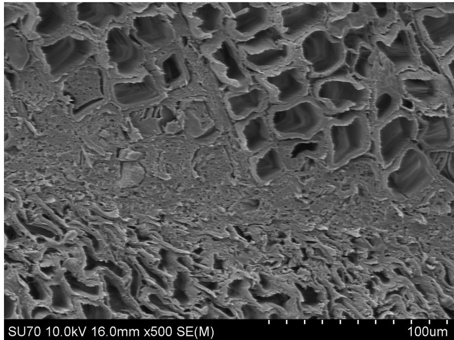
Figure 22. The glue penetrating the spaces between wood cells.
