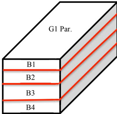
Figure 9. The parallel cuts at 3 7/8'', 2 5/8'' and 1 1/2'' for G1, G2...G5 samples.
